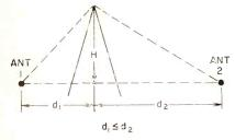
Fig. 2. Knife-edge refraction is caused by a high obstacle in the signal path. It occurs in much the same way that sound waves bend around a corner.
