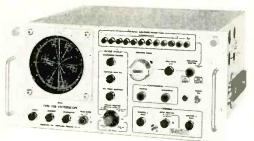
Measuring amplitude changes and phase shifts can be done accurately, conveniently, and independently with the Vectorscope.
