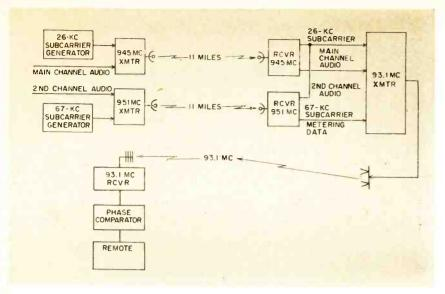
Fig. 3. At the KOSO(FM) transmitter site, the main carrier is modulated with main channel audio; the 26-kc subcarrier is modulated with second-channel audio; the 67-kc subcarrier is modulated with metering data for relay back to the studio via the station's radiated signal. A stereo receiver at the studio feeds frequency and modulation monitors and the metering data on the 67-kc subcarrier is fed into direct readout circuitry.
