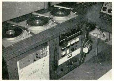
Turntables are mounted on left console wing where patch panel and audio terminal gear are located.
