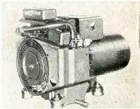
by the CCKB engine, offering a choice of gasoline or gaseous fuel carburetion. Rating of the horizontally-opposed 2-cylinder engine is 19.5 h.p. Generator offers optional reconnectible feature for delivering rated output in either 120- or 240-volt 2-wire service. Two models are available: remote starting and portable. Automatic load transfer is optional.
