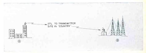
Fig. 1. AM and FM stations can eliminate leased studio-to-transmitter telephone lines with a microwave STL.
