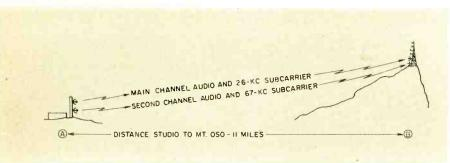
Fig. 2. KOSO(FM) STL employs two microwave transmitters at the studio to relay two stereo channels and two subcarriers to the remote transmitter location.
