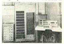
machine voltages, punched cards, digital clock, machine cues, and operator intervention. Said to be compatible with existing control equipment, the UNICON consists of two main frames, containing solid-state logic circuitry, power supplies and blowers, plus 5 display panels and a control and entry panel; panel units may be incorporated into master control console.
