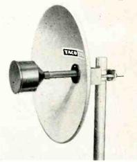
bronze to complement all architectural types. Antennas can be mounted on 2" to 4 1/2" diameter masts and rotated through 360° azimuth with 0 to 7° tilt. Installed from the rear of the reflector, the slot-dipole feed is "Cycolac" radome protected and may be positioned for horizontally or vertically polarized color and b & w signals.
