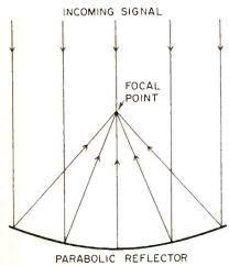
Fig. 4. A parabolic reflector concentrates the signal of a broad wavefront into a very small area.
