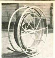
Heliax flexible waveguide for use in emergency restoration of 6-and 11-gc microwave systems available from Andrew Corp. Types EW56 and EW107 are being packaged on portable aluminum reels in various predetermined lengths with end fittings attached. In the event of failure, a transmission line section can be replaced quickly.
