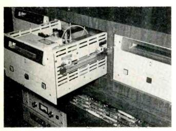
Slide-mounted cart machines provide easy access for cleaning and maintenance.
