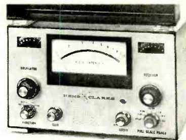
Nems-Clark FIM-135 uses taut-band meter movement to eliminate meter face-tapping.
