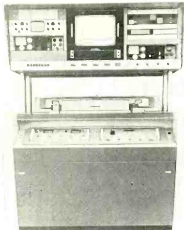
"Allenized" VTR is capable of all-band operation at the flip of a switch.
