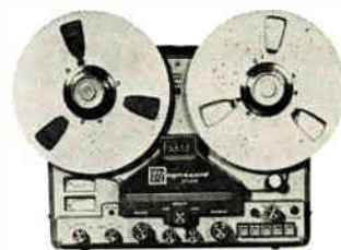
MAGNECORD MODEL 1048 Professional 2 channel (stereo) recorder/reproducer for use in main studio, production studio or conference recording. (10½" reel capacity) Model 1048 is available in ½- or ¼-track.
