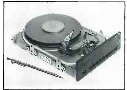
Today's disk drives provide high performance at a low cost. This 2-platter drive provides 20 Mbytes of storage.
