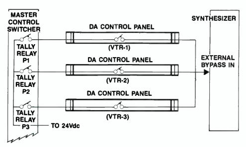
Figure 4. The stereo synthesizer is controlled from the switcher's tally signal routed through the appropriate VTR DA control panel.
