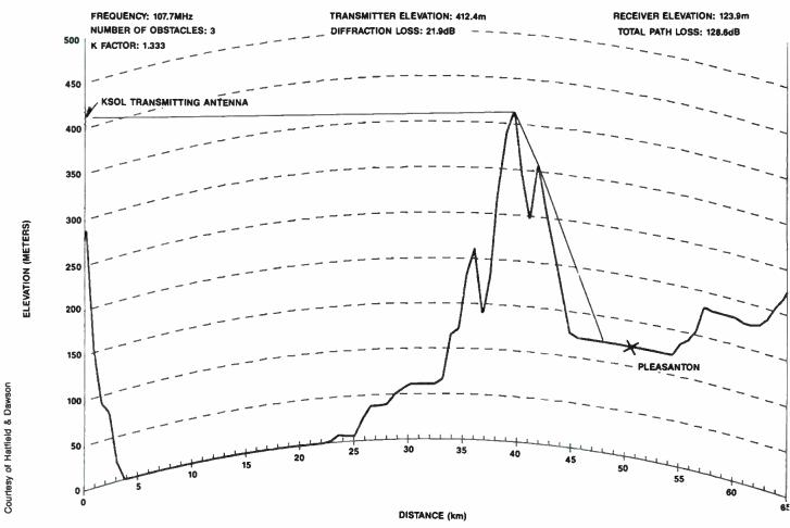
Figure 2. Elevation plot of the San Francisco Bay area showing the signal blockage suffered by KSOL-FM (and many other Bay area broadcasters). The mountain ridge effectively shields the community of Pleasanton from service, despite predicted Grade A coverage signal strength.
