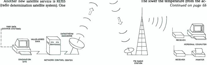
Figure 3. Data communications systems use broadcasters as "last mile" distribution system. The datastream from the network is transmitted on vacant FM subcarriers.
