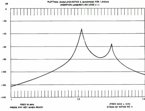
Figure 3. The graphic display illustrates the importance of plotting a filter's response. In this graph, C2 was changed to 4.7pF, which might have gone unnoticed without a frequency-response
