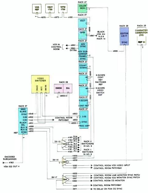
Figure 1. At the foundation of any new design or upgrade are the pulse and signal-flow diagrams. These diagrams should include cable and equipment location numbers to reduce confusion and help in equipment setup.
