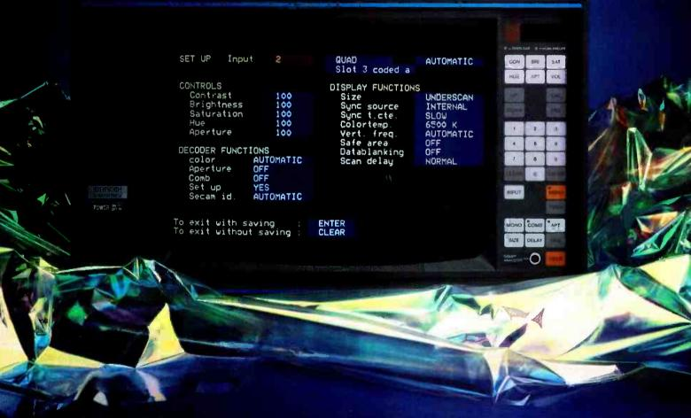
BARCO INDUSTRIES' new CVS professional broadcast monitor is microprocessor-based to make it intelligent in operation and easy to use.
