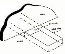
Cable trays that pass through walls or floors must be filled with a blocking material to prevent the transmission of sound.
