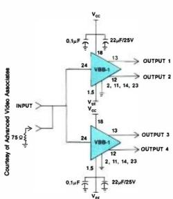
Figure 1. New integrated circuits permit up to 75MHz bandwidths on video DAs. This chip makes it possible to build a 1-in, 4-out video DA with only a handful of parts.
