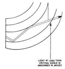
Figure 3. Light at less than the critical angle for reflection escapes the fiber and is absorbed into the jacket.
