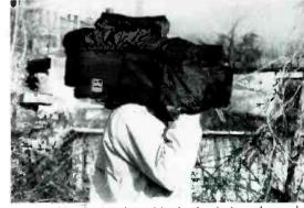
Newly developed instant rain-top shown in place. Note small pocket for storing
