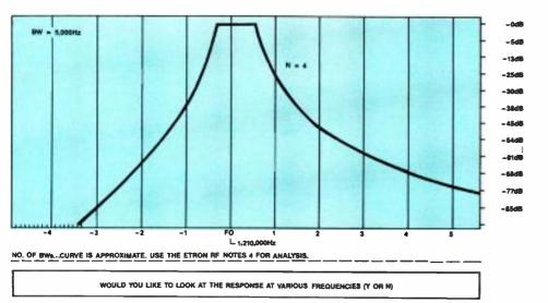
Figure 5. Insertion loss for circuit calculated in Figure 4.
