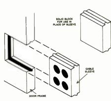
If camera cables or other movable cables must pass through a door, a removable sleeve may be used to help maintain isolation.
