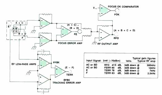
Figure 1. The RF signal is produced by the cross-connected photodiodes. The RF amplifier can be checked easily by "buzzing" the inputs.
