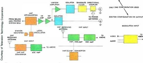
Figure 4. Block diagram of a typical UHF translator. Note that this design provides three possible inputs: VHF, UHF and discrete audio-video.
