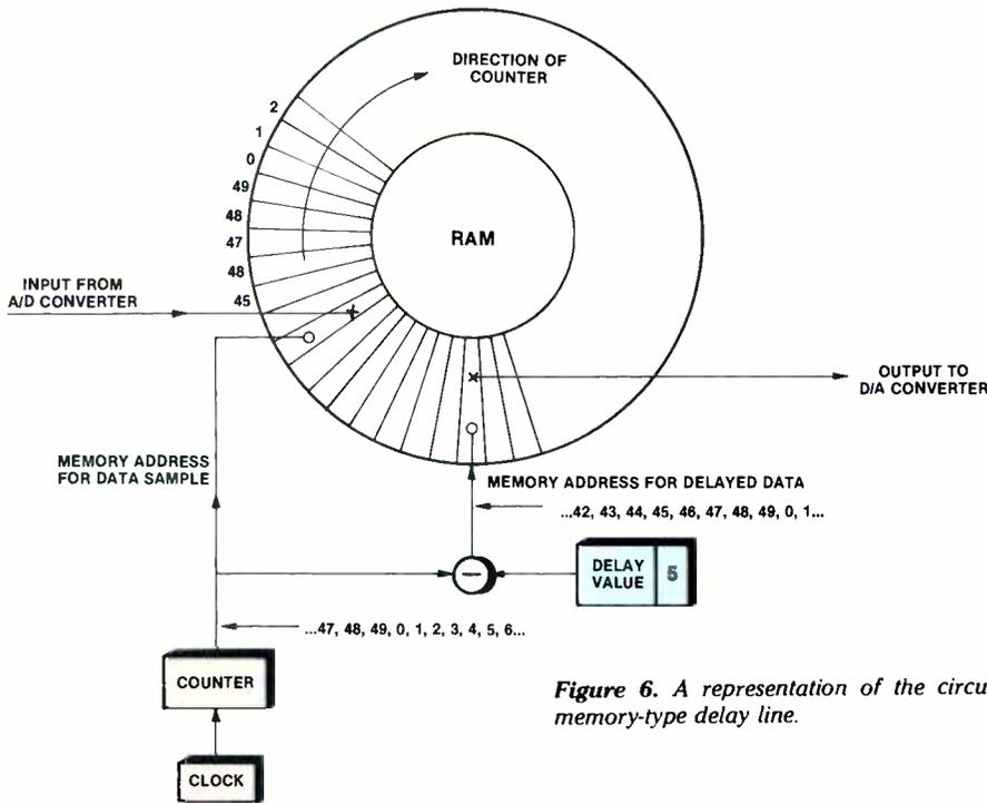
Figure 6. A representation of the circular memory-type delay line.
