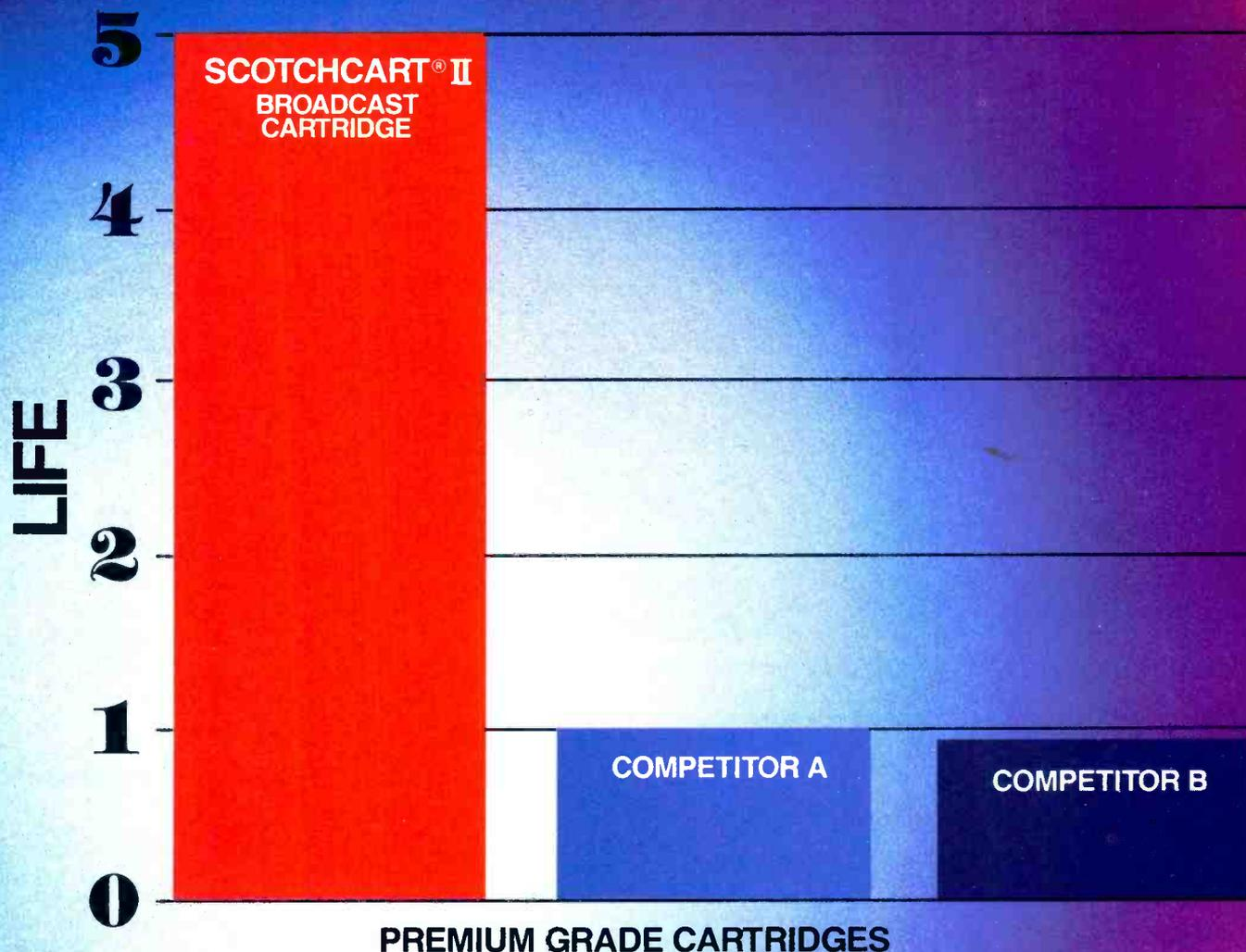
**R**esults are based upon tests using 3.5 minute length premium grade cartridges and ITC cartridge machines. A cartridge was considered at the end of useful life when it reached a 5 dB frequency response loss at 10 kHz, .5% DIN weighted flutter, or mechanical failure. These criteria represent easily recognizable problems that should result in the cartridge being removed from service.
