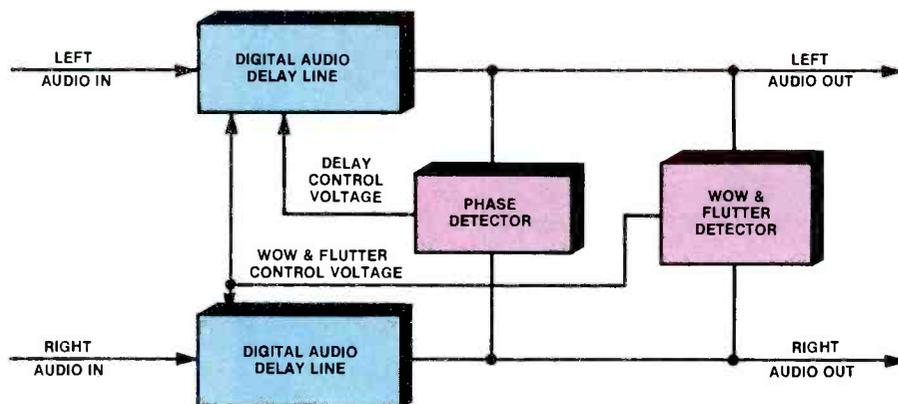
Figure 7. Simplified block diagram of a digital TBC.
