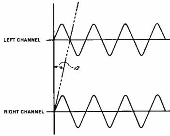
Figure 2. These signals represent the output from a stereo recorder. The interchannel delay of  $180^\circ$  represents a worst-case situation for any desired monaural signal.
