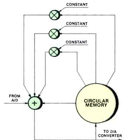
Figure 8. A simplified digital reverberation device block diagram.
