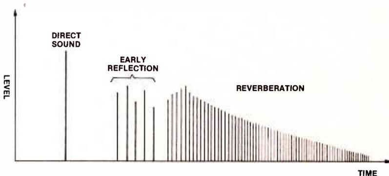
The echogram, shown here, displays the basic elements of a sound in a room as heard in a typical listening position. The direct sound out of the speaker is received a short time after it is presented because of the distance between the speaker and the listener. Sound travels approximately one foot per millisecond, making this delay tens to hundreds of milliseconds long.
