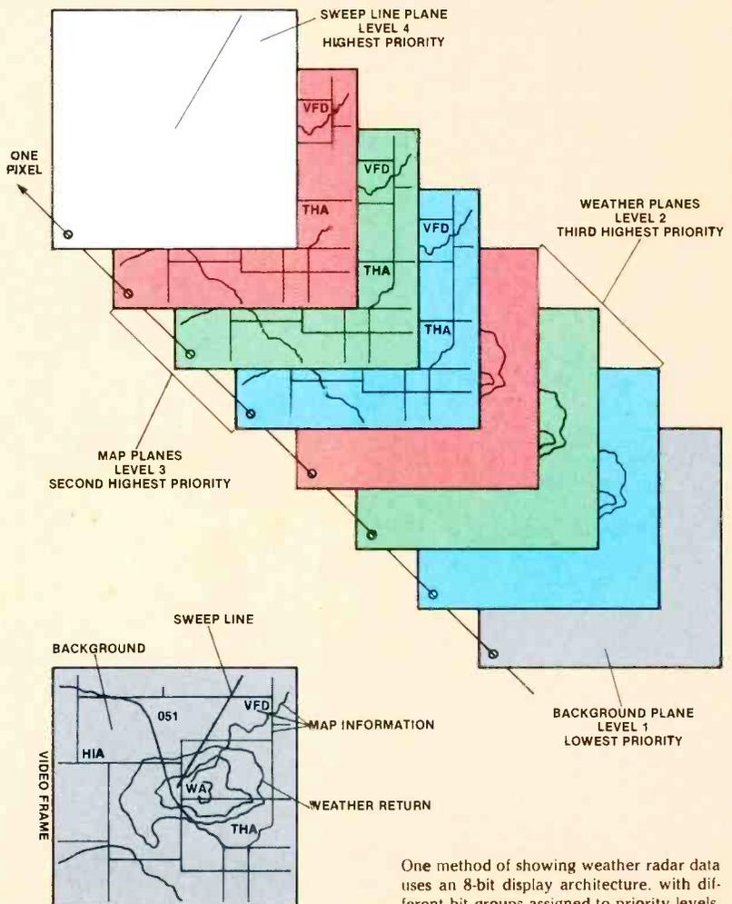
One method of showing weather radar data uses an 8-bit display architecture, with different bit groups assigned to priority levels.
