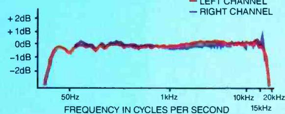
The new tape was conceived as an integral part of a complete cartridge system. When used with high quality equipment, such as an ITC "99B" cartridge machine, the ScotchCart® II broadcast cartridge is capable of frequency response equalling professional reel-to-reel performance.
