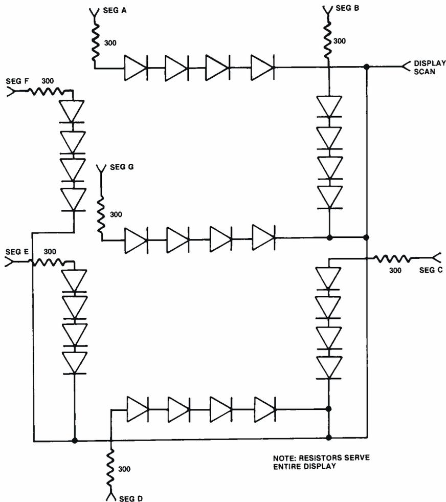
**Figure 2.** The large display consists of four LEDs connected in series. When supplied with a short-duration 24Vdc pulse, they provide an attractive display.
