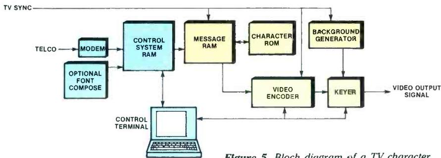
Figure 5. Block diagram of a TV character generator/titrer.
