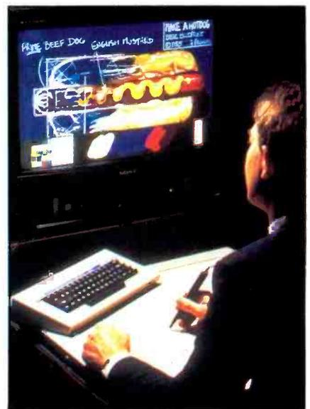
Drawing options on a graphics system may be indicated by a menu, at the lower left edge of the screen, and accessed from the drawing pad or keyboard. A color-mixing palette appears at the bottom of the screen.
