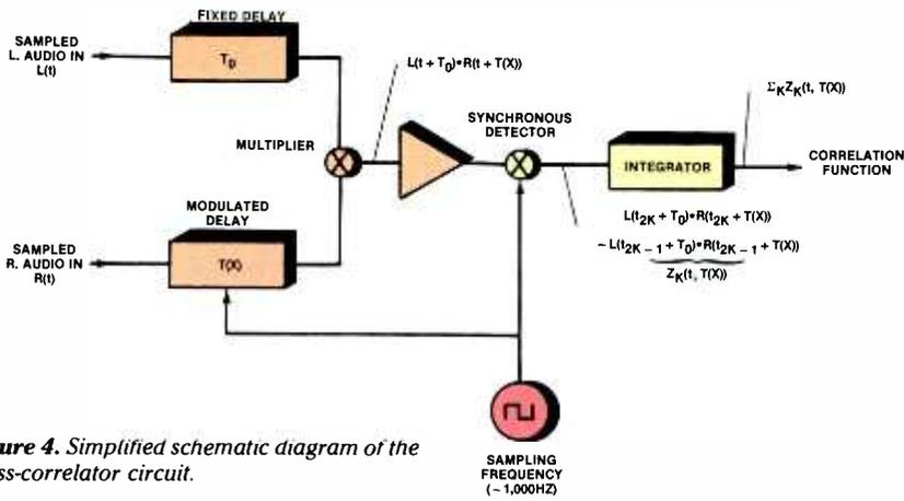
Figure 4. Simplified schematic diagram of the cross-correlator circuit.
