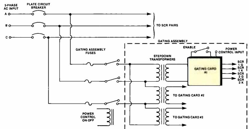
Figure 1. Block diagram of a 3-phase thyristor power control system.
