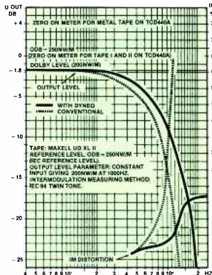
Figure 1. Notice how a constant input level causes lower output and high distortion at high frequencies.
