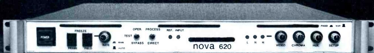
We brought our new nova 620 time base corrector to the SMPTE Show in Los Angeles to introduce its full frame of storage to freeze a field or frame of video for special effects applications.
