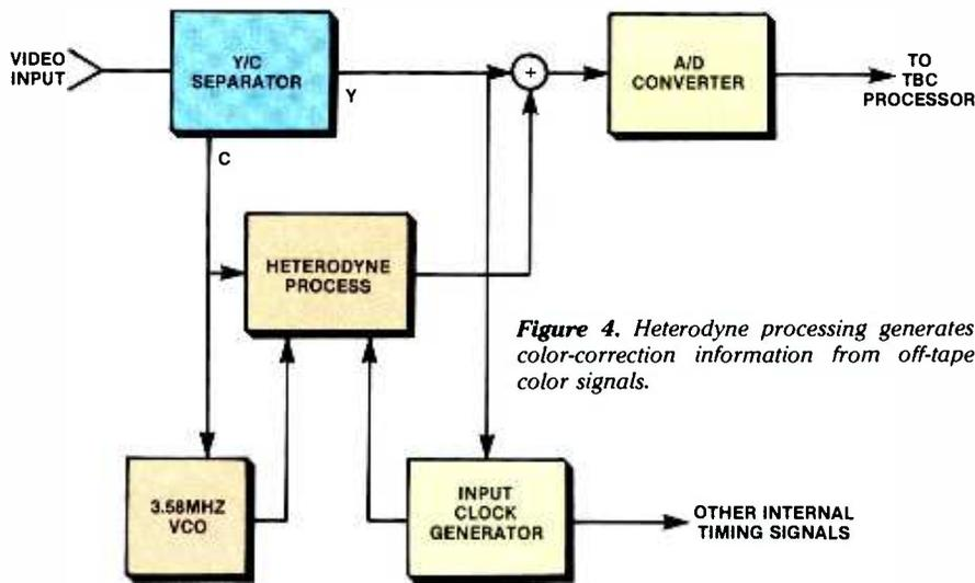
Figure 4. Heterodyne processing generates color-correction information from off-tape color signals.
