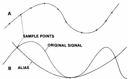
**Figure 1.** Two sampling rates showing the effect in the time domain. Curve A shows the effect of sampling more often than two times the input frequency. Curve B shows how an alias curve is generated when sampling less than two times the input frequency.
