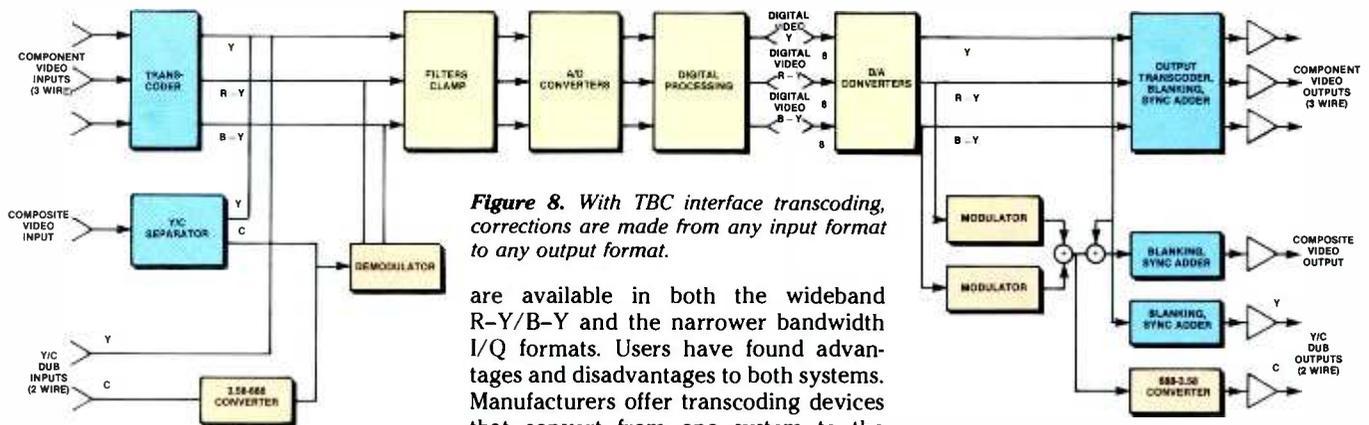
**Figure 8.** With TBC interface transcoding, corrections are made from any input format to any output format.
