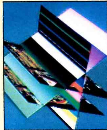
One live camera signal and two test patterns are combined through 3-D software. This uses object priority and perspective as a result of the viewing angle, but does not use horizon perspective.
