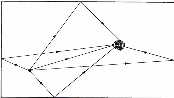
Two representations of reverberation signals. Above, the reflections from surfaces in a space. Below, a plotted representation of the signal content over a period of time.
