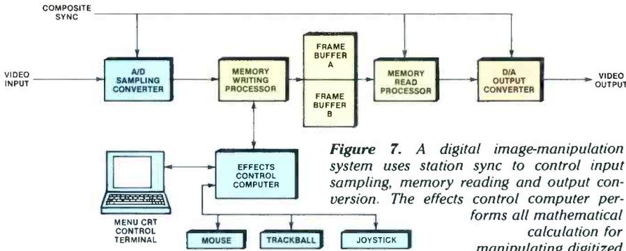
**Figure 7.** A digital image-manipulation system uses station sync to control input sampling, memory reading and output conversion. The effects control computer performs all mathematical calculation for manipulating digitized video according to algorithms called by control terminal.
