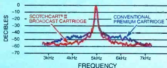
The Revolutionary ScotchCart® II broadcast cartridge design eliminates the excessive audio sideband noise which results from the rubbing effects of pressure pads and the mechanical irregularities of rotating hubs found in conventional cartridge designs.
