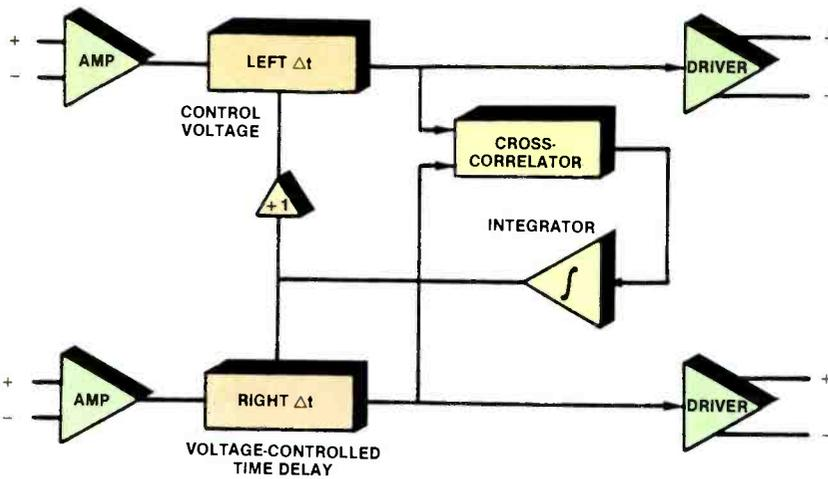
Figure 6. Block diagram of a functional cross-correlator TBC.
