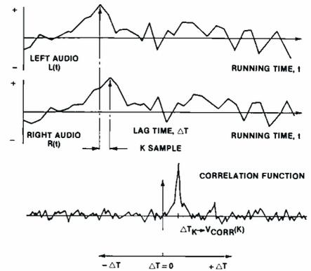
Figure 3. The upper graph represents the left and right signals to be analyzed. The lower graph represents the output voltage from the cross-correlator corresponding to delta T.
