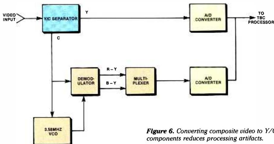
Figure 6. Converting composite video to Y/C components reduces processing artifacts.
