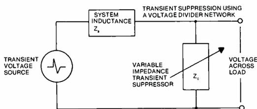
Figure 1. The mechanics of transient suppression using a voltage-clamping device.
