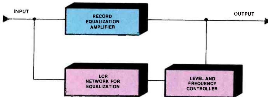
**Figure 3.** The Dyneq circuit dynamically adjusts the record equalization curve as the amount of high-frequency material varies. Tapes produced on this machine are usable on any other cassette recorder.
