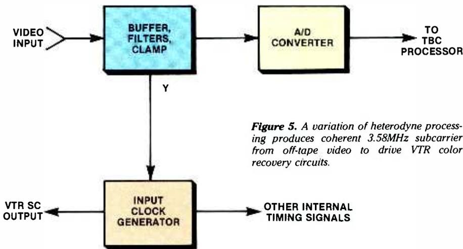
Figure 5. A variation of heterodyne processing produces coherent 3.58MHz subcarrier from off-tape video to drive VTR color recovery circuits.
