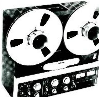
Universal reliable direct drive tape deck based on die-cast chassis; motion sensing and full logic control of all tape transport functions; two speeds; wide range available; for VU meters with peak indicators; professional headblock with 3-point mounting; electronics with high head room.
