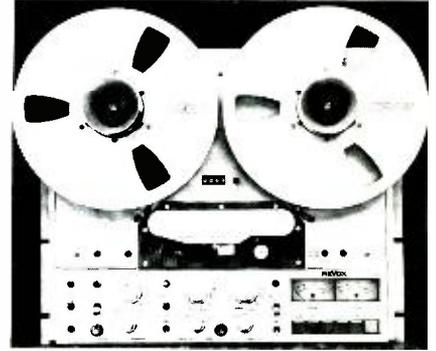
Professional broadcast recorder/re-producer. Three direct drive motors; servo-controlled capstan; tape dump feature; sel sync for both channels; optional balanced microphone input; full logic control with motion sensing; modular construction with die-cast chassis; 2-track or mono versions, portable, rack- or console-mount versions available.
