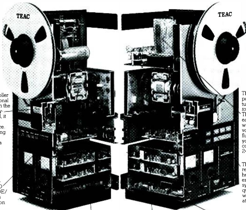
The impedance roller is strictly professional caliber. Along with the heavy dynamically-balanced flywheel, it guarantees better tape-head interface. Therefore, reducing the possibility of dropouts during a critical recording session.
