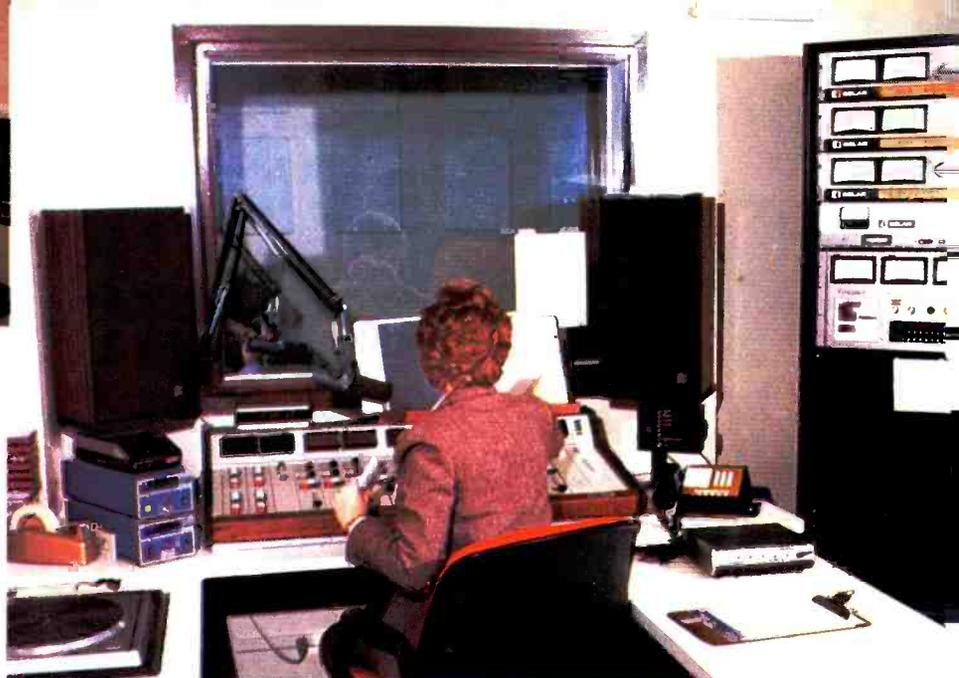
A view inside KBIA's main Studio A announce/control room, with staffer, Becky Preuss, at the controls. On the left are Technic SP-10 turntables and UMC Beaucart cartridge machines. The announcer faces and operates the Broadcast Audio System 16 audio console; Electro-Voice audio monitors flank the viewing window. On the right is an equipment rack housing the Belar monitors and Moseley transmitter remote controls.
