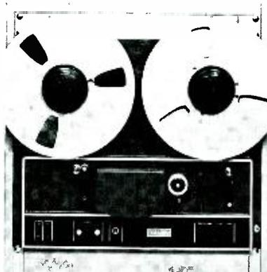
The 255 series of machines, developed for broadcasters, are compact 10.5-inch reel tape reproducers for mono or stereo automation or reproduce-only applications. This series has a heavy cast deckplate to maintain tape alignment, short head-to-capstan distance to reduce flutter, trouble-free TTL logic, optional 25 Hz tone sensor for automation and optional remote control.
