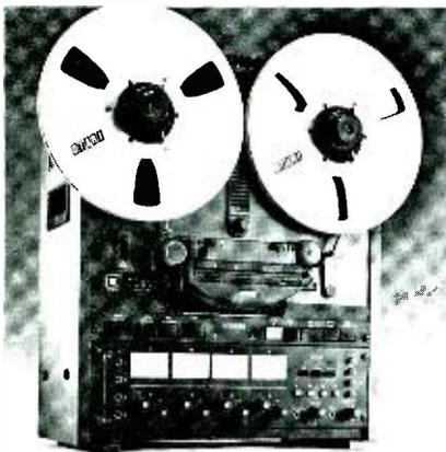
General features include compact 1/4-inch 4-channel machine with dual speed (15 7/8-1/2ips) variable speed dc capstan servo, selective reproduce, motion sensing control logic, built-in test and cue oscillator, plug-in heads and easily accessible electronics adjustments.
