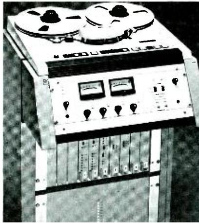
tive balancing on inputs and outputs; adjustable phase compensation, bias, record and playback levels that are aided by an internal multi-frequency square/sine wave generator; and rear-panel interface to transport and time base functions for SMPTE interlock.
