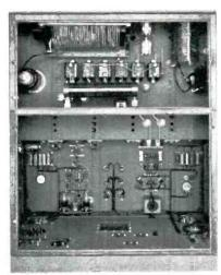
Vacuum variable tank condenser, output circuitry, and accessibility of components are shown.
