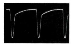
Figure 2 Waveform observed at plate of crystal oscillator V-I.
