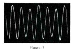
"Stair step" waveform seen at plate of first tripler (V-7) showing tripling action. This is 300 Kc. with a 100 Kc. component appearing as AM. This effect is removed by coils L-1 through L-6.
