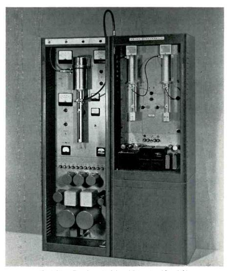
The UST-10 Translator (right) and RA-7 Amplifier (left) combined to form a 100-watt Translator-Transmitter.
