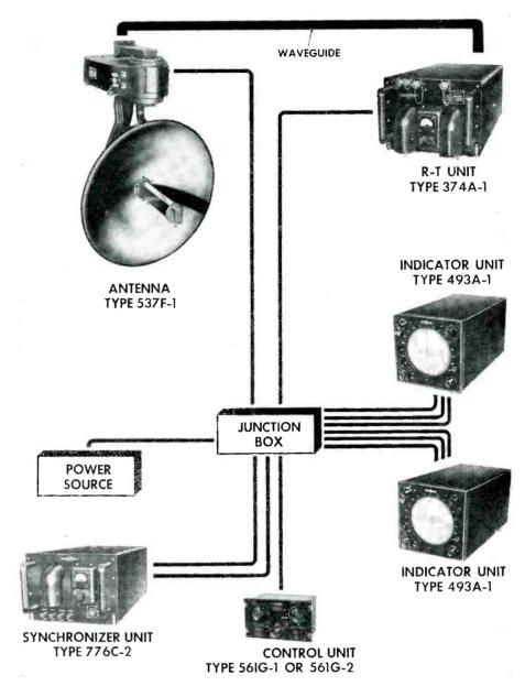
Figure | | Complete Weather Radar System.
