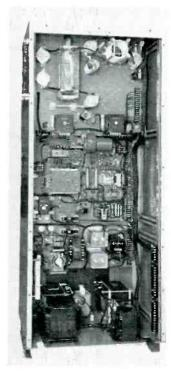
RCA BTA-1R Vertical construction provides accessibility.
