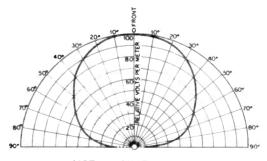
USTA-4 UHF Antenna Horizontal Radiation Pattern.
