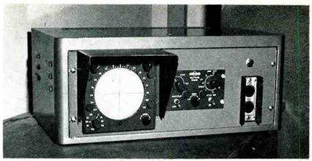
Figure 2 Radar Indicator and Control Unit.
