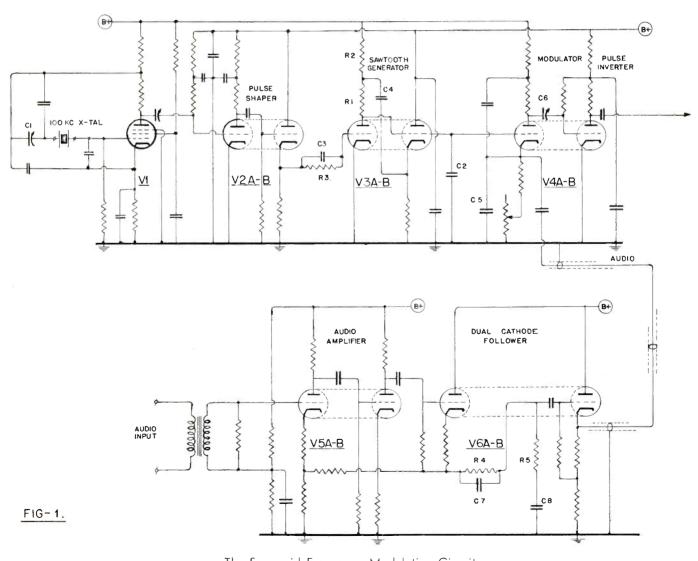
The Serrasoid Frequency Modulation Circuit
