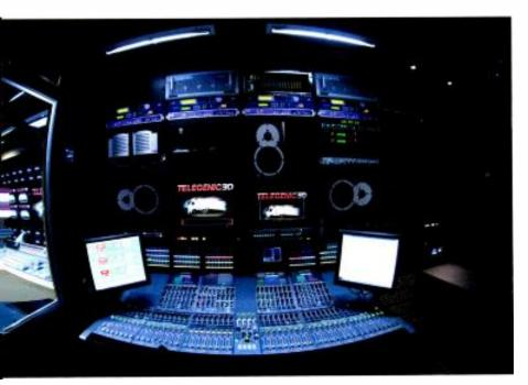
Shown here aboard a Telegenic OB truck, the Calrec Apollo console allows users the option to output LtRt phase-encoded signals directly from the console's main outputs. onsoles sit at the center of every recording and broadcast project — in the studio, in the field, routing and processing audio. But, although technology has developed significantly, the role of the console has remained fundamentally consistent for the last 75 years or so.
