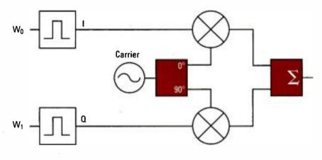
Figure 1. QAM modulator
