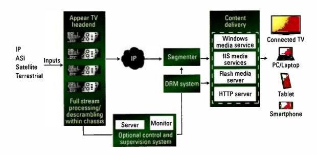
Figure 1. The Appear TV Multiscreen's open architecture allows it to receive signals through a variety of interfaces — including XML and SOAP — and deliver them to devices ranging from connected TVs to smartphones.
