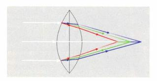
Figure 1. If chromatic abberation exists, meaning all three images do not converge in the same plane, adjustments could be made. But new modern lenses have fixed imagers, so the lens must provide precise focus.
