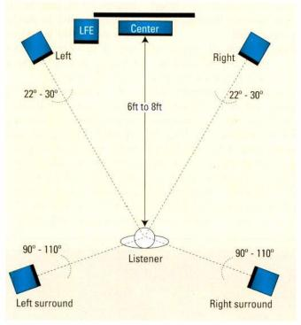
Figure 1. Shown here is the speaker placement for 5.1 audio.
