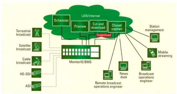
Figure 1. Digital Nirvana's MonitorlQ BMS integrates with other broadcast operations systems. Staff can access the BMS using any Web-enabled device from any location.
