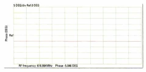
Figure 9. Final measured phase difference at midband Channel 38
