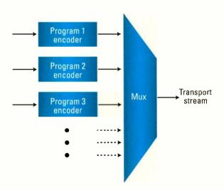
Figure 1. Transmission multiplexing involves the generation of transport streams. Within these streams, the various programs are compression encoded.
