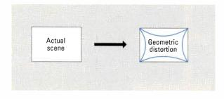
Figure 2. Geometric distortion occurs when a three-dimensional object is projected on a plane.
