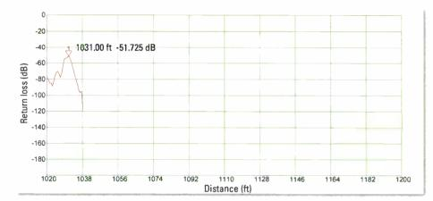
Figure 3. Initial measured time domain length difference for upper transmission line
