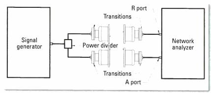
Figure 1. A basic through measurement configuration includes a signal generator, power divider, transitions from N female connectors to the correct transmission line size and impedance, and a network analyzer.
