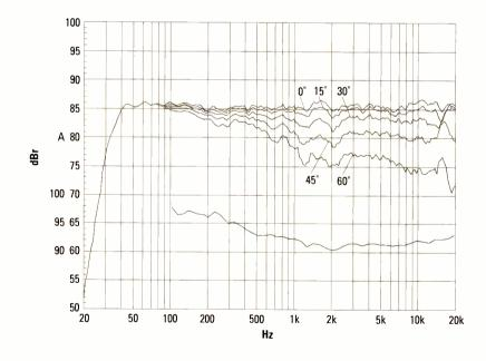
Figure 4. Illustrated here is the typical freestanding monitor frequency response featuring a directivity control waveguide and associated directivity curves (off-axis response); the lower curve is the power response of the system measured in an IEC-approved reverberant chamber.
