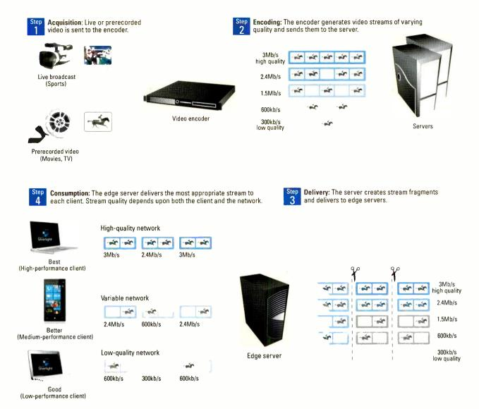
Figure 2. Microsoft IIS Smooth Streaming can adapt to changing network conditions by varying the quality of the stream.
