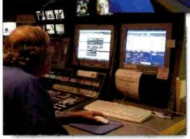
functions include: schedule import/export, editing and event monitoring with alarming and manual override; machine control for manual device control, server ingest and clip trimming; media database management; resource configuration; and a log viewer that can be filtered by any number of parameters. Up to 10 workstations can connect to an automation processor at the same time.
