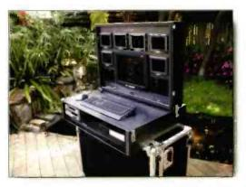
The Journeyman, a virtual studio in a box, has a 17" flat-panel LCD control monitor; eight individually assignable, 5.6" LCD monitors; and a control PC, keyboard and mouse.
