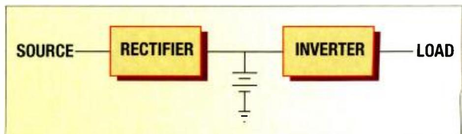
Figure 2. In an online configuration, incoming power is fed to the system's battery at all times, providing an effective low pass filter.
