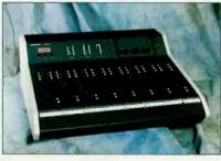
The eight-channel surface accepts up to 16 stereo inputs and has two stereo and one mono output. 24-bit internal processing. Inputs can be AES-3, SPDIF or analog. Flip-top front allows easy internal access. Graham-Patten Systems is the manufacturer of the internal electronics.
