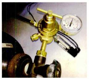
Figure 4: Omega tank pressure sensor
