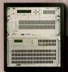
EM 2000 is a 2000W FM transmitter made up of the EM 25 DIG exciter (or EM 20/30 exciter) and the AM 2000 FM amplifier. AM 2000 Includes eight 300W high-efficiency MOSFET technology amplifying modules, fee by 2 independent switching power supplies, which are mode to withstand the working conditions. The amplifying modules work independently thanks to a power combining structure that provides high isolation between them.
