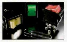
is diffused through a matching clear cap to guarantee even color distribution. These switches are uniquely designed to have current ratings of 9A@125Vac or 6A@250Vac in a compact body. The long mechanical life of 30,000 operations minimum is made possible by the quick-make, quick-break characteristic of the contact mechanism which limits arcing. This single-break, snap-acting contact mechanism provides smooth actuation and audible feedback to operators.
