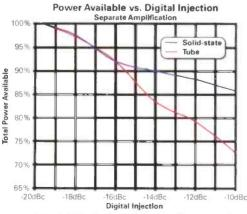
Figure 2. Transmitter derating for separate amplification.
