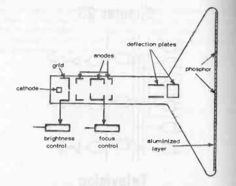
Fig. 23-1. The TV tube and its basic controls, shown in simplified form.
