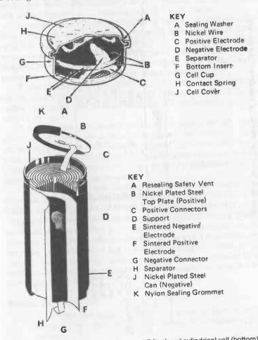
Fig. 25-5. Typical nickel-cadmium button cell (top) and cylindrical cell (bottom).
