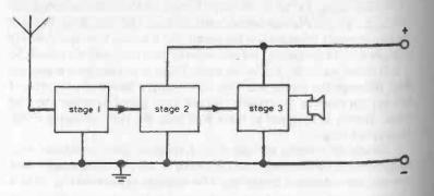
Fig. 19-2. Stages shown with "common ground" and power supply connections.
