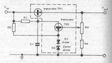
Fig. 14-2. Voltage-regulator circuit using CA3097E array.
