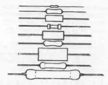
Fig. 4-2. Examples of modern resistor outlines (actual size).
