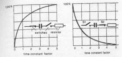
Fig. 6-2. Closing switch 1 allows capacitor to charge right up in a time equal to 5 time constants. It then takes a similar period to discharge fully through a load resistor when switch 2 is closed.
