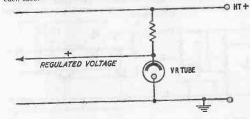
Fig. 27-5. Voltage stabilization with VR tube.
