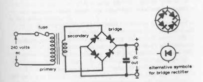
Fig. 8-5. Practical power-supply circuit. A high value capacitor is used. The four diodes are bought as a single component called a bridge rectifier.
