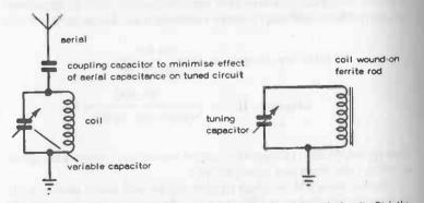
Fig. 22-1. A variable capacitor and coil form the usual tuned circuit. Strictly speaking this tunes the aerial, if an external aerial wire is used. Most AM receivers use a ferrite rod aerial which does not require an external aerial.
