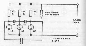
Fig. 10-6. Sequential flasher using NE-2 miniature neon lamps (or equivalent).
