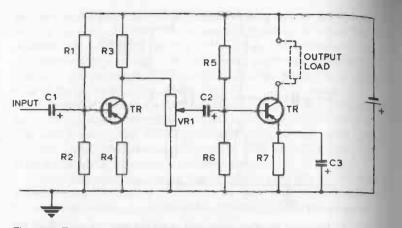
Fig. 17-7. Two-stage amplifier with volume control.
