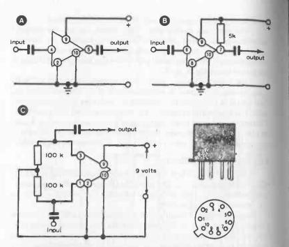
Fig. 13-2. Three amplifiers based on the CA 3035 IC, all giving a gain of about 100. All externals capacitors are 10 µF.
