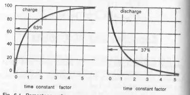
Fig. 6-1. Percentage voltage across capacitor related to time when being charged (left) and discharged (right).
