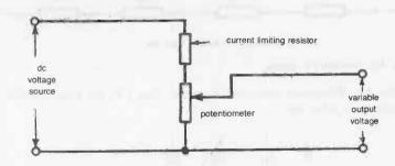
Fig. 4-4. A practical adjustable potential divider.
