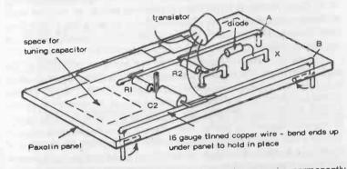
Fig. 20-4. Lay down the top and bottom lines in tinned copper wire, permanently mounted on the panel. Shorter lengths of bare wire can be used for other common connecting points. Complete by soldering component leads in place.
