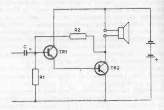
Fig. 17-4. Amplifier for loudspeaker output. Components:
