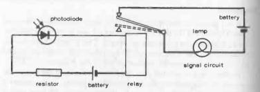
Fig. 11-6. Photodiode used as a "light" switch. The rise in current when the diode is illuminated makes the relay pull in completing an external circuit through the relay contacts.
