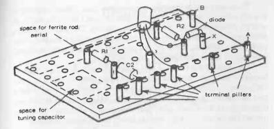
Fig. 20-6. Pegboard assembly is similar to Fig. 20-5 except that the board is predrilled to accept terminal posts. Locate these posts at suitable points to act as common connecting points. Connect components to posts, then complete the additional wiring as necessary. Note: all these constructional drawings show the same circuit—a simple single-transistor radio receiver with preamplifier. Components required are:
