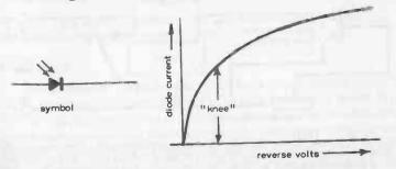
Fig. 11-5. Symbol (left); and characteristic performance of a photodiode
