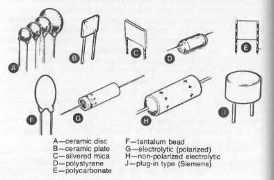
Fig. 5-2. Examples of modern capacitors.
