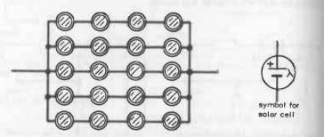
Fig. 11-10. Connections for a 2-volt solar battery to give a current of 15 milliamps through a 100 ohm load.
