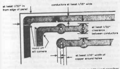
Fig. 21-3. Basic recommendations for planning conductor widths and spacings on PC boards.
