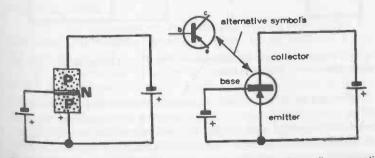
Fig. 9-4. Bias and supply connections to a PNP transistor shown diagrammatically (left) and in symbol form (right). bottom N section will promote a flow of current through the transistor bottom-to-top.
