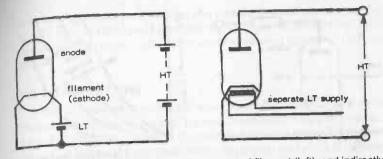
Fig. 12-1. Diode vacuum tubes with directly heated filament (left); and indirectly heated filament (right).
