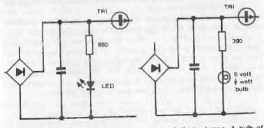
Fig. 26-3. Alternative arrangements for charging indicator lamps. A bulb of appropriate voltage could be used in one of the output leads without a dropping resistor.
