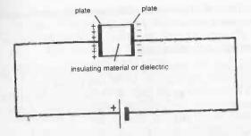
Fig. 5-1. Illustrating how a capacitor builds up a charge when connected to a dc voltage, blocking current flow.
