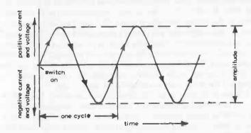
Fig. 2-3. Alternating current flow is in "cycles" of positive and negative current.
