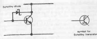
Fig. 11-4. Typical circuit for a Schottky diode (left) and the equivalent single component, a Schottky transistor (right).
