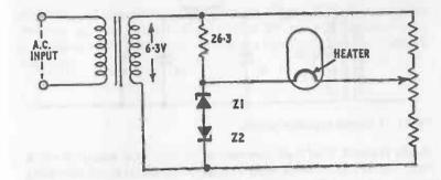
Fig. 27-12. Stabilized heater supply.
