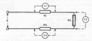
Fig. 3-3. Resistors drop voltage in a dc circuit.
