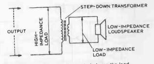
Fig. 17-11. Using an output transformer to balance the load.
