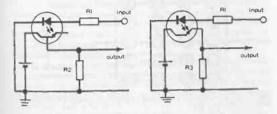
Fig. 11-9. Opto-isolator (combined LED and phototransistor), working as a photodiode (left); and phototransistor (right).
