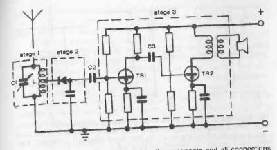
Fig. 19-3. The same stages drawn with all components and all connections required.
