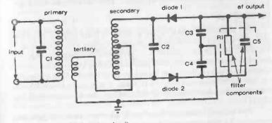
Fig. 22-5. Basic FM detector circuit.
