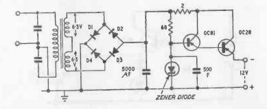
Fig. 27-13. Transistor power supply
