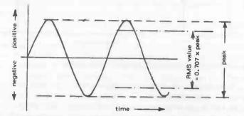
Fig. 2-4. Peak and Root Mean Square (rms) values of amplitude defined and compared.
