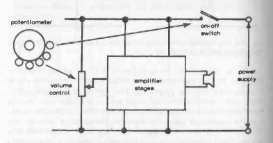
Fig. 19-6. In this example, a single component (the potentiometer connections) appears in two separate parts of the circuit diagram.
