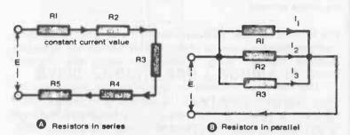
Fig. 3-2. Current has the same value through all resistors connected in series; but is different through each resistor connected in parallel.
