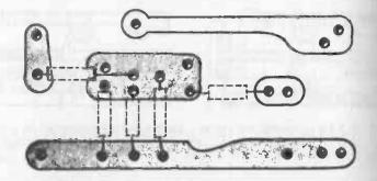
Fig. 21-4. Quite large areas of copper can be left on low voltage battery powered circuits. There is no need for consistent widths (or shapes) of conductors.
