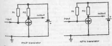
Fig. 9-8. Simple current bias circuits for transistor working.
