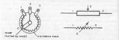
Fig. 4-3. Potentiometer shown in schematic form (left). Corresponding terminal positions are shown on the symbols (right).
