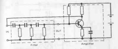
Fig. 18-9. Phase-shift oscillator based on filter circuit.
