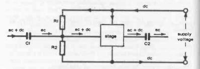
Fig. 3-8. Diagrammatic representation of flow of ac and dc in a circuit.
