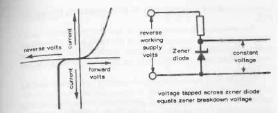
Fig. 11-1. A Zener diode, working with reverse bias, breaks down at a specific reverse voltage. Connected as shown, it can be used as a source of constant voltage supply. Note the symbol for a Zener diode.
