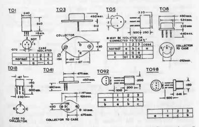
Fig. 9-10. Some common transistor outlines (diagrams by Electrovalue, all dimensions in inches).
