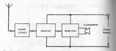
Fig. 19-1. Basic stages in a simple radio receiver.
