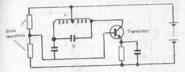
Fig. 18-5. Practical Hartley-oscillator circuit.
