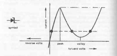
Fig. 11-3. Symbols (left) and characteristic performance of a tunnel diode. From "peak" to "valley" it exhibits negative resistance.
