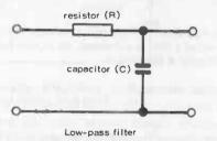
Fig. 6-9. Simple scratch filter circuit. Any combination of component values giving a product of RC = 1600 will work.
