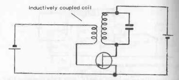
Fig. 18-3. Self-oscillating oscillator circuit.
