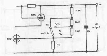
Fig. 26-2. Switching circuit for altering dc output voltage. R4A — 39 ohms R4B — 150 ohms R4C — 150 ohms
