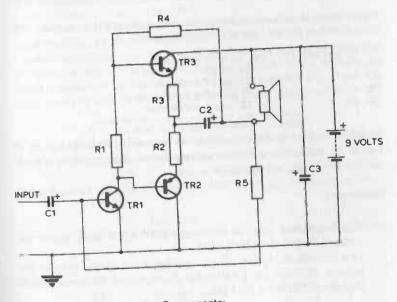
Fig. 17-9. Push-pull amplifier. Components:
