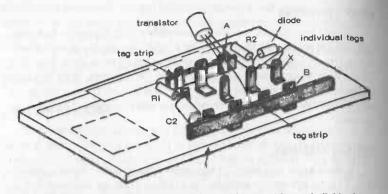
Fig. 20-5. All the connecting points are formed by tag strips or individual tags mounted on the panel. Solder components to appropriate tags, and complete with additional wiring as necessary.
