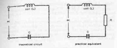
Fig. 7-3. Components which make a resonant circuit.
