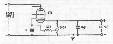
Fig. 27-11, Variable voltage supply.
