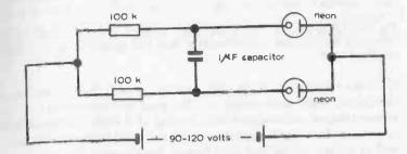
Fig. 10-7. Astable multivibrator circuit, each neon flashing in turn.
