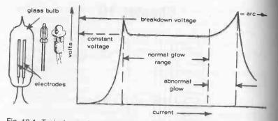
Fig. 10-1. Typical neon lamp construction and characteristic performance. A neon lamp only works in a dc circuit.
