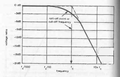
Fig. 6-8. The actual "roll-off" point on the frequency response curve of a filter is not sharply defined. The cut-off frequency is really a nomina figure and generally taken as the frequency at which there is a 3 decibel loss or a volts in / volts out ratio of 0.707. This is equivalent to a 50 percent loss of power.
