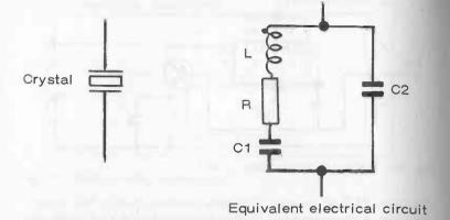
Fig. 18-7. Electrical circuit equivalent of a crystal.
