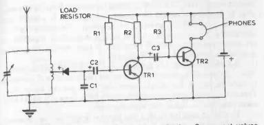
Fig. 17-3. Crystal set with two stages of amplification. Component values matching OC71, OC72 or near equivalent for TR1 and TR2:
