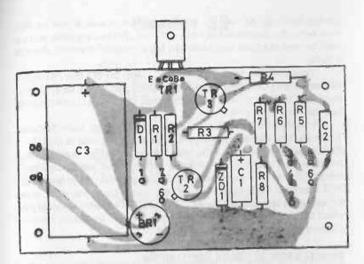
Fig. 21-5. Example of a printed circuit design with copper area shown shaded and position of components indicated.
