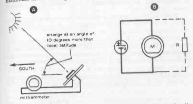
Fig. 11-11. Aligning a photocell to measure solar energy (left). The circuit on the right is a complete solar energy meter, the meter used being a 0-50 milliamp type.
