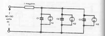
Fig. 6-4. Random "cascade" flasher circuit. Any number of lamps can be connected in this way and will flash in random order.
