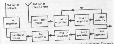
Fig. 22-10. Basic design of an AM/FM receiver shown in block form. The only common circuit is an af amplifier (usually a Class B output) following the detectors.
