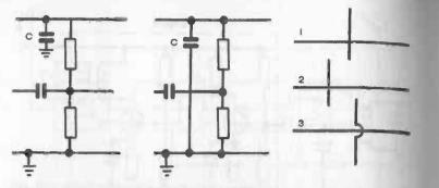
Fig. 19-5. The capacitor (C) is connected between top and bottom lines, but may be shown in a circuit diagram in either of these two ways. On the right are three ways of drawing crossing lines with no connection. Method 1 is the usual way. Method 2 is clearer; and method 3 clearer still.
