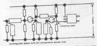
Fig. 19-7. Typical component layout drawing or working plan. This is the same circuit as Fig. 19-3, following the tuned circuit (which would be a ferrite rod aerial).
