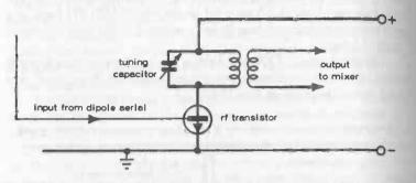
Fig. 22-3. Basic rf amplifier (or preamplifier) circuit as used in most FM receivers.
