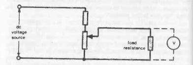
Fig. 4-5. The potentiometer can be adjusted to give required voltage across the load.
