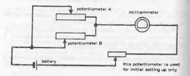
Fig. 13-4. Elementary analog computer based on two potentiometers.
