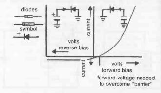
Fig. 9-7. Working characteristics of a typical semiconductor diode.
