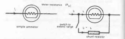
Fig. 3-5. Extending the range of a milliammeter.
