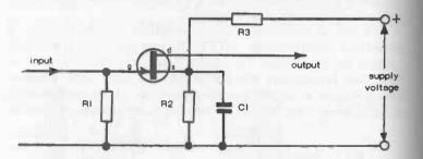
Fig. 9-13. Basic FET amplifier circuit. Performance is generally superior to that of a bipolar transistor amplifier.
