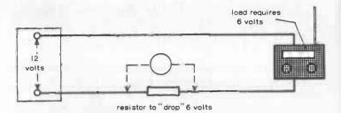
Fig. 3-4. Practical application of a dropping resistor.
