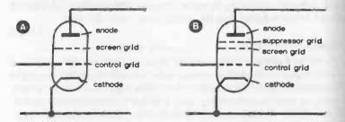
Fig. 12-4. Tetrode (left) and pentode (right) tubes, shown in simple diagrammatic form.
