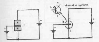
Fig. 9-6. Bias and supply connections to an NPN transistor, shown diagrammatically (left) and in symbolic form (right).
