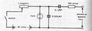
Fig. 10-5. Simple tone generator based on an NE-2 miniature neon lamp.
