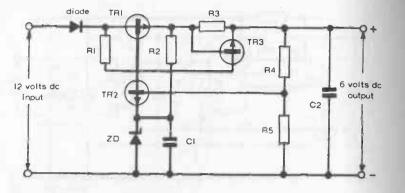
Fig. 26-4. Stabilized 6 volt dc charger working off 12 volt battery. Components: R1 - 680 ohms
