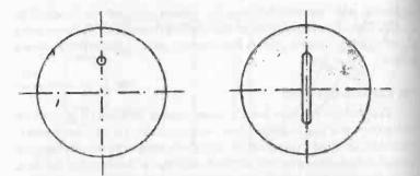
Fig. 12-6. Simple display of dc voltage (left) and ac voltage (right) on a cathoderay tube. The vertical displacement is a measure of the value of the voltage concerned.
