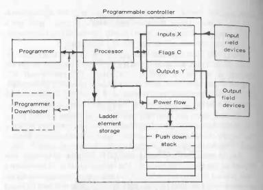
Fig. 24-1: Block diagram of Texas 510 Programmable Controller.
