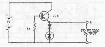
Fig. 27-15. Simple low-loss stabilizing circuit.
