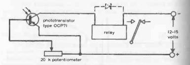
Fig. 11-7. Practical "light switch" circuit using a phototransistor. The relay should be of sensitive type and adjusted to pull in at about 2 milliamps. The potentiometer is a sensitivity control. A diode connected across the relay will improve the working of this circuit.
