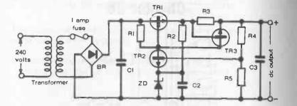
Fig. 26-1. Stabilized output dc charger for working off ac mains. Components:
