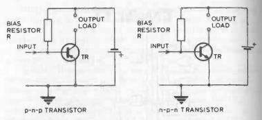
Fig. 17-1. Basic amplifier circuit.
