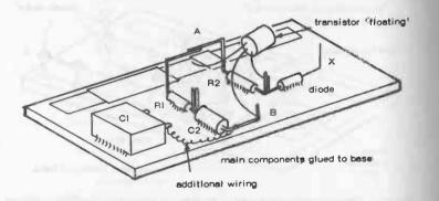
Fig. 20-3. Bonded mounting is similar to Fig. 20-2 but all components (except transistors) are glued down to a base panel. Turn up ends of leads to form connecting points.
