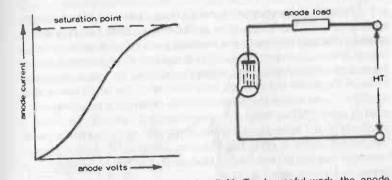
Fig. 12-2. Typical diode characteristics (left). To do useful work, the anode current must flow through a load resistor.
