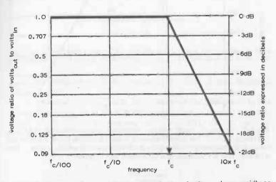
Fig. 6-7. Simplified diagram of how the ratio of volts  $_{\rm in}$  / volts  $_{\rm out}$  drops rapidly as the cut-off frequency of a filter is exceeded. All signals below the cut-off frequency are passed without attenuation.
