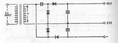
Fig. 27-10. Voltage-multiplier circuit using diodes.
