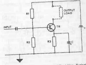
Fig. 17-5. Transistor amplifier stage with stabilized bias. Typical values for low/medium-power transistors:
