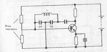
Fig. 18-6. Practical Colpitts-oscillator circuit.
