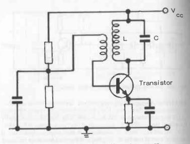
Fig. 18-11. Basic resonant circuit oscillator with transistor amplifier.
