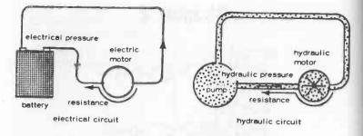
Fig. 2-1. An electrical circuit is similar to a hydraulic circuit.
