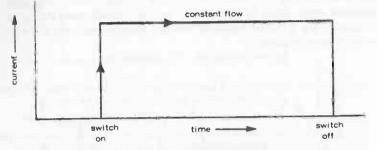
Fig. 2-2. Direct current flow with constant circuit resistance.
