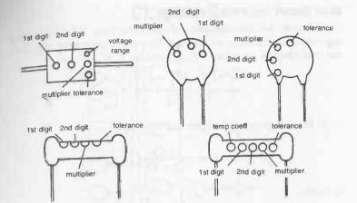
Fig. 5-5. Other coding systems used on capacitors,
