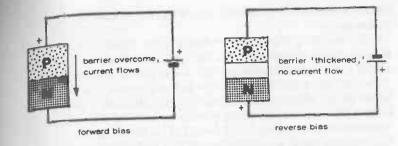
Fig. 9-2. The two modes in which a diode can be worked.
