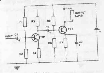
Fig. 17-6. Two-stage amplifier circuit.
