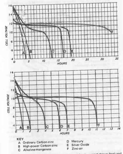
Fig. 25-3. Performance of AA size cells under moderate current drawn (top) and higher current drawn (bottom).
