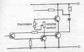
Fig. 11-13. Practical circuit incorporating a thermistor to counteract fluctuations in value of other resistors in the circuit due to heating effects or temperature changes.
