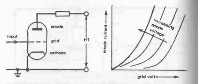
Fig. 12-3. A triode is a three-element tube. Anode current is controlled by the grid "bias" voltage.
