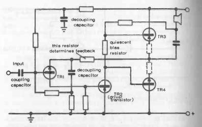
Fig. 22-8. Basic Class B output circuit. TRI works as a preamplifier. TR2 is the driver. TR3 and TR4 are a complementary pair of transistors, working alternatively in "push-pull." The two resistors shown by dashed lines may be added to improve the stability of the circuit. These only need to be of very low value (e.g., 1 ohm).
