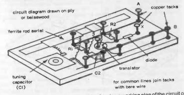
Fig. 20-1. Pinboard construction starts by drawing a working plan of the circuit on a panel of ply or balsa. Then drive in copper tacks at each connection point. Solder component leads to tacks, and complete circuit as necessary with any additional wiring.
