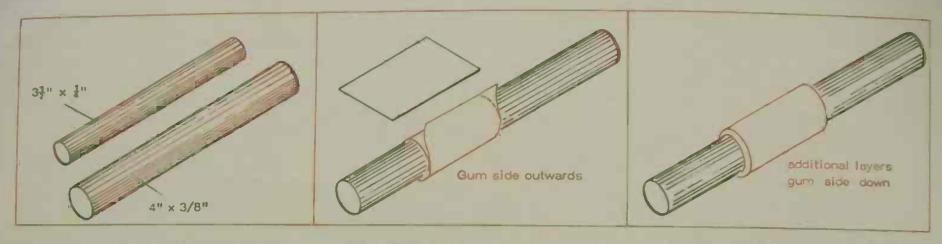
1. Two standard diameter sizes of Ferrite rod are shown. You can use either for making a *lerrite rod aerial*. Cut to length with a hacksaw, or mark with a sharp file and break off. 2. Cut several lengths of gumstrip (gummed paper) about 35 mm (1<sup>1</sup>/<sub>2</sub>") long. Moisten one strip and wind round the rod, gum side outwards to make a neat wrapping.
