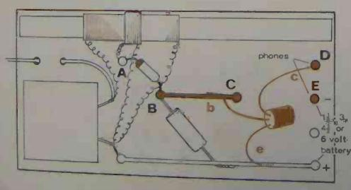
This circuit is a basic crystal set (with diode), with the addition of a transistor to work as an *amplifier* to boost the strength of the signal received (photograph, far right). This time all three leads to the transistor are connected and a battery is needed to power the transistor.
