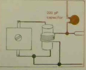
Back to the same trick of connecting the aerial into the diode side of the circuit. Here it has no direct connection at all to the main aerial coll—but it often works well.
