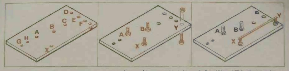
4. Use a 3 mm drill to drill holes A, B, C, D, E and F. Use the same drill to drill holes X and Y. Then change to a  $\frac{1}{16}$  drill to drill holes G and H.
