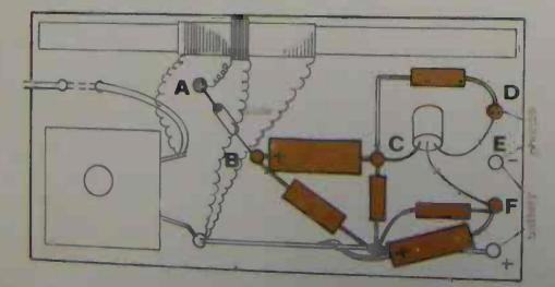
This circuit is the same as that on page 18, with *capacity coupling* between terminals B and C and the addition of several more components in the *transistor amplifier* stage; intended to 'fix' and stabilise the working point of the transistor. This should give more consistent results.
