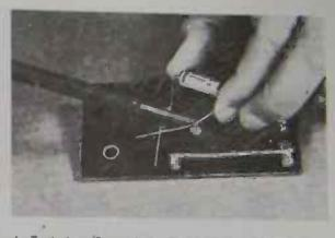
4. Technique for soldering 'bus bar' and component leads in place. Hold iron in place to heat up joint, then touch with solder, which should-melt and run freely to complete joint.
