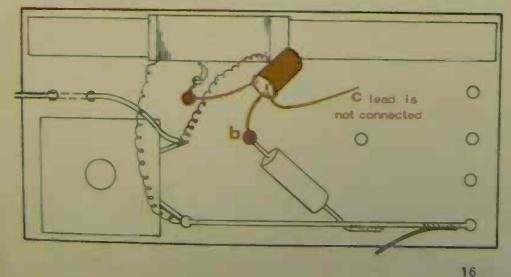
A transistor can work like a diode, using just two of its connections—the (e) or emitter and (b) or base leads. The diagram opposite shows the complete circuit—the same as on pages 1.2/13 with a transistor used instead of a diode. The unused (c) lead of the transistor is twisted out of the way.
