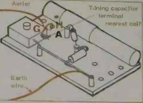
4. The diode is connected next. Cut the leads to about 25 mm (1") long. Solder one lead to terminal A and the other lead to terminal B. It does not matter which way round the red end is.
