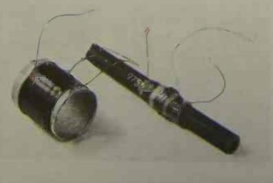
Air-cored coils are not as efficient as ferrite rod aerials, but they are cheaper to make. You can wind these coils on card tube formers—or even a length of hardwood or balsa dowel. Coil diameter should be 25 mm (1")—not smaller. You can use a larger coil former (in which case reduce the number of turns), but this produces a more cumbersome coil. The size shown in the illustrations matches a 500 pF tuning capacitor.
