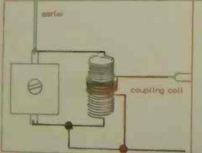
This type of senial coil, with an overwound coupling coil, will often work better than a single coil with a tapping point. Adjust coupling coil position up or down for best results.
