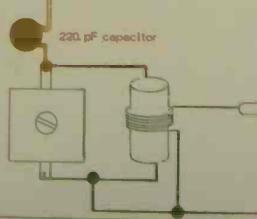
Again we can use this 'double' aerial coll with the serial wire connected via a 220 pF capacitor. Note that the main (aerial) coll is guite separate from the coupling coll as repards conflections.
