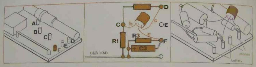
1. The circuit panel is made up as previously, but with the hole not used (F) also fitted with a 6BA terminal screw. There are now six terminal points, A, B, C, D, E and F.
