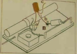
Transistors come in all shapes and sizes I For simple radio circuits you need only an inexpensive type like an OC70, OC71, NKT 214, 2N280, 2N1305, AC122, AC125, or equivalent.
