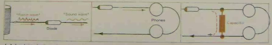
4 A broadcast signal consists of 'sound waves' superimposed on 'radio waves'. A diode can act as a *detector* to separate the sound wave content from the radio waves and pass this on.
