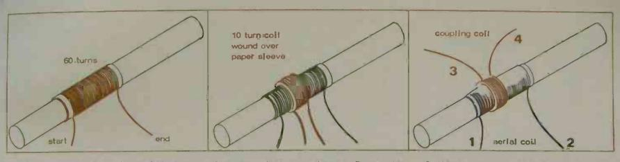
1. Make a papel sleeve to fit a ferrite rod, as on pages 8/9, and wind on a 60-turn coil of 38 s.w.g. wire with no tapping point. Secure the start and end with cement: 2. Make a short paper sleeve to fit over this coil. This should be a loose fit southat you can slide it up and down the first coil. The best position is found by experiment.
