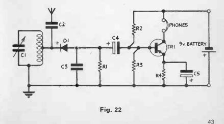
This involves two additional resistors and one additional capacitor. A theoretical diagram of this circuit (*fig. 22*) uses the following components:
