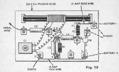
C4—8 microfarad capacitor. This is an *electrolytic* type, marked with a plus sign on one end, and must be connected the correct way round.
