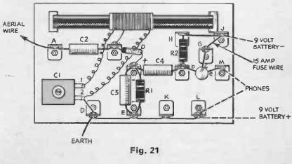
The emitter lead (e) of the transistor is connected to this tag, and to one lead of the phones. The other lead of the phones goes to tag L. Tags G and J are connected with a short length of 15 amp fuse wire.
