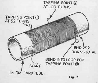
Use a 6BA brass bolt and nut to connect a length of insulated wire to one side of the variable capacitor from tapping point 2 for medium wave; and from tapping point 3 for long wave. Tapping point 1, of course, connects to the diode and aerial.
