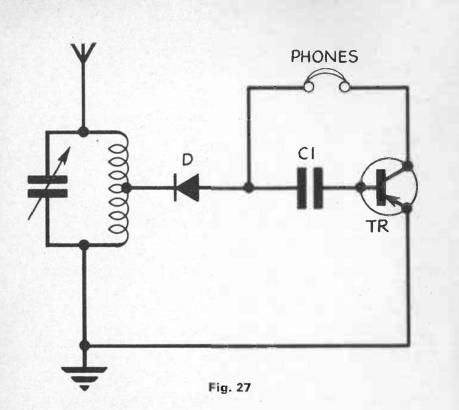
the diode to the base of the transistor (*fig.* 27). Use a Mullard OA70 or OA71 diode, and a Mullard OC70 or OC71 transistor.
