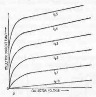
Fig. 906-b. Output characteristic curves of grounded-emitter.
