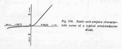
in the direction of the arrows. There can be no significant recombination, and the junction resistance appears high. As a result of this action, the current flow is low.
