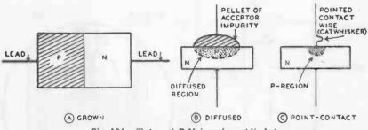
Fig. 104. Types of P-N junctions (diodes).
