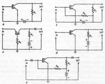
Fig. 404. Typical single-battery amplifier stages.
