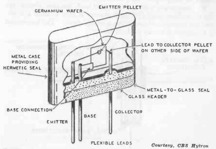
Fig. 205. Cutaway view showing inner construction details of junction transistor.
