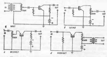
Fig. 409. Positions of the gain control in amplifier circuits.
