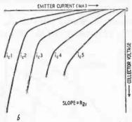
Fig. 905-b. Forward characteristic curves.
