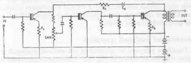
Fig. 405. Resistance-coupled 3-stage transistor amplifier.
