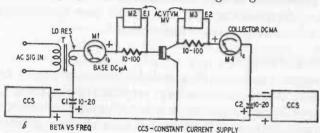
Fig. 912-b. Test circuit for checking base-to-collector current amplification.
