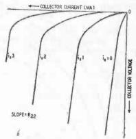
Fig. 903-b. Output characteristic curves.
