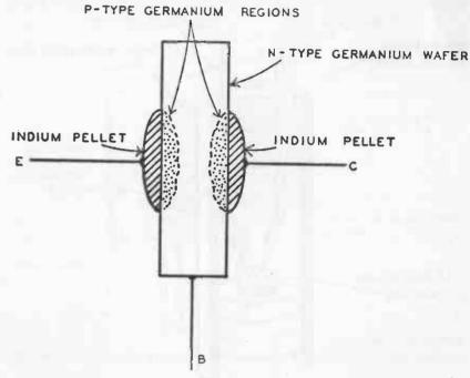
Fig. 203. Construction details of diffused P-N-P transistor junction.
