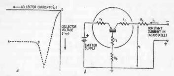
Fig. 215. Curve showing property of negative resistance in collector circuit.
