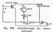
initially by applying an accurately-known d.c. input current corresponding to full-scale deflection of the meter, and adjusting the calibration control rheostat R1 for full-scale deflection. When a 0-1 milliammeter is used, this input current should be 25  $\mu$ a for the CK721 or 100  $\mu$ a for the CK722. With a 0-100 microammeter, a 2.5  $\mu$ a calibration current is used with the CK721 and 10  $\mu$ a with the CK722.
