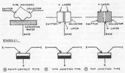
Fig. 202. Point-contact and junction type transistor triodes.
