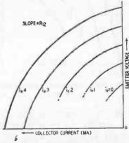
Fig. 904-b. Feedback characteristic
