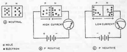
Fig. 105. Effect of junction bias voltage.
