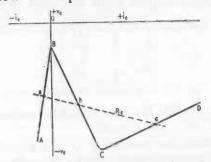
Fig. 704. Emitter negative-resistance characteristic with multiple operating points.
