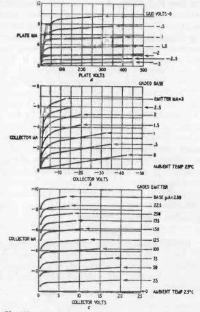
Fig. 213. Transistor collector current vs. collector voltage curves compared with vacuum-tube characteristics.
