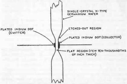
Fig. 207. Detail of surface-barrier transistor cross-section.
