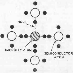
Fig. 102. Acceptor-impurity atom in semiconductor.
