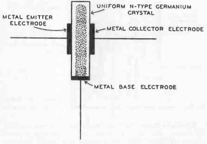
Fig. 206. Schematic cross-section of surface-barrier transistor.
