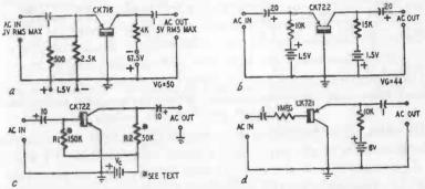
Fig. 801. Resistance-coupled, single-stage a.f. amplifiers.
