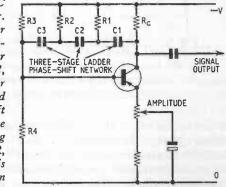
are many variations of it. One important use of the principle is the self-oscillating mixer which was described in Chapter 5 (Fig. 5.1). There are, however, a number of other approaches to sinewave oscillator design. Three fairly widely used circuits are the RC oscillator, the Wien bridge oscillator and the crystalcontrolled oscillator. The two first are used mainly for the generation of low-frequency sinewave signals.
