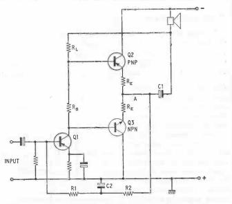
Fig. 4.5. Complementary symmetry output stage, using a pnp and an npn transistor, with single-ended output connection. The load  $R_L$  of the driver transistor Q1 is a.c. coupled to the emitters of the output transistors via C1 so that the output transistors operate in the commonemitter mode. The d.c. feedback network R1, C2, R2 is often used with this circuit.
