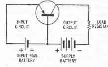
Fig. 1.16. Circuit diagram of the type of circuit, LOAD the common-base circuit, RESISTANCE shown diagrammatically in Fig. 1.15. In this case, however, a pnp transistor is shown, with the polarities of the bias batteries reversed accordingly.
