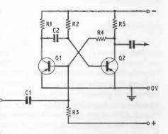
the circuit from the stable to the unstable state, and after a time determined by the time constant of the single RC coupling network the circuit reverts to its stable condition.
