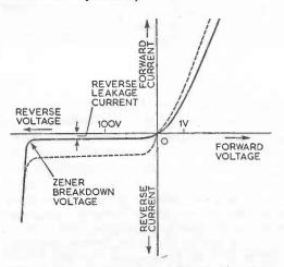
Fig. 1.11. Characteristics of a pn junction. The broken-line curves show the effect of increase in temperature on the characteristics.
