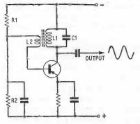
Fig. 3.10. If the LC-tuned circuit load is coupled back to the base by means of a small coupling winding L2, as shown here, a simple r.f. oscillator is obtained providing a sinewave output at a frequency determined by the values of L1 and C1.
