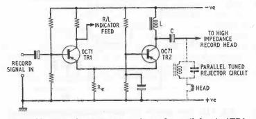
Fig. 4.11. Record output stage using a long-tailed pair (TR1, TR2) in which the coupling between the transistors is via the shared emitter resistor R<sub>e</sub>. With this arrangement the output transistor TR2 operates in the common-base mode.
