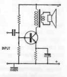
illustrated transistor a.f. amplifier stages is the use of a transformer in the collector circuit to match the transistor output impedance to the impedance of its load—the loudspeaker—maximum power being fed to the loudspeaker when these two impedances are the same. To obtain maximum power gain in the output stage, the common-emitter configuration is used, and a step-down transformer, as shown, is needed to match the low impedance of most types of loudspeaker to the relatively high
