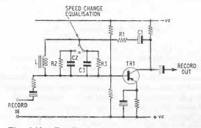
Fig. 4.12. Equalisation by means of a frequencyconscious feedback loop.
