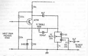
Fig. 4.8. Voltage amplifier stage incorporating tone control networks. Note polarity of electrolytic coupling capacitors. The treble tone control takes the form of a frequency-conscious variable feedback network, the bass control being in a 'passive' circuit.
