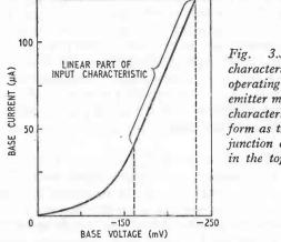
Fig. 3.3. Typical input characteristic for a transistor operating in the commonemitter mode. Note how the characteristic has the same form as the basic forward pn junction characteristic shown in the top right quadrant in Fig. 1.11.
