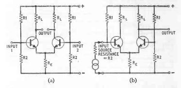
Fig. 6.11. Basic differential amplifier circuits: (a) 'push-pull' version, (b) single-ended input and output version.
