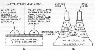
Fig. 2.3. Stages in the manufacture of a germanium alloydiffused transistor. (a) p-type wafer forms collector region, n-type layer being diffused into it to provide the base region. E and B are pellets which are alloyed on to the n-type diffused layer, the former to provide an emitter region and the latter to provide an ohmic connection to the base region. (b) Active part of the alloy-diffused transistor after alloying, with connecting leads to the base and emitter regions.
