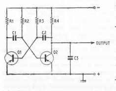
Fig. 5.15. The basic multivibrator circuit, used as a timebase waveform generator. The waveform is again developed as a result of C3 charging and discharging. The multivibrator consists of two RC coupled amplifier stages cross-coupledfrom collector to base -to each other.
