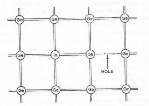
Fig. 1.7. Germanium crystal lattice incorporating a trivalent indium atom (In), showing the hole in the crystal lattice structure created by the impurity atom accepting an electron to complete its covalent bonds with adjacent germanium atoms. (Elements having three valence electrons are termed 'trivalent'.)
