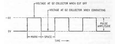
Fig. 6.1. The output from the collector of an astable symmetrical (i.e. R1 = R4, R2 = R3, C1 = C2 in Fig. 5.15) multivibrator is a square wave as shown here when the charging capacitor shown in Fig. 5.15 (C3) is omitted. This is an ideal waveform to show the principle: in practice, the sides of the waveform would not be perfectly vertical nor the top of the pulses perfectly flat.
