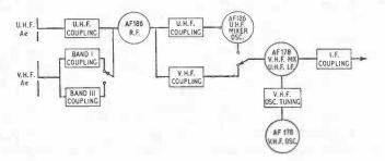
Fig. 5.13. Integrated u.h.f./v.h.f. tuner units are used in some television receivers. This block schematic shows a typical arrangement.
