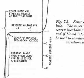
Fig. 7.3. Zener diode characteristic. The zener diode has a low reverse breakdown or zener voltage and if biased into this region can be used to stabilise voltage against variations in current.
