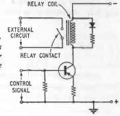
circuit, it is usual to connect, as shown, a diode across the coil to overcome the potentially damaging voltage peak that occurs when the field in the relay coil collapses on Q1 cutting off and the relay de-energising.
