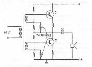
Fig. 4.3. In this push-pull output stage the two transistors are fed from separate windings on the driver transformer, thermistors are included in the base bias networks to provide stabilisation against the effects of temperature variation, and the loudspeaker is coupled by means of a capacitor (C1) to the centre-point of the output stage—an arrangement sometimes referred to as 'single-ended output'.
