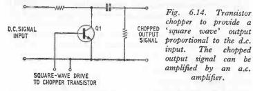
this is that the transistor short-circuits the d.c. signal input when it is switched on, and a square-wave output proportional to the d.c. input is obtained. A transistor may similarly be used to 'demodulate' the signal after it has been passed through the a.c. amplifier.
