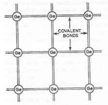
Fig. 1.2. Diagrammatic representation of the germanium crystal lattice structure at absolute zero temperature, showing the two-electron covalent bonds that exist between adjacent atoms.
