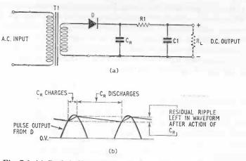
Fig. 7.1. (a) Basic half-wave rectifier circuit fed from a transformer, with reservoir capacitor  $(C_R)$  and RC filter circuit R1, C1 to smooth out the rectified a.c. (b) Waveforms showing the pulse output from the rectifier D and the action of the reservoir capacitor.
