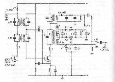
Fig. 5.11. Typical dual-channel i.f. stages of an a.m./f.m. receiver. Standard i.f.s are 10.7 Mc/s for f.m. and 470 kc/s for a.m. The higher frequency i.f. transforms are connected nearest to the collectors of the transistors. The f.m. demodulator comprises a ratio-detector circuit X1, X2.
