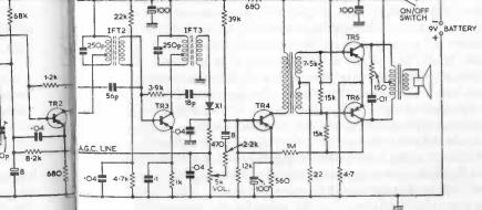
resistor (10 k) in this network must be decoupled at signal frequency  $(0.04-\mu F \text{ capacitor})$ . TR2 and TR3 i.f. amplifier stages are provided with unilateralisation networks. X1 detector, TR4, a.f. amplifier, TR5 and TR6 push-pull output stage.
