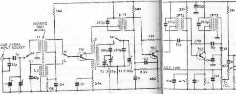
Fig. 5.3. A typical six-transistor, two-waveband (L.W. and M.W.) radio receiver using alloy-junction transistors throughout. TRI is self-oscillating mixer. Note that the input coupling windings are in series with the base bias potential divider network so that the lower accurately in relation to each other—track correctly, as it is called. Also for alignment purposes ferrite tuning cores are incorporated in the oscillator and mixer output tuned circuits.
