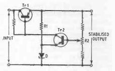
stabilised output voltage from the circuit. A change in the voltage at Tr1 junction is used by the feedback circuit to alter Tr1 base bias so that it passes a greater or smaller current. A common variation of the circuit shown is the use of a compoundconnected pair of transistors in position Tr1.
