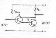
follower and compound-connected pair. The circuit consists of a pair of transistors, often in fact supplied as an integrated pack, with the two collectors connected together and with the base of the
