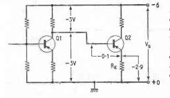
Fig. 3.8. Directly coupled transistor amplifier stages. The value of  $R_E$  is chosen to establish the correct base bias for the second stage when it is fed direct from the collector of the first stage.
