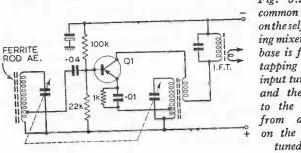
Fig. 5.2. Some common variations on the self-oscillating mixer. Here the base is fed from a tapping on the input tuned circuit and the feedback to the emitter is from a tapping on the oscillatortuned circuit.
