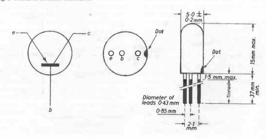
Fig. 2 Details of transistor connections
