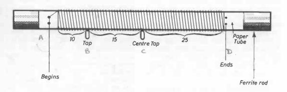
Fig. 4 The special coil for the receivers described in Chapters 3 and 4
