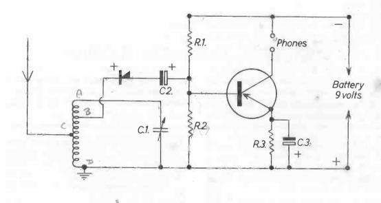
Fig. 3 Theoretical circuit of the diode/transistor receiver
