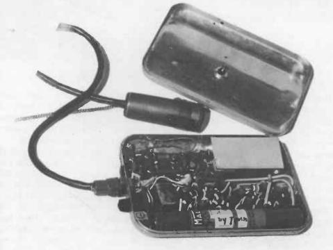
Fig. 27 BBC radio microphone using semi-conductors
