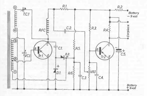
Fig. 6 Theoretical circuit of the two-transistor pocket receiver
