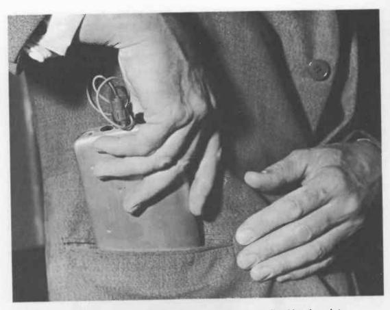
Fig. 28 Showing how easily the BBC radio microphone can be slipped into the pocket
