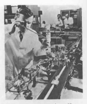
Fig. 22 A new automatic system for assembling computer transistors at the rate of 1,800 an hour—developed by IBM
