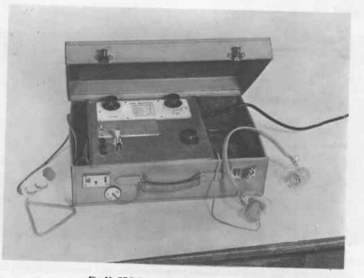
Fig. 29 BBC Outside Broadcast suitcase apparatus
