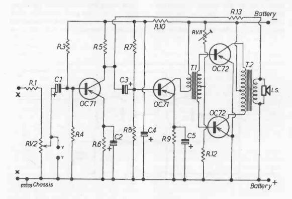
Fig. 14 An audio-amplifier with push-pull transistor output
