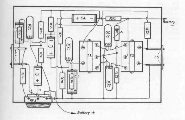
Fig. 15 Wiring diagram of the transistor audio-amplifier
