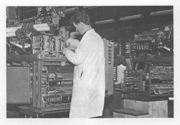
Fig. 26 Miles of complicated wiring go into a high-speed IBM accounting machine, here shown being assembled at their Greenock factory
