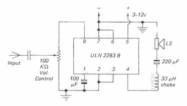
Figure 20. Schematic diagram of amplifier using ULN 2283 B. (Reproduced by courtesy of Ambit International)
