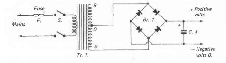
Figure 28. A mains unit for power supply. Components required: F - 1 to 3 amp. fuse. S - Double-pole mains switch. Tr.1. - Mains transformer 9-0-9 volts 1 amp. Br.1. - Bridge rectifier 1 or 2 amp. 100 volt p.i.v. C.1. - Electrolytic capacitor 4,700 mfd. 25v. wkg.
