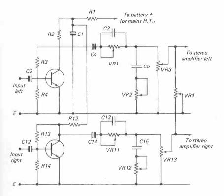
Figure 24. Pre-amplifier for stereo amplifier.
