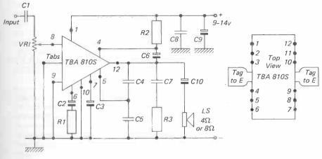
Figure 14. Audio Amplifier using TBA 810 S.
