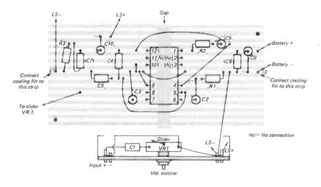
Figure 15. Veroboard mounting for Amplifier shown in Fig. 14. Components are mounted on the upper side which is clear of copper strips, and lugs, wire ends etc. are passed through the holes.
