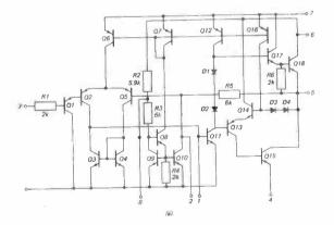
Figure 31. TBA 820 M Chip. (above and next page) (Reproduced by courtesy of Ambit International) (a) Internal connections.
