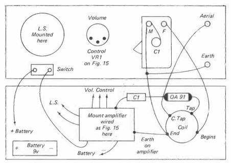
Cut out corner of back to allow insertion of battery. Make leads long enough to connect up to battery before insertion.
