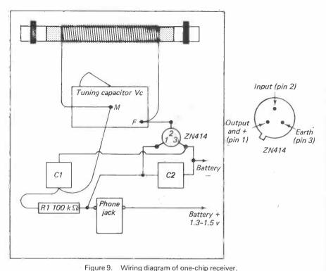
Components required: Ferrite rod — 5 ins. or 13 cm. long Wire — see text Tuning capacitor Vc — solid dielectric 500 pF variable (but see text) C.1. 0.01 mfd. capacitor (fixed) C.2. 0.15 mfd. capacitor (fixed) R.1. 100 kilo-ohm resistor (fixed) ZN 414 Ferranti single-chip integrated circuit Phone jack or two terminals Earphone (see text)
