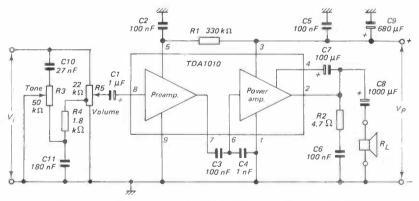
Figure 22. Complete mono audio amplifier using Mullard TDA 1010. (Reproduced by courtesy of Mullard Ltd.)
