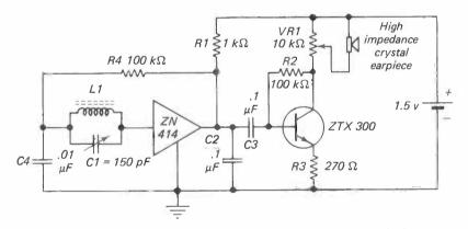
Figure 11. Adding a Transistor Amplifier to circuits in Figures 9 & 10. (Reproduced by courtesy of Ferranti Ltd.)
