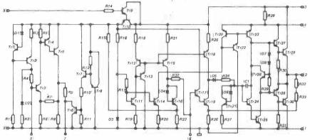
Figure 21. Internal connections of Mullard TDA 1010 chip. (Reproduced by courtesy of Mullard Ltd.)
