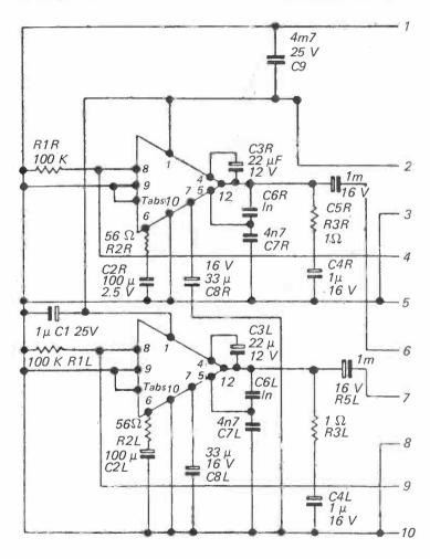
Figure 18. Stereo amplifier using IC's TCA 940
