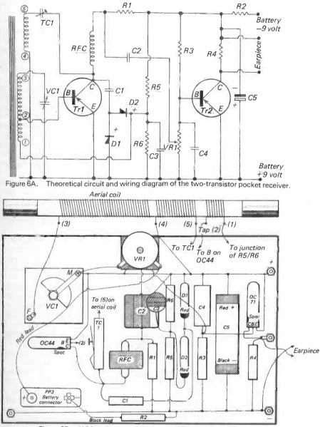
Figure 6B. Wiring diagram of the two-transistor pocket receiver.
