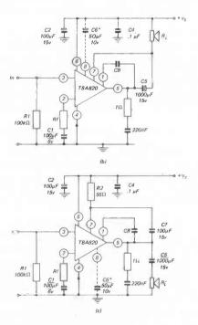
Figure 31. TBA 820 M Chip. (see also previous page) (Reproduced by courtesy of Ambit International) (b) Loudspeaker connected to supply. (c) Loudspeaker connected to ground (earth).
