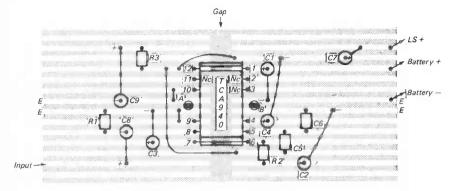
Figure 17. Veroboard layout of TCA 940 amplifier.
