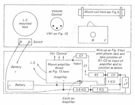
Figure 26. Wiring diagram of a one-chip and amplifier receiver.
