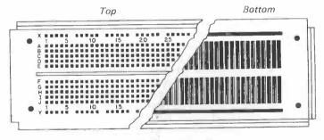
Figure 3. The C S C "breadboard".
