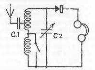
Fig. 4 Crystal Set Theoretical Diagram
