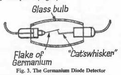
A crystal set has no power to amplify the signals which it receives via the aerial and the crystal detector merely converts the radio signals into currents capable of actuating the diaphragms of our headphones and producing sounds thereby.
