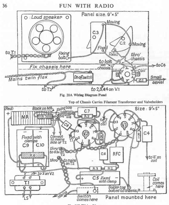
Fig. 20B Wiring Diagram
