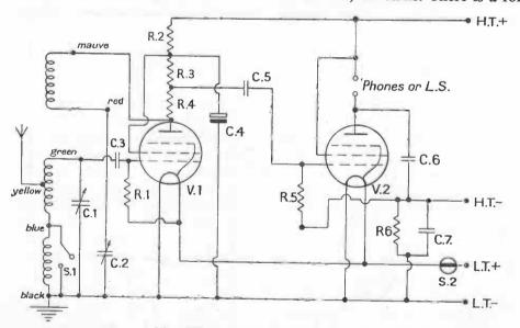
Fig. 9 Battery Two-valve Receiver **Theoretical Diagram**
