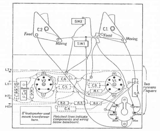
Fig. 10 Battery Two-valve Receiver Wiring Diagram
