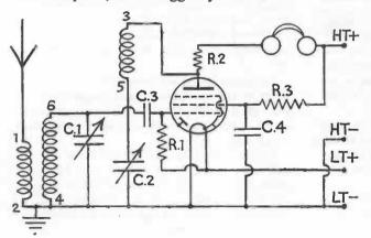
Fig. 7 One-Valve Set Components required: Wood for baseboard and panel B7G valveholder C.1. 0005-mfd. variable capacitor Repanco DRR 2 coil (see text) C.2. 0001-mfd. variable capacitor C.3. 0002-mfd. fixed capacitor C.4. 11-mfd. bypass capacitor R.1. 2-2-megohm grid leak R.2. 10,000-ohm fixed resistor R.3. 5-megohm resistor Headphones, wire, terminals, etc. DAF 91 or 96 valve On-off switch for wavechange
