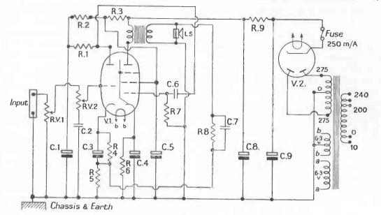
Fig. 23 Basic Diagram for 2-valve amplifier
