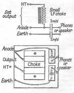
Fig. 18 Output Filter Circuit
