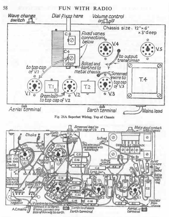
Fig. 28B Superhet Wiring Diagram
