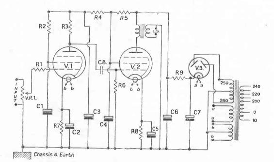
Fig. 24 Basic Diagram for 3-valve amplifier
