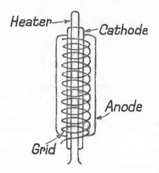
Fig. 14 An Indirectly Heated Triode
