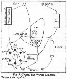
Components required: •0005 mfd. solid dielectric variable capacitor (C.2) On-off switch DRR 2 coil (Repanco) •0002-mfd. fixed capacitor (C.1.) Germanium diode (Osram GEX 35 or Mullard OA 81) 4 terminals or 2 double mounts Crocodile clip Wood, wire, etc. Tuning knob
