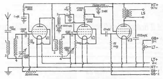
Fig. 11 Three-Valve Battery Receiver. Theoretical Diagram
