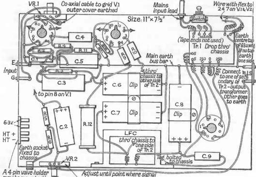
A 4-pin valve-holder may be mounted here to give a supply for a feeder unit for radio.
