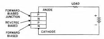
Figure 30. Three-junction (PNPN) semiconductor
