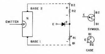
Figure 26. Unijunction transistor
