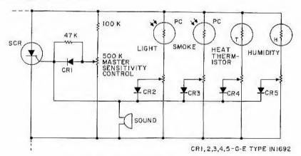
Figure H3.8 Multiple detector input circuit
