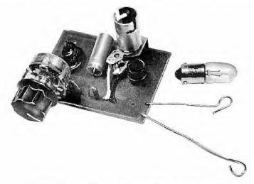
Figure E3.4 Light flasher assembled on circuit board
