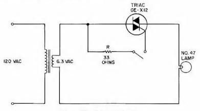
Figure 39. Triac test circuit
