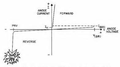
Figure 31. Three-junction (PNPN) semiconductor characteristic
