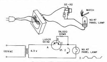
Figure 35. Electric candle circuit
