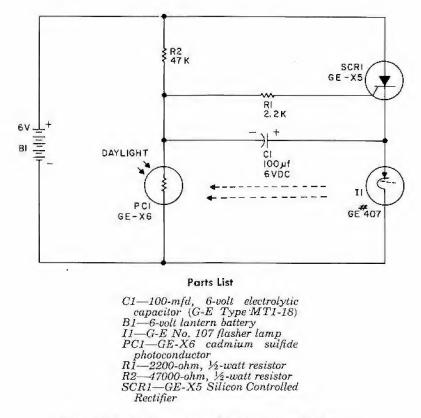
Figure E4.1 Battery-operated flasher schematic diagram
