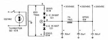
Figure W11.3 Alternate silicon rectifier replacement circuit resistance in each leg
