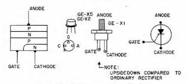
Figure 32. Silicon-controlled rectifier (SCR)
