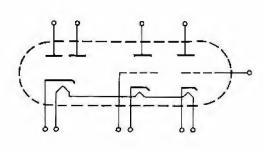
Figure 8. One type of Compactron
