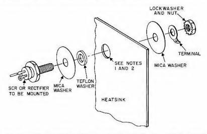
NOTES: I. DRILL HEATSINK HOLE TO TIGHTLY RECEIVE THE TEFLON WASHER.
