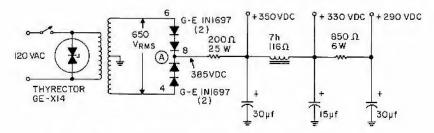
Figure W11.2 Alternate silicon rectifier replacement circuit resistance in load
