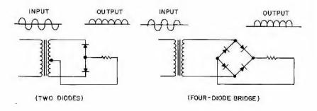
Figure 11. Solid-state full-wave rectifier circuits
