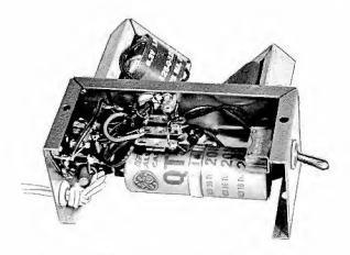
Figure E10.6 Power supply with cover removed
