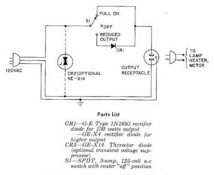
Figure H1.1 High-low switch schematic diagram
