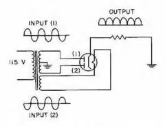
Figure 4. Diode connected for full-wove rectification
