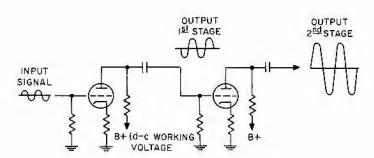
Figure 6. Two-stage triode amplifier
