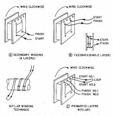
Figure A5.4 Transformer bobbin winding instructions
