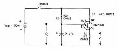
Figure 28. Relaxation oscillator circuit
