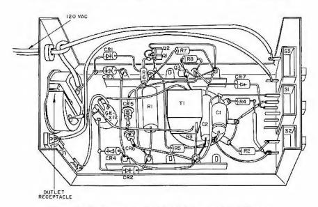
Figure H5.2 Time-dependent light dimmer pictorial diagram
