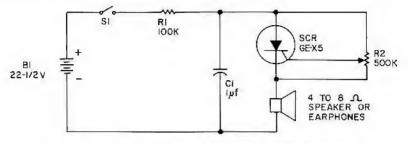
Figure H3.1 Basic relaxation oscillator schematic diagram
