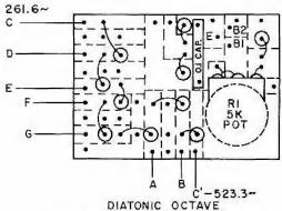
NOTE: USE POTENTIOMETER SHAFT NUT AS MOUNTING DEVICE.
