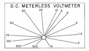
Figure W8.2 Scale used with calibrating potentiometers
