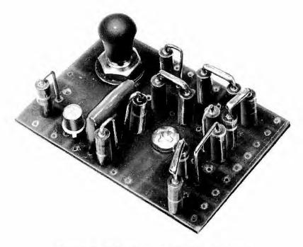
Figure E7.3 Unijunction organ circuit board showing mounted components—Diatonic
