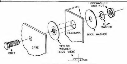
NOTE: FILE OFF ALL DRILL BURRS IN CASE AND HEATSINK. Figure 45. Insulated heatsink mounting
