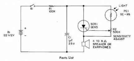
C1—1-mfd, 25-volt (minimum) capacitor (G-E MTI-1) PC1—GE-X6 cadmium sulfide photoconductor R1—100000-ohm, 1-watt resistor R2—500000-ohm, 2-watt potentiometer
