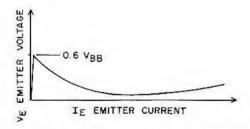
Figure 27. Unijunction transistor characteristic
