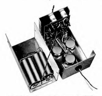
Figure W6.2 Multimeter adapter construction details
