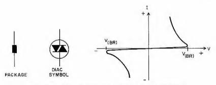
Figure 40. Symbol and characteristic of the Diac (GE-X13)
