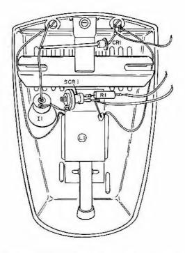
Figure A1.2 Battery-saver pictorial diagram (negative ground)
