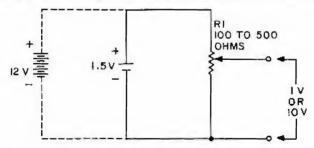
Figure W6.3 Voltage calibration source for adapter
