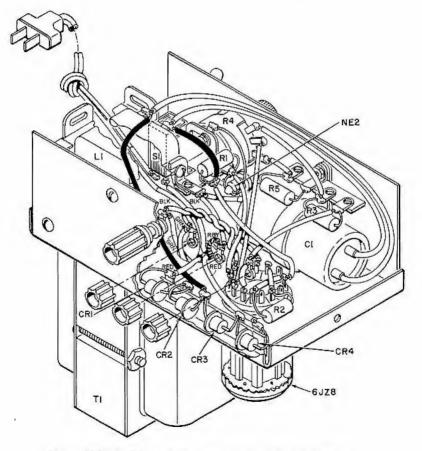
Figure W10.4 Regulated power supply pictorial diagram
