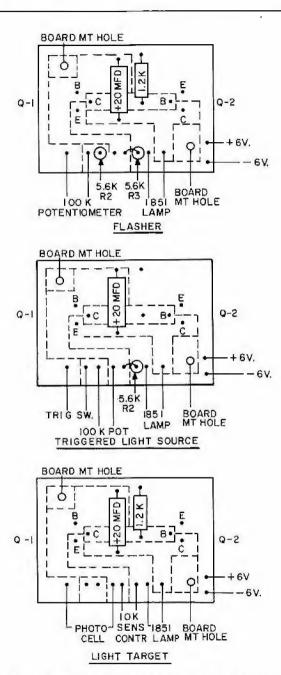
Figure E3.5 Parts location on printed circuit board
