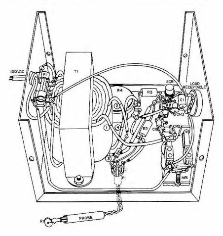
Figure W2.2 Basic temperature-operated relay pictorial diagram
