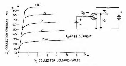
Figure 25. Transistor characteristic curves
