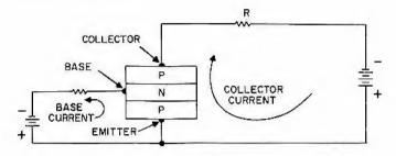
Figure 20. PNP transistor
