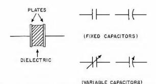
Figure 1. Capacitor—Elementary construction and symbols
