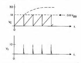
Figure 29. Relaxation oscillator circuit waveforms
