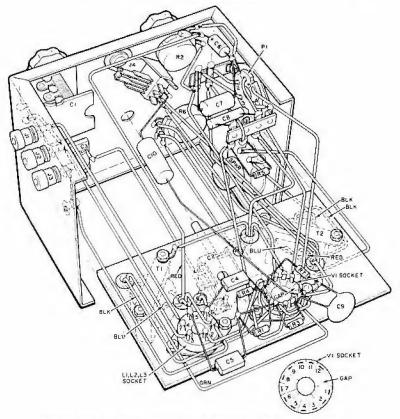
Figure E10.5 One-compactron receiver pictorial diagram
