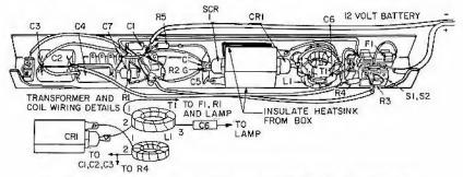
Figure H6.2 Battery-operated fluorescent light pictorial diagram
