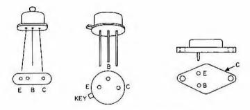
Figure 23. Transistor case styles
