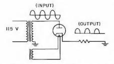
Figure 3. Diode connected for half-wave rectification
