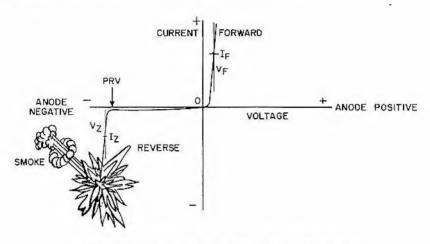
Figure 15. Solid-state rectifier characteristic curve
