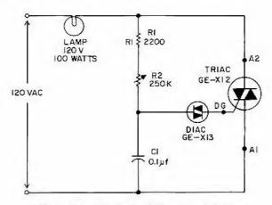
Figure 41. Basic Triac/Diac control circuit
