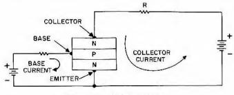
Figure 21. NPN transistor
