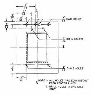
Figure A5.3 Transformer bobbin drilling dimensions
