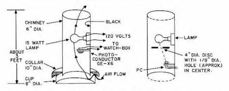
Figure H3.6 Cross-section view of smoke detector
