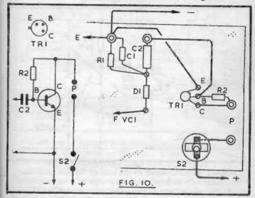
TR1, R2 and S2 are connected as shown. For TR1, a BC108, 2N706, or similar general purpose NPN transistor will be satisfactory. R2 can generally be 1 megohm with satisfactory results, but it can be worth while trying values from about 100k to 2.2 megohm here, as performance depends on the transistor, phones, and battery voltage.
