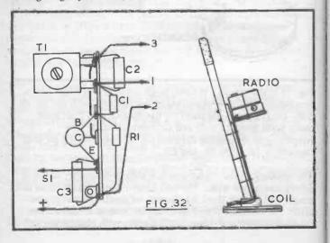
A shelf is bolted to the handle, and the detector rests on this, with connections passing down to the search coil. A few loops of tape or string will secure these to the handle.
