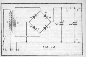
Sometimes R1 and C2 are omitted. Should hum accompany reproduction from an amilifier, this shows that smoothing is probably inadequate, and if so the cure is to add R1 and C2.
