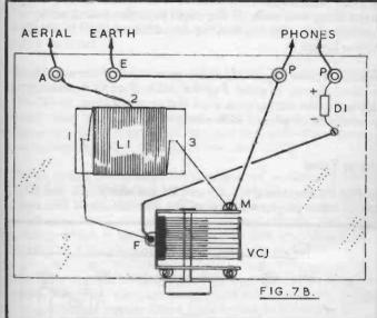
Four terminals, for Aerial, Earth, and Phones, will complete the receiver. Best results will be had by connecting a good headset, of about 500 ohm to 2,000 ohm. Very low impedance earpieces, such as are employed with some transistor receivers, are not suitable here.
