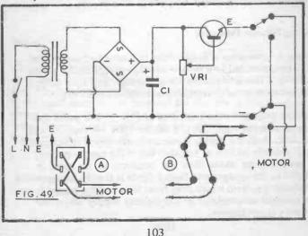
A transformer with a 12v secondary will be suitable for the usual model requiring up to 12v. The circuit is similar to that of the supply in Fig. 47. The potentiometer VR1 gives speed control. C1 can be around  $2,000\mu$ F.
