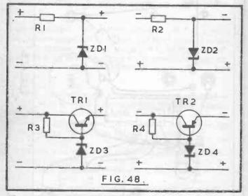
The second circuit is virtually the same, but polarity is reversed, so that the ground return is positive.
