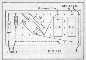
A screened input circuit will be found necessary when the IC amplifier is used with a preamplifier or similar items. Connect the outer brading of this lead to the negative line, and the inner conductor to C1. Such screening is not necessary with very short connections from other stages to the IC amplifier, or when using it to amplify a crystal diode radio, or for similar purposes.
