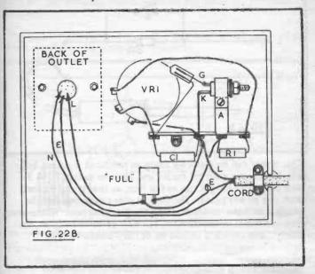
If a fully insulated box is used instead, then the bush of VR1 and of the switch should both be earthed by wires, except when these items are constructed wholly with insulated material. (This precaution is necessary to avoid any chance of metal parts outside the box becoming "live".)
