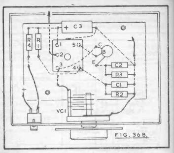
An insulated lead is run from 2 on the IFT, and is placed near the receiver. This lead may be so positioned as to give best coupling into the IF stages of the receiver. If coupling is too weak, the signal from the CW/SSB Resolver will be inadequate. On the other hand, tight coupling will allow the carrier to swamp weak signals tuned in on the receiver. Fortunately the degree of coupling is not at all critical.
