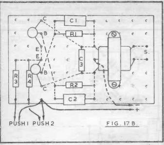
In some circumstances it may be convenient to run a single twin lead from Push 1 on to Push 2, including an extra resistor at Push 2 itself, to modify the tone. This may save taking leads from Push 2 all the way back to the oscillator board.
