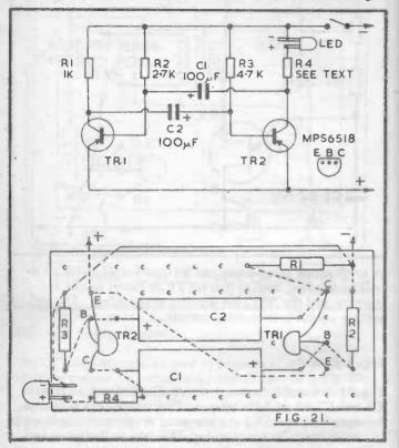
C1 and C2 need only be 6.4v working, and the device can be assembled on a very small perforated board. See p.61 for LED polarity.
