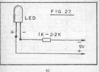
found by trial – the correct connections are those allowing the LED to light. The series resistor may be about 150 ohm to 1k or more, depending on the actual voltage, and brightness required. Current drawn varies with different LEDs, and with voltage and series resistance, but can be about 5mA or less, without reducing the brightness too far.
