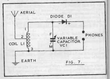
Fig. 7B shows the practical layout. It is convenient to use an insulated board larger than necessary, so that a transistor amplifier can be added later. A board about  $5 \times 8$  inch is suggested, and it can be supported on 1 inch high runners (strips of wood) so that there is clearance for screws or terminals.
