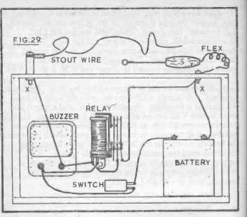
If loop and wire touch, current flows from the battery to the buzzer, which sounds. Current also flows to the relay winding, so that the relay contacts close. Even a momentary contact between loop and wire will thus cause the buzzer to sound until the switch is used to break the circuit.
