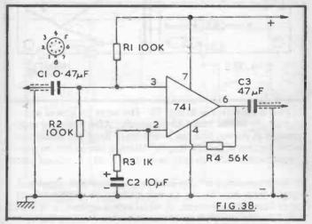
Modification to the values of R3 or R4 allow feedback and gain to be adjusted between quite wide limits, but for general purposes the values shown are satisfactory. A wide range of voltages (not exceeding 36v) may be used. The actual output is from a complementary pair, and is easily adequate for very good headphone volume, if required.
