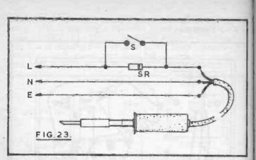
This device can be made by using an insulated junction box which will take a socket outlet and also the switch S. A 3core cord with plug is run to the box, so that it can be used with any power point. The iron or other item can then be plugged into the outlet fitted to the junction box. Remember to make mains connections in the way described earlier, for safety. The switch S should be of fully insulated type.
