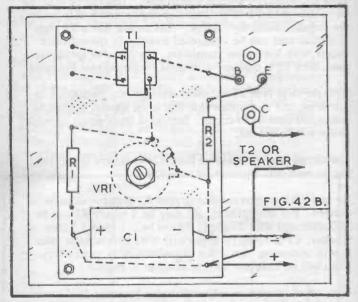
The insulated board carrying the other components is mounted by long bolts with extra nuts. A large Class A stage transistor of this type will grow very warm to the touch, if run at anything like maximum power rating. This does not indicate any defect.
