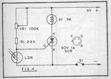
The second device is the silicon controlled rectifier SCR. Normally, this does not allow current to pass from its cathode K to its anode A. However, a small current applied to its gate G will trigger it so that it conducts from cathode to anode. It remains in this state even when gate current is removed. It is restored to the non-conducting state by removing the voltage from its cathode, by opening switch S1.
