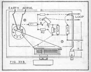
Fit a small slide switch to the box front, and aerial and earth sockets to the back, near the coil. A 9v battery is accommodated in the case.
