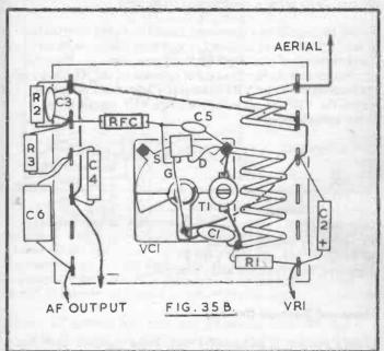
The larger coil has five turns of 18 swg wire, and is  $\frac{1}{2}$  inch in diameter and  $\frac{3}{4}$  inch long. The smaller coil has two turns. Wiring to VC1, T1, C5, the coil and C1 must be as short as can be arranged. Connections elsewhere are reasonably direct. A ceramic disc capacitor may be used at C1. T1 should be a low loss trimmer.
