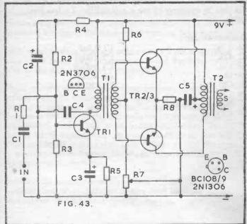
T1 is the driver transformer, with centre tapped secondary, so that TR2/3 may be operated in push-pull (see Fig. 12). T2 couples output to a 2/3 ohm speaker.
