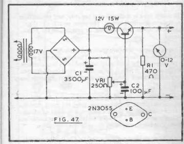
VR1 is panel mounted, and allows the base potential of the control transistor to be set at the required voltage. C2 provides "electronic smoothing" from the base circuit.
