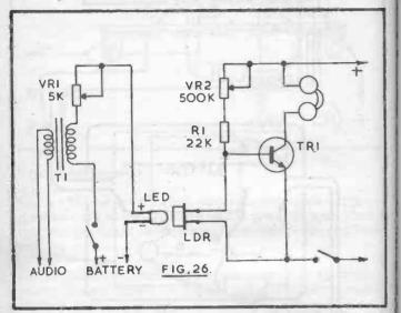
Electrically, the device is in two sections. The first has the light emitting diode LED, VR1, and transformer T1. When the battery is switched on, current flowing through the LED is adjusted by VR1, so that the LED glows dimly. A signal voltage in the secondary of T1 then modulates the LED light intensity.
