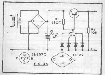
R1 supplies current for any diode, and 1 watt diodes should be used. With a 24v transformer and large transistor such as the 2N1970 or 0C29, an output of up to 1 ampere can then be drawn. The bridge rectifier must of course be rated at 1A or higher.
