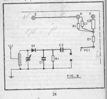
may be considered as replacing the headphones. C2 is a coupling capacitor passing audio signals to the following amplifier.
