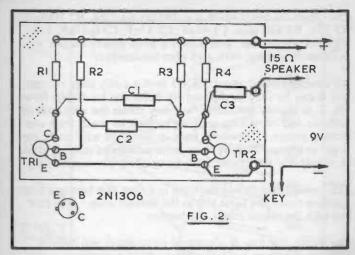
Fig. 2 shows the practical assembly of the device on an insulated board. A theoretical circuit is given in Fig. 14, and is not repeated here, so Figs. 2 and 14 should be looked at together.
