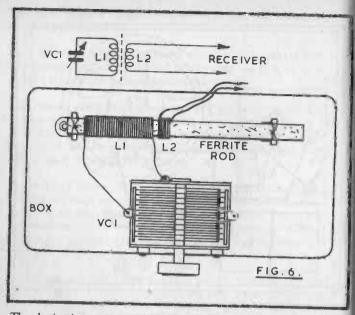
The device is constructed in a plastic lunch box about  $6 \times 4 \times 4$  inch or other *insulated* case. Some boxes of this kind, though strong, are of brittle material. These must be drilled without too much pressure, or they may crack. Drill points should also be sharp.
