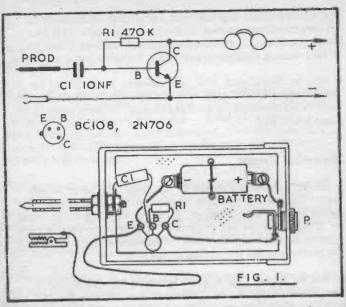
Resistor R1 is connected from collector C to base B, and it supplies a base current for the transistor, so that the latter can operate as an amplifier.
