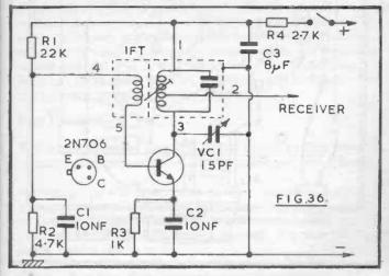
Most popular receivers have an intermediate frequency of about 455kHz to 470kHz. The circuit in Fig. 36 uses an intermediate frequency transformer of similar type, and adjustment of its core allows operation with any IF from 455 to 470kHz. Pin numbers are for the Denco (Clacton) IFT13, normally intended for 465kHz. The connections to the base winding (4 and 5) have to be phased to secure oscillation.
