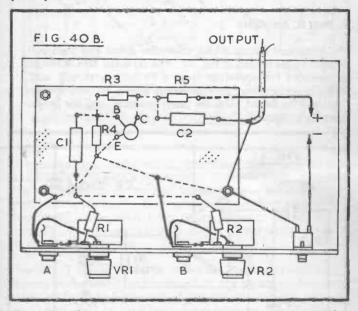
Fig. 40B is the layout, using a metal case or box. A screened output lead is provided. Input sockets A and B may be chosen to suit the type of plugs on existing equipment. The on-off switch is separate from the potentiometers, so that these can be left at pre-set levels if wished.
