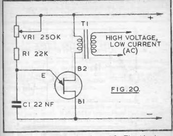
A small mains transformer can be used for T1, with a low voltage winding, such as that for a 6.3v heater circuit, as primary, and the 200/250v winding as secondary. The high voltage output is alternating current.
