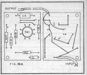
Lead 8 is identified as in Fig. 38. The wires are spread out slightly, to fit the board perforations. After inserting components as shown, turn the board over. Bend and solder the wires, cutting off excess length. Sleeving can be put on any connections which run very near other leads or soldered joints.
