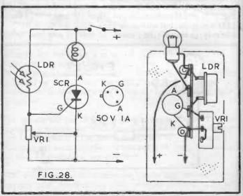
The LDR has a high resistance when in darkness or subdued light, so that the gate potential of the SCR is not sufficiently high to trigger this device. When light reaches the LDR, its resistance falls, and the SCR gate voltage rises. The SCR then moves into its conducting condition, so that current flows through the bulb. The sensitivity of the circuit, or level of illumination needed to trigger the SCR, is set by VR1.
