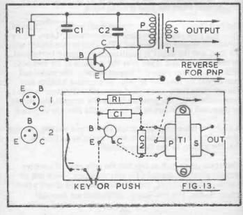
(1) shows leads from a typical NPN transistor, such as the BC108, 2N706, and similar types. (2) is the base of the PNP AC128 transistor.
