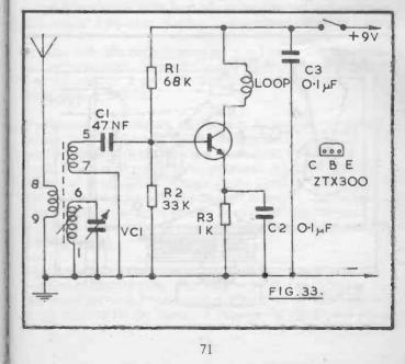
Fig. 33 is the circuit, and it uses a cored tuning coil with aerial coupling winding 8-9, tuned winding 6-1, and base coupling coil 5-7. These numbers are for the pins of the Denco (Clacton) "Blue" Range 2 component. It will be apparent that other coils, or surplus or home-wound inductors, can be substituted.
