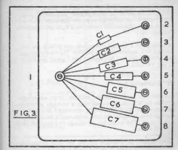
Such a box is easily made as in Fig. 3, using a plastic or other insulated case. Here, point 1 is common to all the capacitors, and any capacitor can be selected by connecting to points 2 to 8. Connections can be taken to 6ba bolts, using extra nuts. An alternative is to have eight sockets, with a pair of test leads equipped with plugs.
