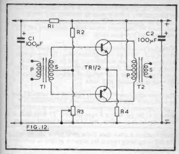
R2 and R3 set the base bias conditions for the transistors. Bias is arranged so that collector current is low, when no audio signal is present. The emitter bias resistor R4 limits peak collector current.
