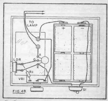
Fig. 4B shows constructional and wiring details. The SCR is mounted on a small insulated board. Clear bared wires are twisted tightly to the LDR, so that this also can be fitted by small bolts and nuts, as shown. The connections to VR1 are also tightly twisted and pressed together with pliers.
