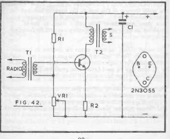
T1 is the coupling or driver transformer, which may receive audio signals from a radio receiver, smaller amplifier, or other equipment. A step down ratio of about 5:1 to 10:1 will generally prove to be suitable.
