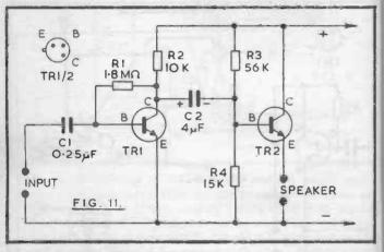
C1 couples the audio signal to the base of the first amplifier TR1, which receives base current through R1. An amplified signal is developed across the collector resistor R2, and is coupled to the base of the following amplifier TR2 by means of C2.
