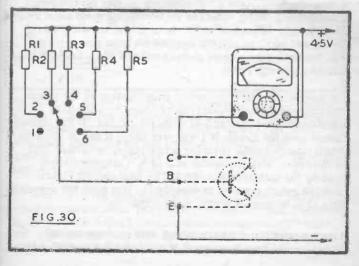
Polarity is shown for NPN transistors. Reverse polarity of both meter and battery for PNP transistors.
