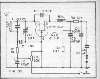
Control of super-regeneration is by means of the potentiometer VR1, which adjusts the FET drain potential. The value of VR1 is not very important, but a linear potentiometer is necessary.
