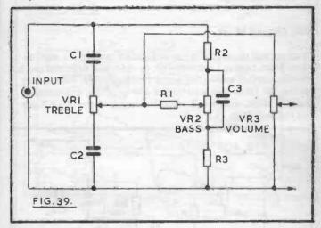
The tone control is a passive circuit, needing no battery, and it can be placed between the source of audio signals (generally a microphone, pick-up, or radio tuner) and the amplifier or preamplifier. It may also be located between preamplifier and main amplifier, if wished.
