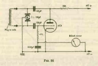
Circuits to be tested with a grid-dip meter do not need to have any RF present. Resonances in transmitter circuits, etc., can thus be checked with the equipment switched off. Aerial resonance may be checked by coupling the grid-dip meter to the aerial.
