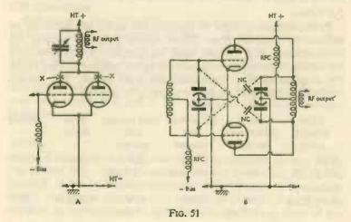
drive requirements will be twice those of a single valve, and anode, SG and heater currents will also be double those of one valve. The power input to the stage can be twice that for a single valve of the same type.
