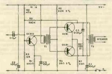
FIG. 98. Driver and push-pull output for 1 wattrto 1 watt
