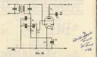
Fig. 26 shows a double-diode-triode providing detection and audio amplification. (The remaining diode is commonly used for AVC, described later.) Typical values are: V1 6AT6; C1 100pF; C2 100pF; C3  $0.01\mu$ F; C4  $25\mu$ F; C5  $0.05\mu$ F; R1 47K; R2 220K; R3 0.5 megohm volume control; R4 3K; R5 250K.
