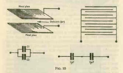
while in receivers for short waves only 100pF to 250pF will be more usual. The minimum capacity of these components is not zero, but will be around 5pF to 25pF or so. Mica capacitors are often up to about 1,000pF. Many paper capacitors are about 1,000pF to 1 $\mu$ F, while electrolytic capacitors are often 2 $\mu$ F to 100 $\mu$ F, and higher.
