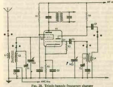
termed the 'padder'. Trimming is carried out as already described. At the low frequency end of the band, adjustment is generally by means of a screwed core, the padder being of fixed capacity. However, the oscillator coil could be of fixed inductance, the padder then being pre-set. Such a pre-set padder resembles an adjustable compression trimmer, except that it is normally of higher capacity.
