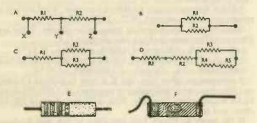
FIG. 6. Resistors in series and parallel, and resistor colour code
