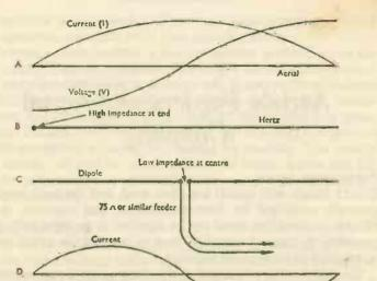
FIG. 70. Half-wave aerials A, B, and C. D is full-wave
