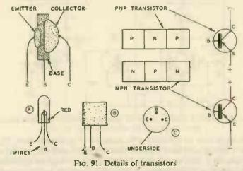
A transistor is a current amplifier and small changes in base current can cause large changes in collector current. Base and collector currents added form the emitter current. As example, with<sup>1</sup>a small transistor emitter current might be 2mA, collector current 1.9mA, and base current 0.1mA (100uA).
