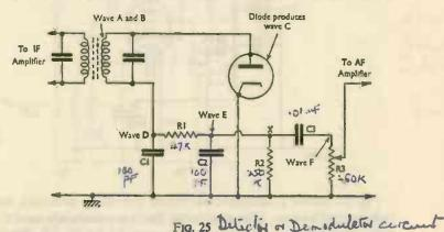
capacitor C2, which complete the RF filter, the wave resembles E. A capacitor C3 removes the DC voltage, which was obtained as a result of rectification, so that the audio signal resembles F, which was the original sound or audio wave used to modulate the transmitter. The signal could be heard if phones were connected across R3, but audio amplification normally follows to work a loudspeaker.
