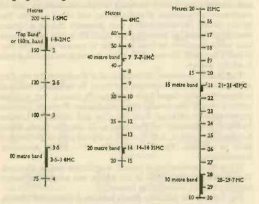
FIG. 1. Showing wavelengths with corresponding frequencies and Amateur Bands
