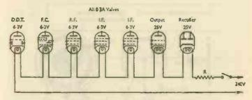
FIG. 7. Series heater circuit with mains dropper-
