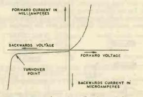
FIG. 90. Characteristics of a semiconductor diode
