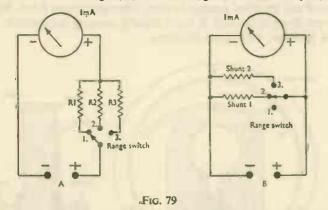
the total resistance needs to be 5,000 ohms. As the meter coil itself contributes 100 ohms, the external resistor is 4,900 ohms. For this correction, the meter resistance is taken from the total resistance.
