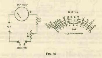
with the meter, the current will be reduced if an external resistor is added, so the meter scale can be arranged to read resistances in ohms. Fig. 80 shows a popular circuit for this purpose.
