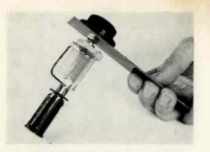
10. Above Absorption meter, as described in chapter on measurements. 11. Below Surplus type absorption meter, with plug in coils, verijer dial, and 250uA meter to show resonance.
