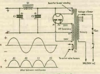
FIG. 67. Full wave rectifier circuit
