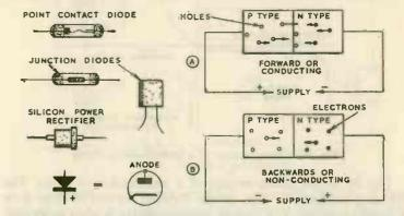
FIG. 89. Semiconductor diodes and polarity compared with thermionic diode
