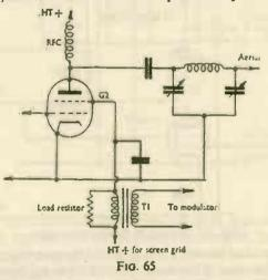
lator is added to that obtainable from the PA. Despite these limitations, grid modulation is extensively employed, in low-cost or small equipment.
