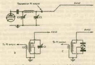
FIG. 74. Ways of connecting an end-fed aeria
