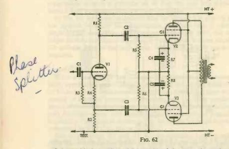
of phase with that at the cathode, and is of about equal magnitude, with a circuit like that in Fig. 62. R1 is the anode resistor, and R2 the cathode resistor, so that audio signals may be taken to the control grids G1, via C2 and C3. C1 provides coupling to an earlier stage, such as V1B in Fig. 60. R3 is the grid resistor, and R4 the bias resistor, of V1 in Fig. 62. R5 and R6 are grid resistors for V2 and V3, R7 and R8 providing cathode bias.
