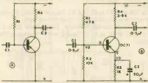
FIG. 93. Audio: amplifier for low signal levels
