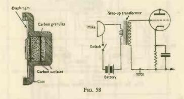
quality is less good than with the types previously described. To avoid a battery and transformer, the cathode current of a valve. may be passed through the mike, the control grid being earthed to chassis.
