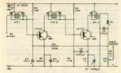
FIG. 96. 2-stage 470kc intermediate frequency amplifier
