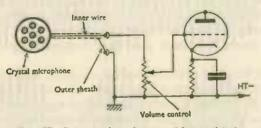
FIG. 57. Crystal microphone and input circuit
