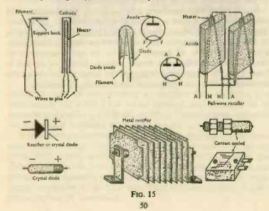
The heater may be operated from direct current or alternating current. Directly heated valves gain their working temperature almost instantly, while indirectly heated valves require some 15 to 30 seconds or more to do so. Indirectly heated valves are generally used in AC equipment, where AC on a filament would cause hum.
