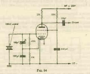
sensitivity of the receiver. Fig. 84 shows a typical circuit of this kind. Values for an EF39, 6K7, or similar value are shown, with a Quartz Crystal Co., Ltd., Q5/100 crystal.
