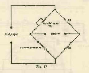
If the bridge were to be used for resistance measurements only, a battery or other source of DC could provide the bridge input, and a meter with central zero could be employed as the indicator.
