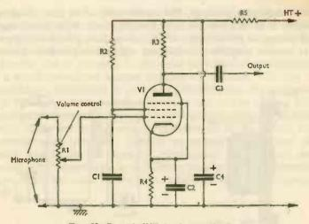
FIG. 59. Pre-amplifier or first audio stage
