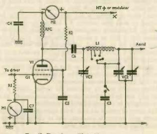
FIG. 49. Tetrode amplifier with  $\pi$  output
