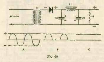
If a metal rectifier were employed, it would be connected in the polarity shown. Should a half-wave valve rectifier be used, rectifier anode is taken to the secondary of the mains transformer T1, and the cathode is taken to C1. That is, valve cathode corresponds to metal rectifier positive. In Fig. 66, a positive supply is obtained for HT circuits.
