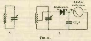
RF energy must be present in a circuit checked with an absorption meter. The absorption coil is placed near the RF coil being checked. When the absorption meter is tuned to the same frequency as the circuit being investigated, it absorbs some RF energy. With an oscillator, amplifier, or PA, this causes a rise in anode current.
