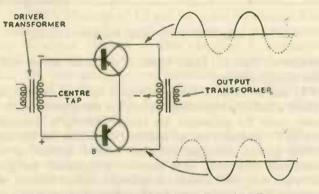
FIG. 97. Operation of transistors in push-pull
