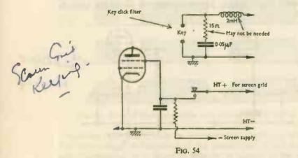
the control grid of the clamp valve is negative. The clamp valve thus passes little anode current, and the PA SG voltage is normal. In these circumstances, the PA is amplifying the RF applied to its control grid, and the transmitter is radiating.
