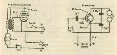
FIG. 3. Two oscillators suitable for Morse practice
