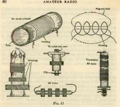
Interference suppressor chokes are also sometimes used in mains circuits, and these may also have to carry a fairly heavy current. Some typical RF chokes, with applications, are as follows:
