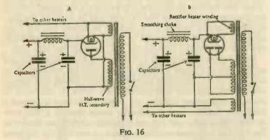
current of 48mA, and a maximum average rectified current of only 8mA. A fairly large rectifier valve for a small transmitter could have a peak current rating of 650mA, and an average rectified current rating of 250mA.
