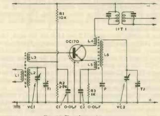
Fig. 95. Transistor mixer stage
