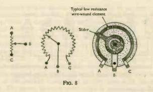
value as the spindle is rotated. Or it may be logarithmic, with a logarithmic variation in value. These components are termed 'linear' and 'log' potentiometers respectively.
