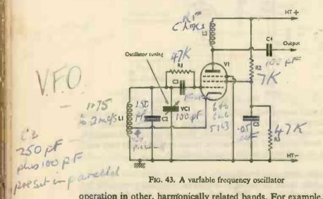
FIG. 43. A variable frequency oscillator
