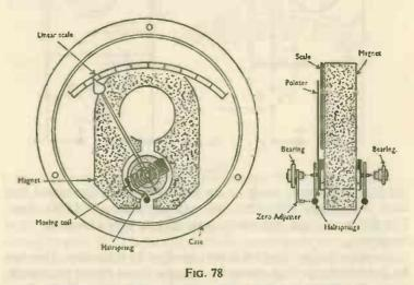
Such meters are used for DC only. Sensitivity depends on the number of turns on the coil, and other factors. A general purpose meter might be a 1mA movement. This means that a current of 1mA will move the pointer to the full-scale reading. Very sensitive meters have a full-scale reading of 0.1mA (100µA) or less. Meters with full-scale readings of 5mA, and over, are often used.
