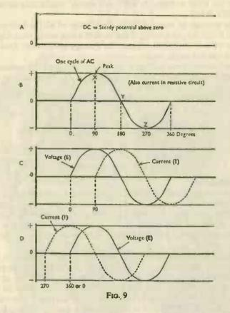
During a complete half-cycle, the voltage rises from zero, reaches maximum, and falls again to zero. The highest voltage reached is termed the 'peak' voltage.
