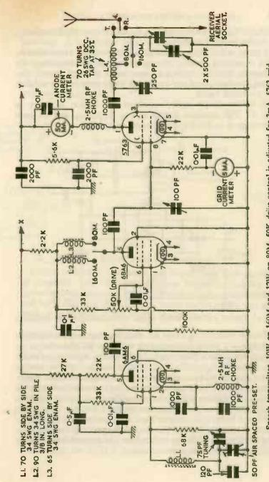
Speech transmitter. 10W on 160M and 12W on 80M. 50K drive control is adjusted for 3mA. 5763 grid current. L1, L2, and L3 wound on \$in diam. formers with cores. L4 1\$in diam. former 2\$in long. Transmitreceive switching is included here and in modulator, p 132.
