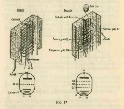
anode. If the grid is very negative, all current may cease. A steady negative voltage is usually applied to the grid, and is termed 'bias'. If the voltage is sufficiently negative to prevent current flowing, the valve is 'cut off'.
