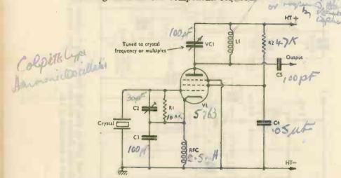
FIG. 41. Crystal oscillator giving output on fundamental and harmonics
