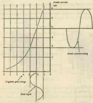
FIG. 18. Operation of class A amplifier
