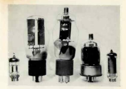
8. Above Receiver and transmitter valves: 1, B7G double triode; 2 5U4G full-wave rectifier; 3, 807 (top anode cap); 4, 6146 (top anode cap); 5, 6BW6 miniature output tetrode. 9. Below DX-40U 10 to 80 metre transmitter, 75 watts CW, 60 watts peak controlled carrier phone. (Heathkit Daystrom Ltd., Gloucester.)
