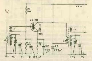
Fig.,94. Transistor radio frequency amplifier
