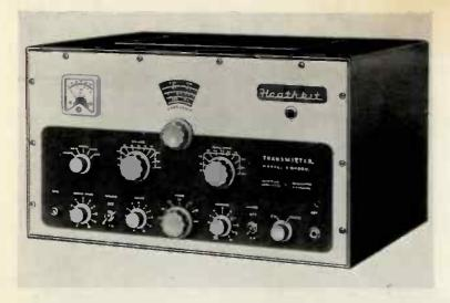
2. Above DX-IOOU table top transmitter, for speech and CW, 150 watts. 3. Below Morse practice outfit – transistor oscillator built to circuit in Chapter 1, and key.
