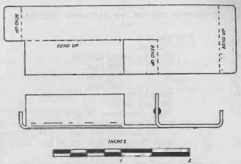
FIG. 10. THE COMPONENT BOARD (Proportions shown are for a "Fountain Pen" cell)
