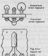
FIG. 1. A METHOD OF MOUNTING TRANSISTORS
