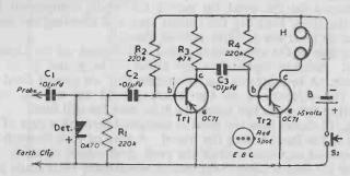
FIG. 12, THE SIGNAL TRACER
