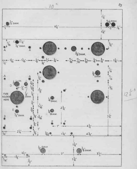
FIG. 21-THE A.C. MAINS SUPERHET, CHASSIS TOP VIEW
