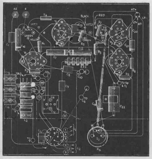
FIG. 19-UNDER-CHASSIS VIEW OF THE BATTERY SUPERHET TAG NO. 7 OF L2 IS EARTHED TO THE COIL'S FIXING BOLT
