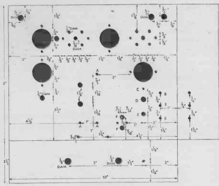
FIG. 18-THE BATTERY SUPERHET CHASSIS, TOP VIEW
