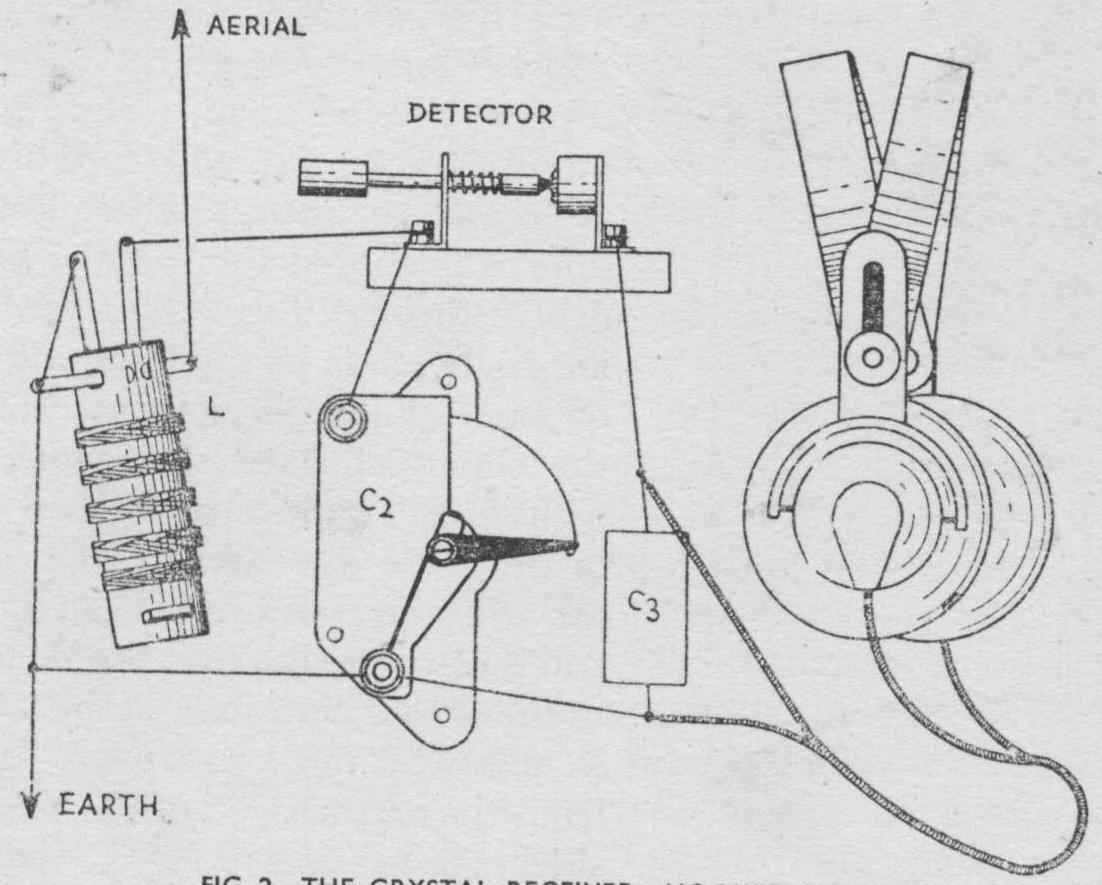
FIG. 2-THE CRYSTAL RECEIVER "HOOKED UP"
