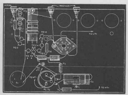
FIG. 8-UNDER-CHASSIS VIEW OF THE ONE-VALVE RECEIVER
