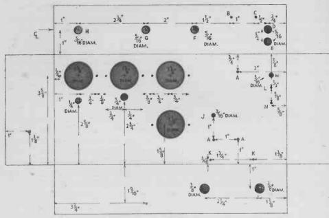
FIG. 7-TOP VIEW OF THE CHASSIS, SHOWING HOW TO DRILL IT
