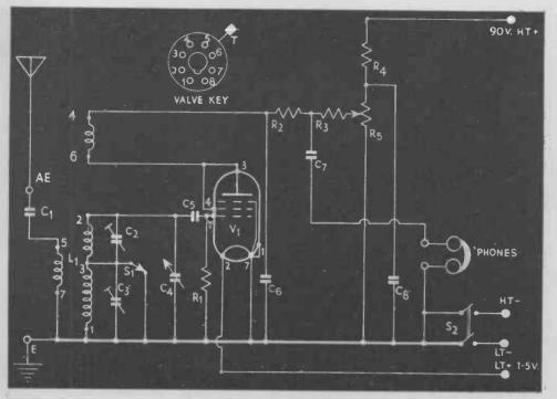
FIG. 6-THE ONE-VALVE RECEIVER
