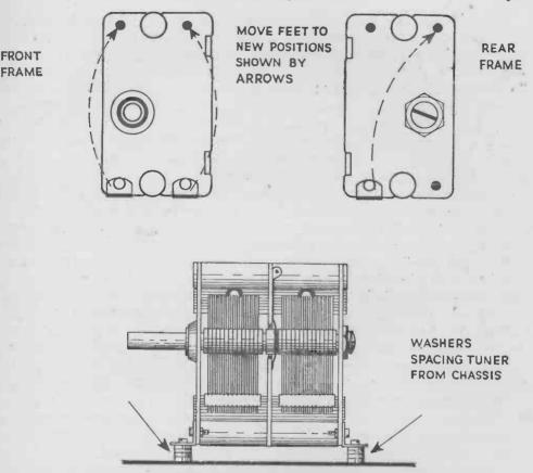
FIG. 9-MOUNTING THE TUNING CAPACITOR
