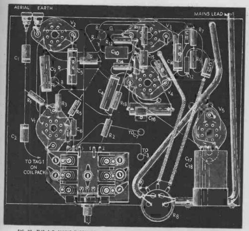
FIG. 22-THE A.C. MAINS SUPERHET, UNDER-CHASSIS VIEW, HEATER WIRING NOT SHOWN
