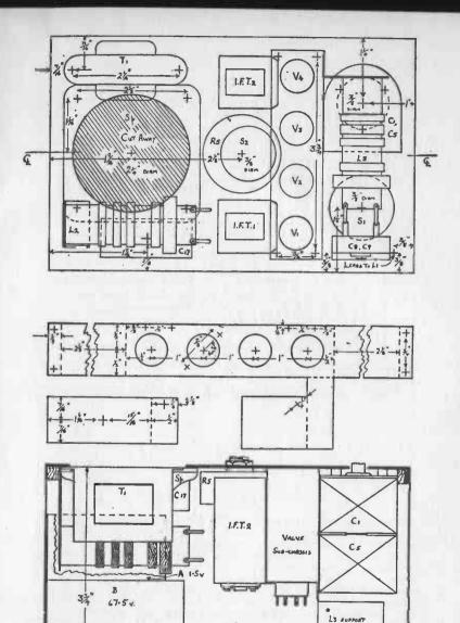
Fig. 12. Panel Dimensions, Bracket, Sub-Chassis and Side Constructional View of the "Two-Band Super" 29
