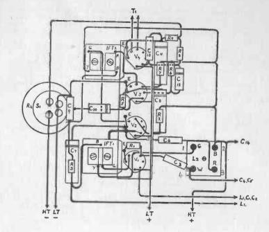
Fig. 10. Point-to-Point Wiring Plan of the "Simplest Super"
