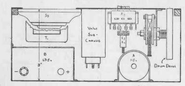
Fig. 2. Panel Dimensions, Sub-chassis and Side Constructional View of the "Minor"
