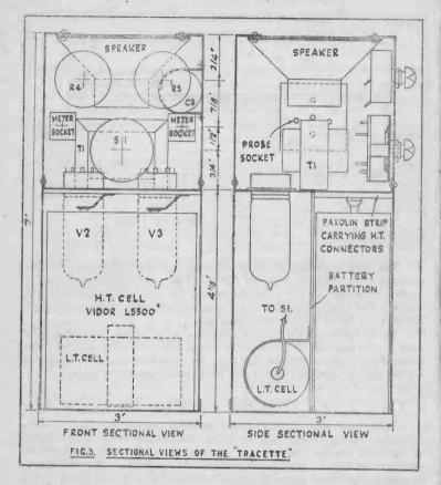
Generally speaking, however, it will be found that the  $2\frac{1}{2}$ " speaker, with its output transformer, can be fitted neatly into the case without trouble.
