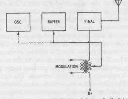
Fig. 6-7. Preferred method of modulating both driving and final stages.
