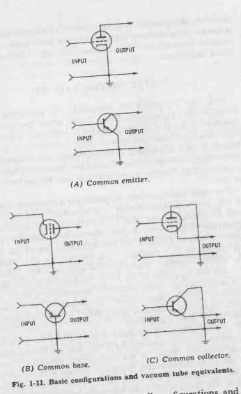
Actually the  $f_{max}$  is the same for all configurations and the actual circuit used would seem to be a matter of choice. However, there are subtle differences which are not immediately obvious. If the frequency of operation is such that the transistor is operating on the flat-gain portion of the frequency-response curve, the common-emitter configuration should be employed for the many reasons just described. However, the
