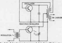
Fig. 6-1. A basic reactance-modulated oscillator circuit. Bias and voltage omitted for simplicity.
