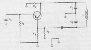
Fig. 2-12. Alternate Colpitts circuit.
