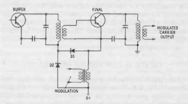
Fig. 6-8. "Trick circuit" for increasing positive peak modulation.
