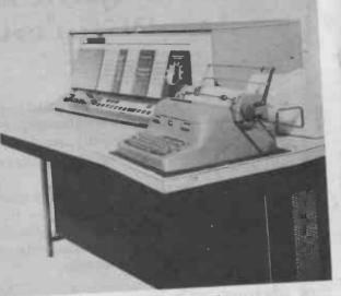
Fig. 1-1. Transistor IBM 1620 computer.
