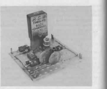
Fig. 3-4. Photo showing crystal socket.
