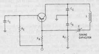
Fig. 2-14. Clapp oscillator configuration.
