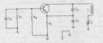
Fig. 2-15. Alternate Clapp oscillator circuit.
