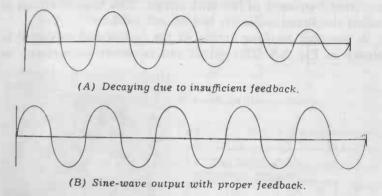
Fig. 2-5. Damped-wave oscillator output.
