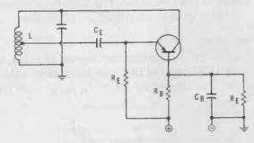
Fig. 2-9. Common-base Hartley oscillator.
