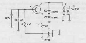
Fig. 3-8. Schematic diagram of the "CB Cyclone."
