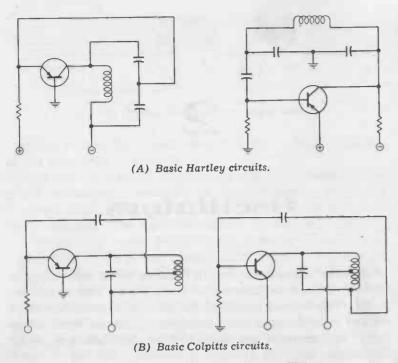
Fig. 2-2. Hartley- and Colpitts-type oscillators.
