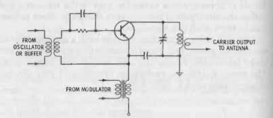
Fig. 6-5. Output circuit of a typical AM transistor transmitter.
