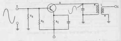
Fig. 2-4. PNP RF-amplifier circuit.
