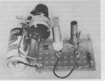
Fig. 7-7. The tunnel-diode transmitter.
