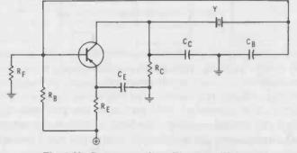
Fig. 2-23. Common-emitter Pierce oscillator.
