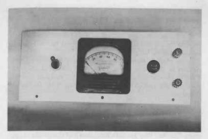
Fig. 1-13. Inexpensive bench voltage source.
