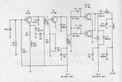
Fig. 8-1. Circuit of high-power CB and 10-meter transmitter.
