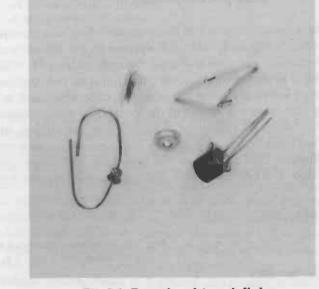
Fig. 7-1. Examples of tunnel diodes.
