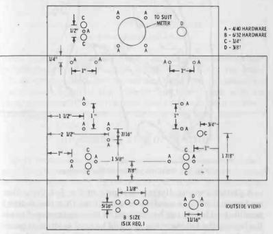
Fig. 5-3. Chassis layout for Novice Powerhouse transmitter.
