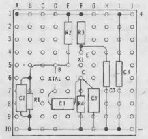
Fig. 3-3. Layout of the crystal checker.
