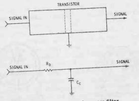
Fig. 1-6.  $\mathbf{R}_{b}$  and  $\mathbf{C}_{c}$  form low-pass filter.
