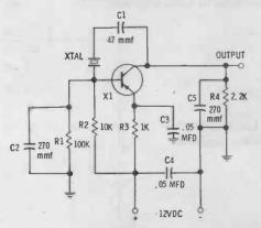
Fig. 3-2. Schematic of the crystal checker.
