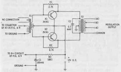
Fig. 6-15. Schematic diagram of the five-watt transmitter modulator.
