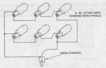
Fig. 5-6. Dummy-load bank for transmitter testing.
