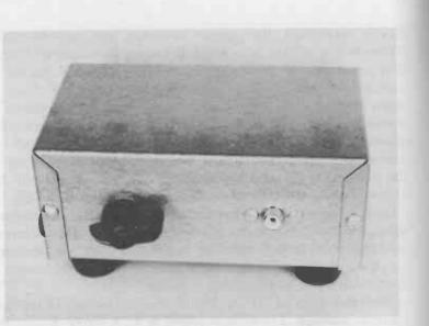
Fig 6-14. Top view of finished half-watt modulator.
