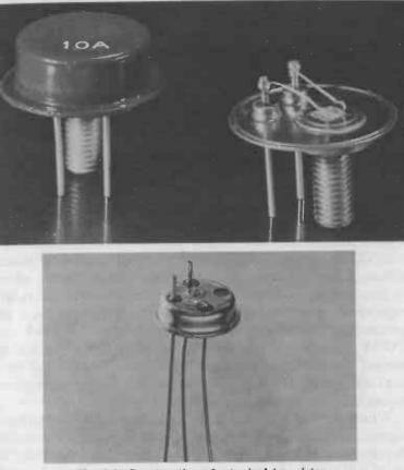
Fig. 1-3. Construction of a typical transistor.
