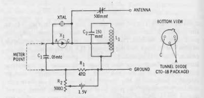
Fig. 7-5. The tunnel-diode oscillator.
