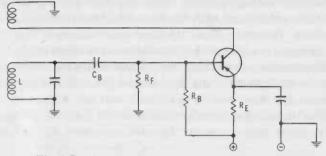
Fig. 2-7. Alternate tickler-coil oscillator circuit.
