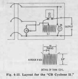
the output of the oscillator board passes between the collector and emitter pins. A  $\frac{1}{4}$ " hole was drilled at G-3 to mount the trimmer capacitor used to resonate the final tuned circuit. A peg for the output connector was installed at J-5. The coil is attached between the tuning capacitor C1 and the bypass capacitor C2, and is supported by its own leads. The finished transmitter is shown in Fig. 4-13.
