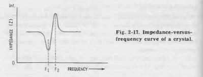
resonance. Note the steep slope between the two points; this indicates that it is a very high-Q tuned circuit.
