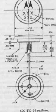
Fig. 1-5. Typical transistor cases.
