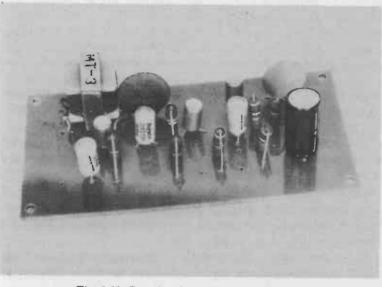
Fig. 6-11. Completed low-power modulator.
