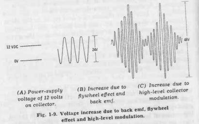
and any one of these peaks can have sufficient duration to cause instantaneous destruction of the transistor.
