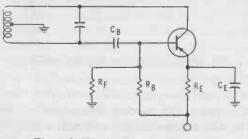
Fig. 2-8. Hartley-type oscillator.
