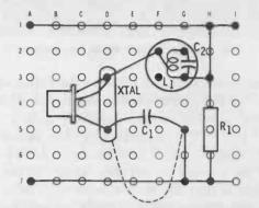
Fig. 7-6. Layout of the tunnel-diode oscillator.
