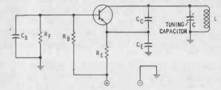
Fig. 2-13. Colpitts with tuning capacitor.
