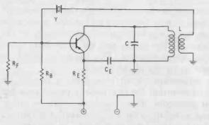
Fig. 2-18. Crystal-controlled version of a tickler-coil oscillator.
