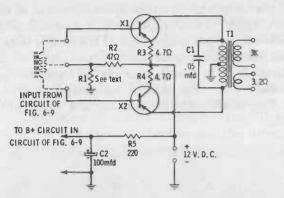
Fig. 6-12. Schematic of the half-watt modulator.
