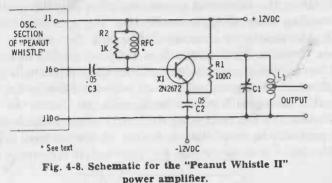
10 times (10 db). The final tank circuit is designed to tune all frequencies between 3 and 10 mc. The power output, approximately .25 watt, is sufficient to dimly light a No. 47 pilot lamp or brightly light a No. 49 lamp.
