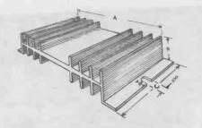
Fig. 1-4. Commercially built heat sink.
