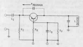
Fig. 2-10. Colpitts oscillator circuit.
