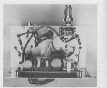
Fig. 6-17. Internal view of 5-watt modulator.
