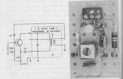
Fig. 2-6. Practical circuit of a tickler-coil oscillator.
