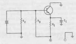
Fig. 2-24. Unusual transistor oscillator circuit.
