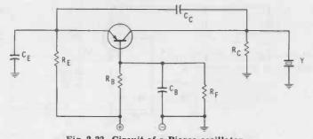
Fig. 2-22. Circuit of a Pierce oscillator.
