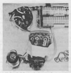
Fig. 1-16. Practical dummy-load system for transmitters.
