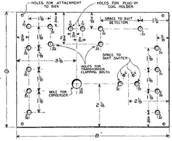
Fig. 121.—Lay-out of Panel.
