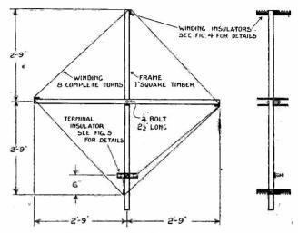
Fig. 32.—Front and Side Elevations of Frame.
