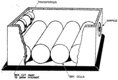
Fig. 140.—-Arrangement of Components Inside Box.
