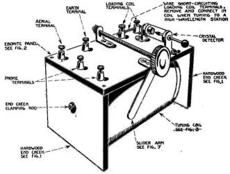
Fig. 99.—Completed Receiver.
