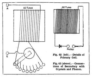
Mounting the Parts.—The switch and detector are mounted on an ebonite panel  $4\frac{1}{2}$  in. by  $5\frac{3}{4}$  in. The two coils are kept central one within the other by means of  $\frac{1}{4}$ -in. wood discs fitting tightly in the ends of each cylinder.
