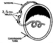
Fig. 69.-Method of Securing Ends of Winding.
