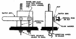
Fig. 93.—Details of Shorting Switch.
