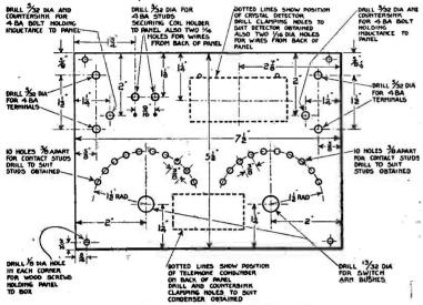
Fig. 86.—Drilling Lay-out of Panel.
