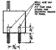
Fig. 84. Method of Securing Coil-Holder to Panel.
