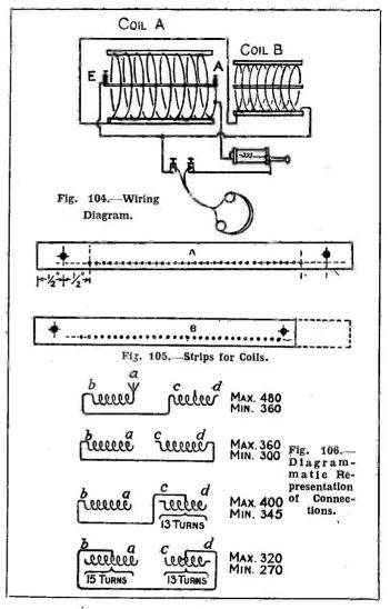
the positions of the holes being as shown in Fig. 105. Strips a are for the outer or large coil and strips B for the inner or smaller coil. All five of the strips may be bored simultaneously by screwing them together. This being done, the bare or enamelled covered wire is prepared for winding in the following manner.
