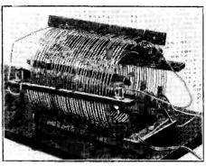
Fig. 102.—Another View of Air-spaced Loose-coupled-Set.
