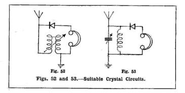
Connections.—The set is connected in the usual manner, as shown in the diagrams (Figs. 52 and 53), the connections being made with bell wire. In order to get good results from a crystal set, it is necessary to insulate every part with ebonite, and also to keep the crystal free from dust. It can be kept clean by putting a thimble over the cup.
