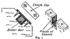
Fig. 1. - Method of Insulating Slider-bar.
