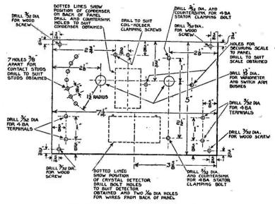
Fig. 66.—Drilling Lay-out of Panel.
