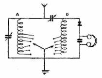
Fig. 39.—Highly-selective Crystal Circuit.
