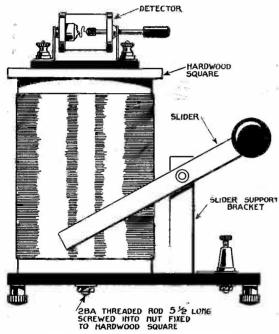
Fig. 27.—Front Elevation of Receiver.
