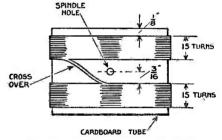
Fig. 70.—Winding Details of Rotor.
