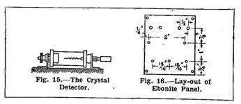
holes in the top are for the earth, aerial and telephone respectively, the centre ones for the detector and the bottom for the variometer. When this has been completed the set may be assembled.
