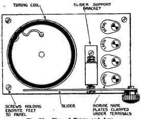
Fig. 28.—Plan of Tuner and Arm.
