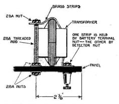
Fig. 126.—Method of Mounting Transformer.
