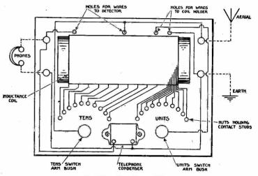
Fig. 90.—Coil Connections,
