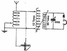
Fig. 38.—Circuit Diagram of "Loud" Crystal Set.
