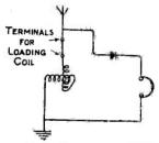
Fig. 6.—Circuit Diagram of Variometer Receiver.
