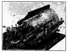
Fig. 101. View of Air-spaced Loose-coupled-Set.
