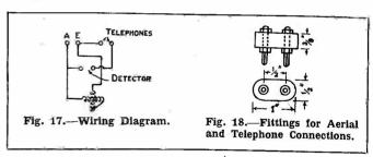
Fixing the Variometer.—The variometer is fastened to the top with the screws provided and the handle knob screwed on. The detector is then fixed down with 5 B.A. screws. The plugs for the outside connections are lightly tapped in with a hammer: on
