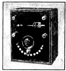
Fig. 40.—The Complete Fixed-Coupled Receiver.
