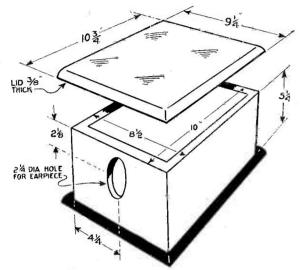
Fig. 134.—Details of Containing Box and Lid.
