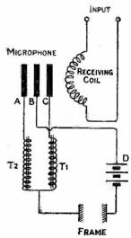
Fig. 55.—Circuit Diagram of "Crystavox."
