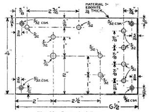
Fig. 20.-Lay-out of Base.
