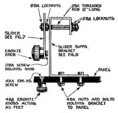
Fig. 26.—Assembly of Slider and Support.
