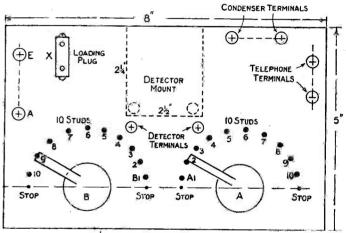
Fig. 47.—Lay-out of Ebonite Panel.
