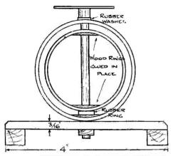
Fig. 9.—Arrangement of Variometer Formers.
