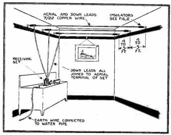
Fig. 19.—Arrangement of Receiver and Indoor Aerial.
