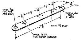
Fig. 135.—Brass Strip for Earpiece Clip.
