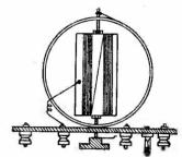
Fig. 4a.—Section of Complete Variometer.
