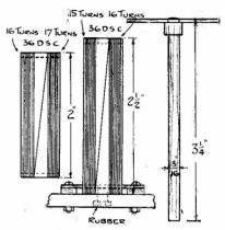
Fig. 8.—Details of Windings and Spindle,
