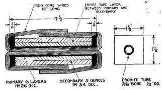
Fig. 124.—Section and Detail of Transformer.
