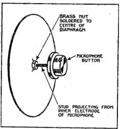
Fig. 410.—Microphone Attached to Earpiece Diaphragm. This arrangement is inferior to that shown by Fig. 114.
