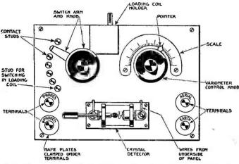
Fig. 74.—Plan View of Panel showing Position of Components.
