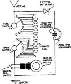
Fig. 91.—Diagram of Connections.
