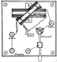
Fig. 9b.—Plan of Complete Receiver.
