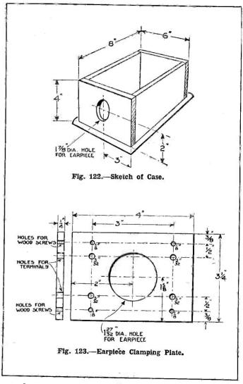
latter should be pushed into the large hole in the ebonite clamping plate (Fig. 123) and four terminals fixed in position in the  $\frac{5}{32}$ -in. diameter holes.
