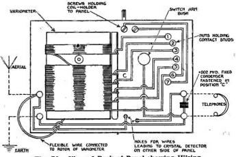
Fig. 76. View of Back of Panel showing Wiring.
