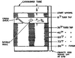
Fig. 72.—Winding Details of Rotor.
