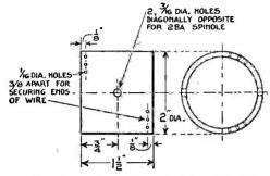
Fig. 67.—Drilling Details of Rotor Tube.
