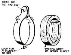
Fig. 136.—Earpiece Clip and Rubber Packing,
