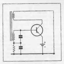
FIG. 40. JUNCTION TRANSISTOR L.F. OSCILLATOR.
