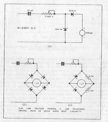
FIG. 18(a). SOME A.C. METER CIRCUITS. FOR LOW VOLTAGE RANGES A LOW RESISTANCE CRYSTAL (SUCH AS GEX 64) GIVES BEST LINEARITY.
