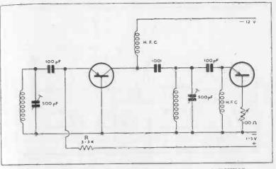
FIG. 26. H.F. STAGE WITH ALTERNATIVE FORM OF MATCHING.
