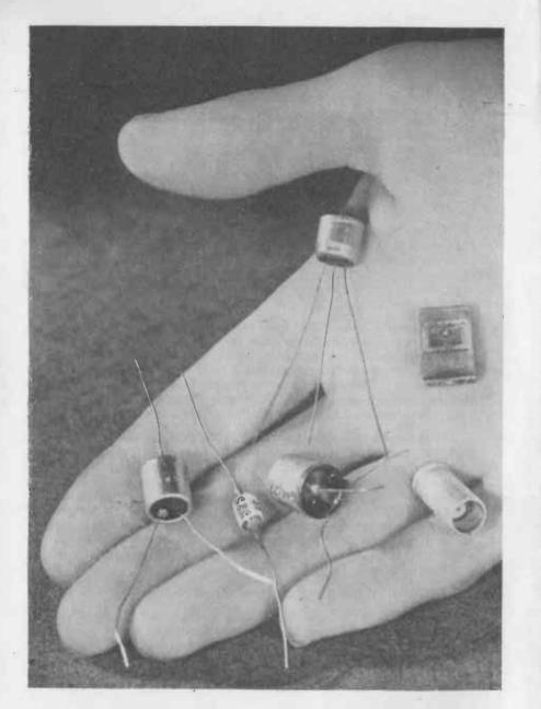
(By courtesy The General Electric Co. Ltd.) A SELECTION OF SEMI-CONDUCTOR DEVICES HELD TO ILLUSTRATE THEIR SMALL SIZE.
