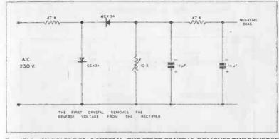
FIG. 17(a). VARIABLE BIAS SUPPLY. THE FIRST CRYSTAL REMOVES THE REVERSE VOLTAGE FROM THE RECTIFIER.
