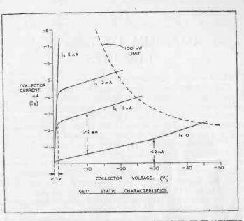
FIG. 9. COLLECTOR-CURRENT CURVES OF POINT-CONTACT TRANSISTOR.
