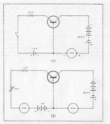
FIG. 43(a). CIRCUIT FOR ROUGH CHECK OF JUNCTION OR POINT-CONTACT TRANSISTORS.
