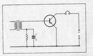
FIG. 36. BIAS ARRANGEMENT TO GIVE IC GREATER THAN Ic.
