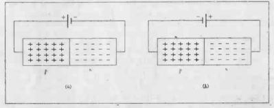
FIG. 1. JUNCTION, TRANSISTOR CONNECTED AT (a) FOR EASY CURRENT FLOW AND (b) FOR SMALL REVERSE CURRENT
