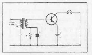
FIG. 35. TRANSFORMER COUPLED AMPLIFIER.
