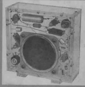
A transistor receiver using two transistors in a reflex circuit. Its total current consumption is 6mA at 18V.
