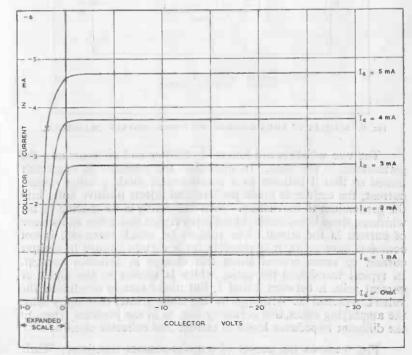
FIG. 7. COLLECTOR-CURRENT CURVES OF A TYPICAL *p-n-p* JUNCTION TRANSISTOR OF  $\infty = .95$  APPROX.
