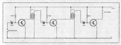
FIG. 38. FUNDAMENTAL CIRCUIT OF HEARING AID AMPLIFIER.
