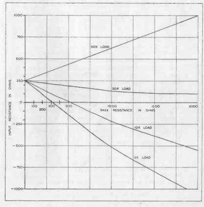
FIG. 45. CURVE SHOWING VARIATION OF INPUT RESISTANCE WITH BASE RESISTANCE.
