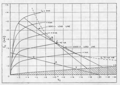
FIG. 19. CURVES OF POINT-CONTACT TRANSISTOR TYPE GET2 WITH LOAD LINES. SHADED PORTION CANNOT BE USED.
