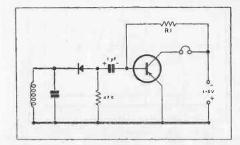
Fig. 34. L.F. JUNCTION AMPLIFIER FOLLOWING CRYSTAL RECEIVER.
