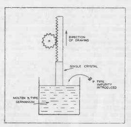
FIG. 2. MAKING A GROWN JUNCTION.
