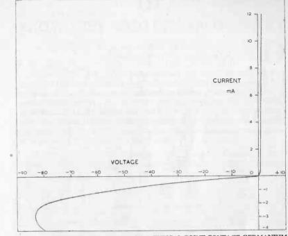
FIG. 5. CHARACTERISTIC CURVE OF A TYPICAL POINT-CONTACT GERMANIUM DIODE.
