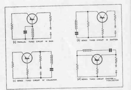
FIG. 29. FOUR POSSIBLE SINE WAVE CIRCUITS.
