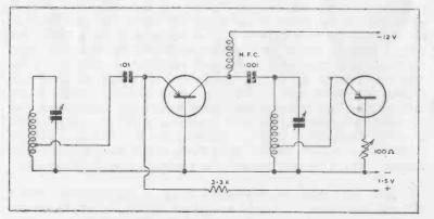
FIG. 25. POINT-CONTACT TRANSISTOR H.F. STAGE.
