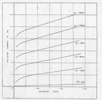
FIG. 32. COLLECTOR-CURRENT CURVES OF A TYPICAL *p-n-p* JUNCTION TRANSISTOR IN EARTHED-EMITTER CONNECTION.
