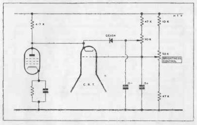
FIG. 12. TV SPOT LIMITER IN ANODE CIRCUIT OF VIDEO VALVE.
