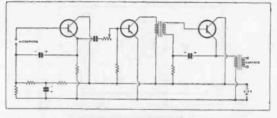
FIG. 39. CIRCUIT OF COMMERCIAL HEARING AID.
