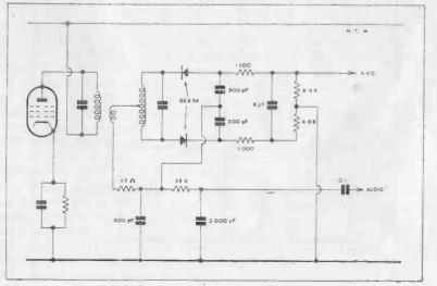
FIG. 17. RATIO DETECTOR USING CRYSTAL DIODES.
