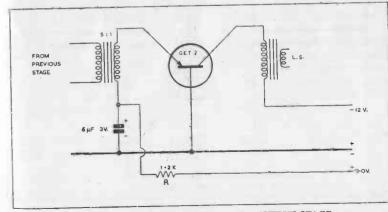
FIG. 20. POINT-CONTACT TRANSISTOR OUTPUT STAGE.
