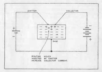
FIG. 8. SCHEMATIC ARRANGEMENT OF POINT-CONTACT TRANSISTOR.
