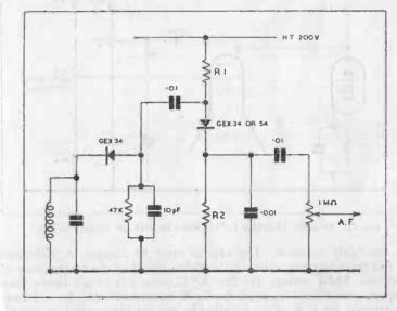
FIG. 11. TV SOUND DETECTION AND LIMITING.
