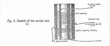
4 turns of 26 s.w.g. wire are used, this winding being about  $\frac{1}{8}$  in. from the grid winding, as in Fig. 2. The ends of both windings are joined, as indicated, this lead going to the receiver chassis.
