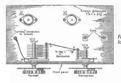
Fig. 20. The simple layout of components.
