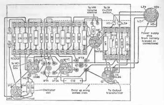
Fig. 54. Underchassis wiring extra to the group board wiring,
