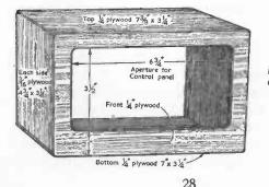
Fig. 15. Construction of a suitable cabinet for the receiver.
