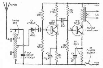
Fig. 7. The two-transistor circuit.
