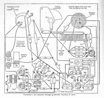
Fig. 46. Complete wiring diagram and connections between control panel and chassis.
