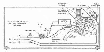
Fig. 13. Underchassis wiring. As an alternative arrangement, S1 and S2 could be mounted on the side of the cabinet.
