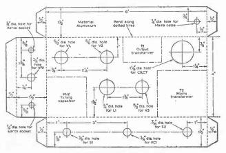
Fig. 17. Dimensions of the chassis.
