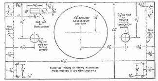
Fig. 52. Dimensions of the front panel.
