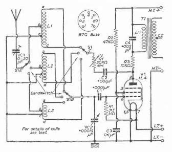
Fig. 23. The circuit of the detector stage.
