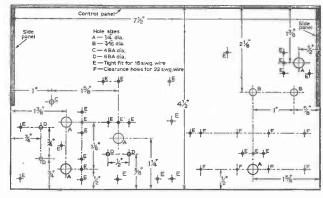
Fig. 45. Dimensions of the chassis.
