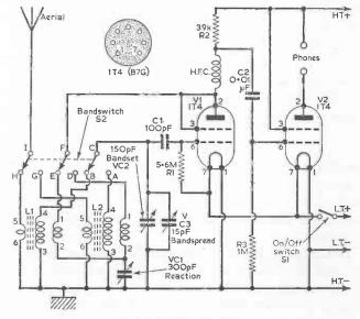
Fig. 19. The circuit. 37 batteries, the zinc case is negative. Cells must not be wired in series, nor must more than  $1\frac{1}{2}V$  be used. The filament consumption is only 0.1A.
