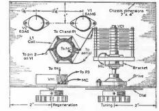
Further details of the tuning drive will be seen in Fig. 5. The dial is just clear of the panel. Some form of reduction drive is essential and a small ball-drive of this kind is easy to fit. The projecting lug on the drive must be prevented from rotating, and this is arranged by passing a bolt through the panel, as in Figs. 3 and 5. A slotted bracket will allow the tuning capacitor to be mounted at the correct height, so that the whole turns smoothly.
