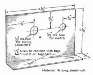
Fig. 32. Details of the panel which carries the tuning capacitor and wave-change switch, and which is bolted to the component tag board.
