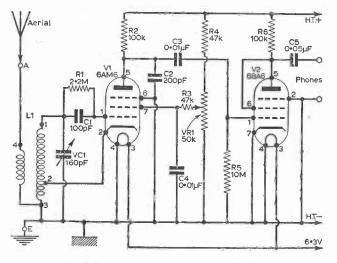
Fig. 1. The receiver circuit less power supplies.
