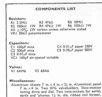
2<sup>1</sup>/<sub>2</sub> in. long, with chassis socket if plug-in type (Eddystone). Small, insulated tag strip. Bracket for VCI. Two knobs. Tinned copper wire for coils. Connecting wire, nuts, bolts, etc.
