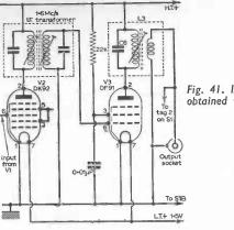
Fig. 41. Increased output may be obtained with this circuit modification.
