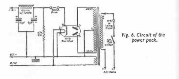
Current is drawn from a 3-pin plug, and the chassis of the receiver is earthed. If this earthing is effective, and a 500mA or other low-rating fuse is included in the mains circuit as in Fig. 5, mains voltages cannot be present at the receiver, even if the mains transformer were faulty.
