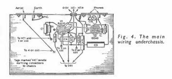
A single tag, on a small tag strip, and insulated from the chassis, forms the h.t. positive junction point, for R2, R4 and R6. The three power supply leads emerge through a grommet in the rear runner, and should be identified to make sure there is no error in connecting the receiver to its power pack. A lead from the chassis forms the h.t. negative
