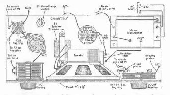
Fig. 12. Chassis and panel dimensions, layout and wiring above chassis.
