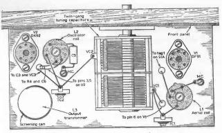
Fig. 39. Chassis component layout.
