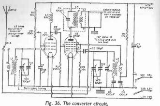
across L3 which is tuned precisely to this frequency. To enable a suitable match to be made to the aerial coil of the subsequent receiver with which the converter is used, the low impedance winding associated with L3 is employed and the coil is in fact a standard medium wave coil used in reverse.
