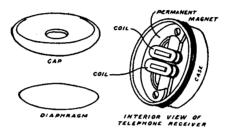
FIG. 64.—Showing construction of a "watch case" telephone receiver.
