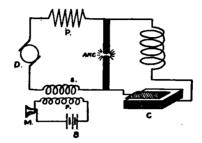
FIG. 145.—Arrangement of the speaking arc.
