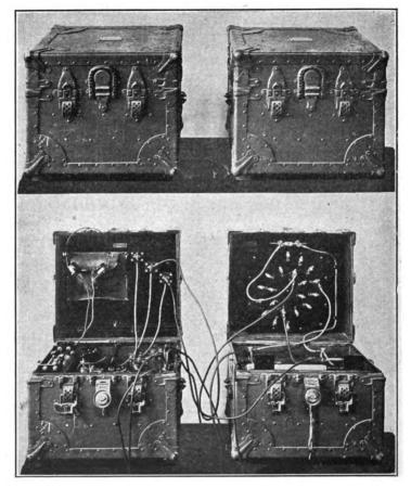
FIG. 108.—U. S. Signal Corps pack sets shown open and closed. Receiving apparatus on the left.
