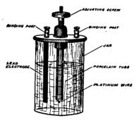
FIG. 38.—Electrolytic interrupter.
