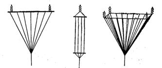
FIG. 15.—Vertical aerials of the "grid," "fan" and "inverted pyramid" types.
