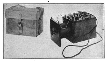
FIG. 60.—Portable receiving set and case.
