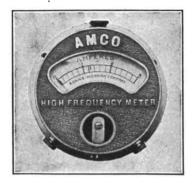
FIG. 88.—Hot-wire ammeter.
