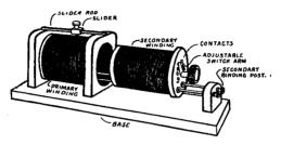
FIG. 91.-Loose coupled tuning coil.
