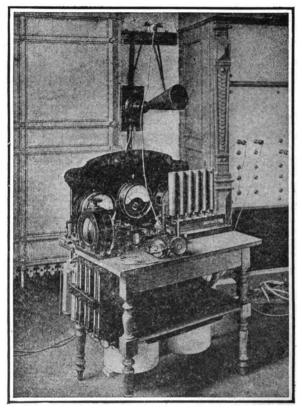
FIG. 147.-Poulsen wireless telephone equipment.
