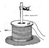
FIG. 30—If a magnet is suddenly plunged into a hollow coil of wire a momentary electric current will be induced in the coil.
