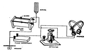
FIG. 79.—Diagram showing fixed condenser in circuit.
