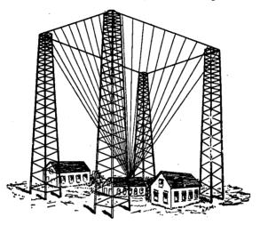
FIG. 16.-A diagram showing pyramid aerial.
