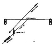
FIG. 89.—The principle of the hot-wire ammeter.
