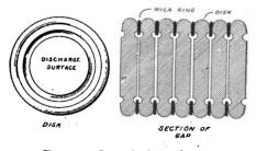
FIG. 53.-Quenched spark gap.
