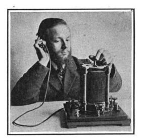
FIG. 97.—Bellini-Tosi radio-goniometer for directive wireless telegraphy.
