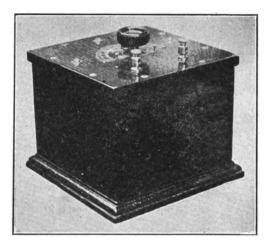
FIG. 81.-Rotary variable condenser.
