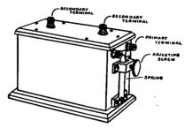
FIG. 35.-Induction coil for wireless telegraph purposes.
