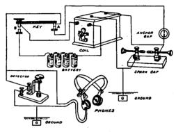
FIG. 118.-Breaking-in system.
