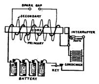
FIG. 34.-Diagram of induction coil.
