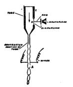
FIG. 148.—The Majorana wireless telephone transmitter.
