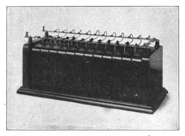
FIG. 95.-Transmitting condenser (molded dielectric).
