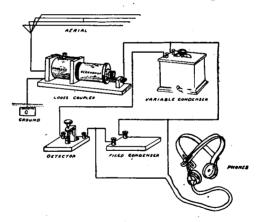
FIG. 85.—Diagram showing arrangement of rotary variable condenser in receiving circuit.
