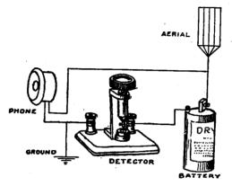
FIG. 73.-Electrolytic detector in circuit.
