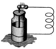
FIG. 4.—A Leyden jar discharging through a coil of wire produces a brilliant spark and high frequency oscillations are created.
