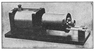
FIG. 92.-Loose coupled tuner.
