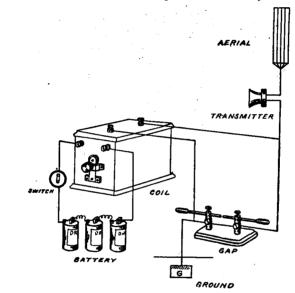
FIG. 139.—A "logical" form of wireless telephone which is impracticable.
