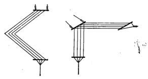
FIG. 18.—Aerials of the "V" and inverted "L" types.
