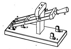
FIG. 54.—Diagram of aerial switch.
