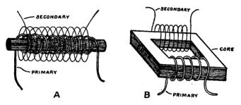
FIG. 39.—Open and closed core transformers.
