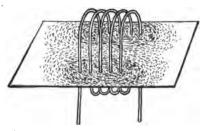
FIG. 33.-Magnetic phantom formed by coil of wire carrying current.
