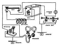
FIG. 118.—Breaking-in system.
