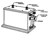
FIG. 35.—Induction coil for wireless telegraph purposes.
