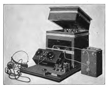
FIG. 109.—The receiving apparatus of the airship "America" (Wellman expedition).
