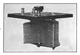
FIG. 82.-Interior of rotary variable condenser showing construction.
