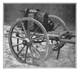
FIG. 101.—Telefunken wireless cart, showing transmitter.
