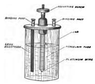
FIG. 38.—Electrolytic interrupter.
