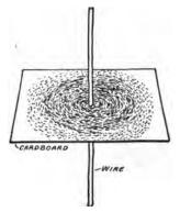
FIG. 32.-Magnetic phantom formed by wire carrying current.
