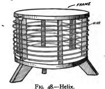
THE HELIX is an instrument consisting of copper or brass wire wound around a frame of hard rubber or sea-
