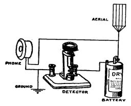
FIG. 73.-Electrolytic detector in circuit.
