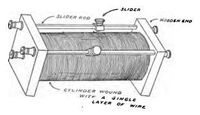
FIG. 78.—Tuning coil of the double slide type.
