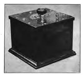
FIG. 81.-Rotary variable condenser.
