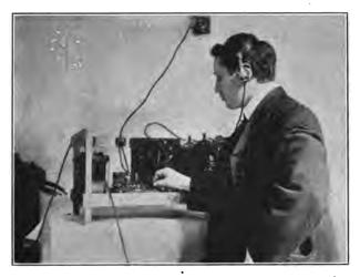
FIG. III.—Operating the U. S. Signal Corps airship wireless apparatus.
