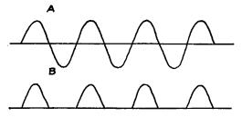
FIG. 66.-Illustrating the valve action of a rectifying detector.
