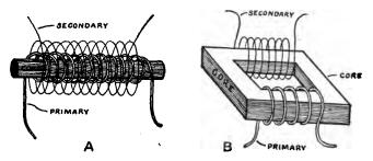
FIG. 39.—Open and closed core transformers.
