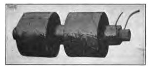
FIG. 36.-Induction coil, primary and secondary.
