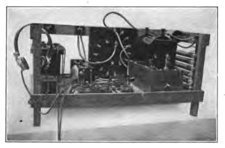
FIG. 100.—Special light weight wireless telegraph set for airship service.
