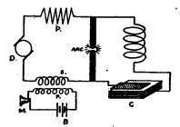
FIG. 145.-Arrangement of the speaking arc.
