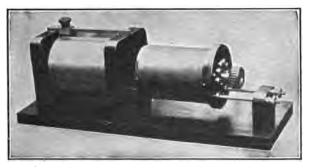
FIG. 92.-Loose coupled tuner.
