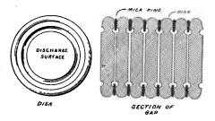
FIG. 53.—Quenched spark gap.
