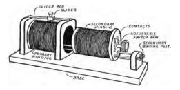
FIG. 91.-Loose coupled tuning coil.
