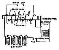
FIG. 34.-Diagram of induction coil.
