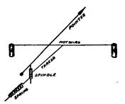
FIG. 89.—The principle of the hot-wire ammeter.
