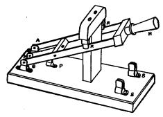
FIG. 54-Diagram of aerial switch.
