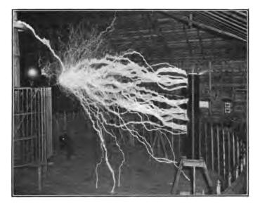
FIG. 156.—Twenty-five foot sparks from a Tesla transformer.
