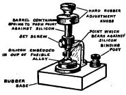
FIG. 71.—Silicon detector.
