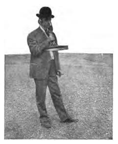
FIG. 141.—Wireless telephone receiving apparatus (induction method).
