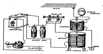
FIG. 90.-Diagram showing loose coupled helix in circuit.
