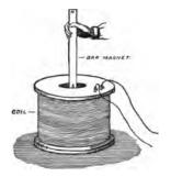
FIG. 30.—If a magnet is suddenly plunged into a hollow coil of wire a momentary electric current will be induced in the coil.
