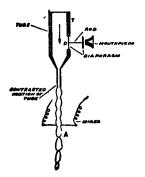
FIG. 148.—The Majorana wireless telephone transmitter.
