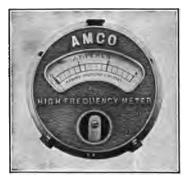
FIG. 88.—Hot-wire ammeter.
