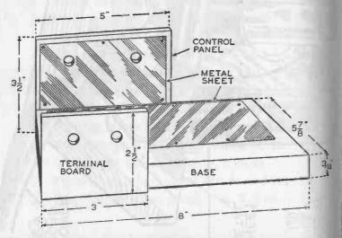
THE CHASSIS UPON WHICH THE COMPONENTS OF THE AMPLIFIER ARE MOUNTED
