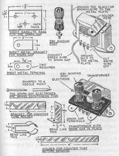
DETAILS OF THE SPARK GAP, BRACKET AND HOLDER FOR G-M TUBE
