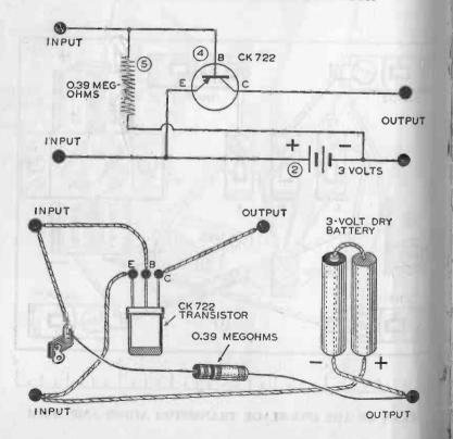
The components can be purchased for \$1.75 or less. When connected to either of the crystal detector receivers described in Chapter Three, this amplifier will greatly increase the strength of the signals.
