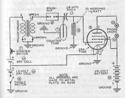
SCHEMATIC CIRCUIT DIAGRAM OF THE "GAMMA SNIFFER"
