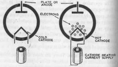
RADIO TUBES ARE ABLE TO FUNCTION BECAUSE OF ELECTRON EMISSION FROM A HEATED FILAMENT
