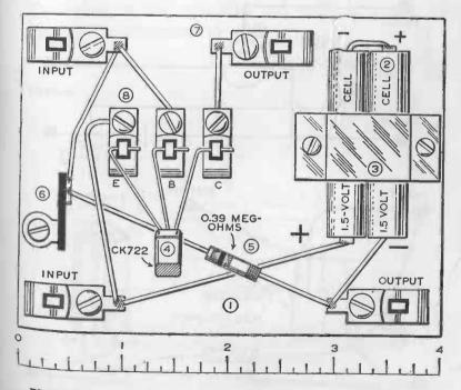
PLAN OF THE ONE-STAGE TRANSISTOR AUDIO AMPLIFIER
