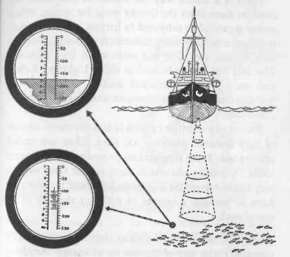
HOW THE EDO FISHSCOPE OPERATES
