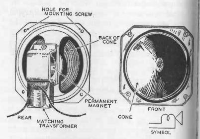
FRONT AND BACK OF A SMALL PM LOUDSPEAKER WITH TRANSFORMER
