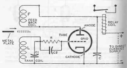
CIRCUIT OF CAPACITY RELAY USED TO STOP AND LEVEL ELEVATORS
