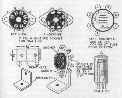
THE 3S4 AMPLIFIER TUBE, ITS SOCKET AND BRACKET FOR MOUNTING THE SOCKET ON CHASSIS
