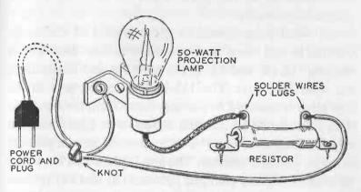
CONNECT LAMP IN SERIES WITH RESISTOR
