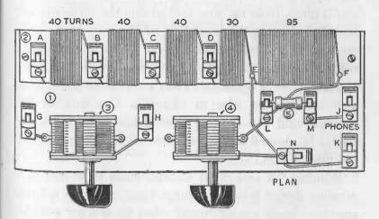
PLAN OF THE CRYSTAL RECEIVER AND DETAILS OF THE TUNING INDUCTANCE
