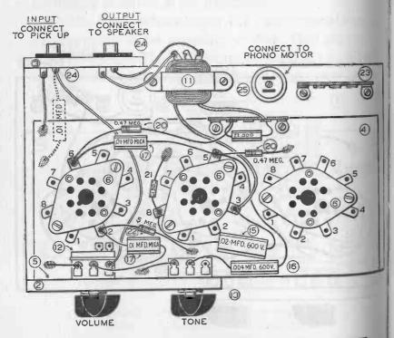
PLAN OF THE AMPLIFIER SHOWING THE WIRING OF THE AUDIO CIRCUIT
