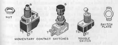
SWITCHES OF THE TYPES USED IN BUILDING THE SNIFFER
