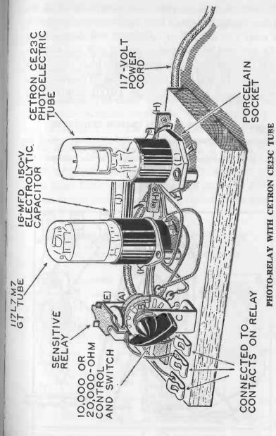
The letters enclosed in parentheses are the keys for identifying the parts with those in the plan.
