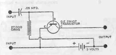
SCHEMATIC CIRCUIT DIAGRAM OF ONE-STAGE AUDIO AMPLIFIER EMPLOYING G. E. 2N107 TRANSISTOR
