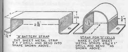
HOMEMADE CLAMPS FOR SECURING THE BATTERIES TO THE CHASSIS
