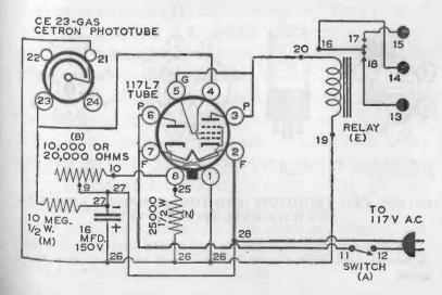
117L7 tube operates directly from the 117-v AC power supply without any form of resistor in series.
