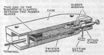
THE CARTRIDGE IN A PHONOGRAPH PICKUP IS A TINY ELECTRICAL GENERATOR
