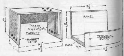
CABINET AND CHASSIS FOR AN ENCLOSED MODEL OF THE AMPLIFIER
