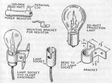
PROJECTION LAMP, SOCKET, RESISTOR AND HOMEMADE BRACKET FOR LIGHT SOURCE
