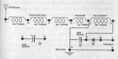
CIRCUIT DIAGRAM OF THE CRYSTAL RECEIVER
