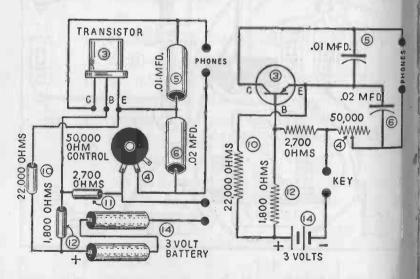
PICTORIAL AND SCHEMATIC CIRCUITS OF THE CODE PRACTICE OSCILLATOR
