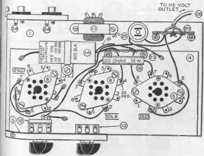
PLAN OF THE AMPLIFIER SHOWING THE POWER WIRING TO THE TUBE HEATERS AND PLATES
