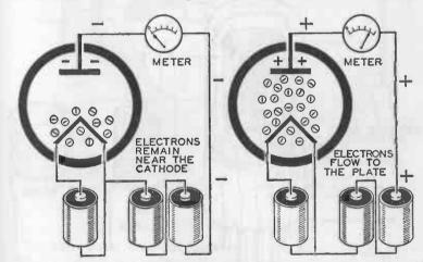
THE FUNDAMENTAL ACTION WHICH OCCURS IN A RADIO TUBE
