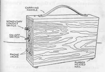
"GAMMA SNIFFER" OR HOMEMADE GEIGER COUNTER FOR DETECTING URANIUM ORES
