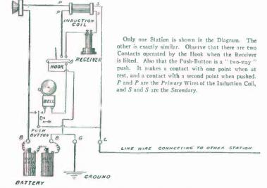
FIG. 153. — Diagram of Connection for a Telephone System employing an Induction Coil at each Station.
