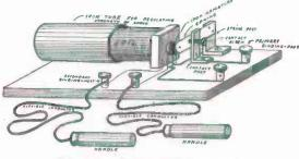
FIG. 156. - Completed Medical Coil.
