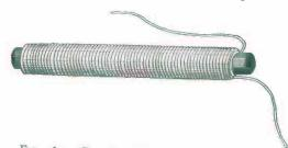
FIG. 160. -Complete Primary Winding and Core.
