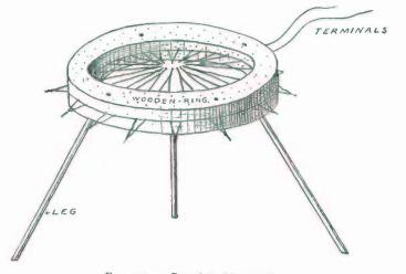
FIG. 305. - Complete Thermopile. An Alcohol Lamp should be lighted and placed so that the Flame heats the Inside Ends of the Wires in the Center of the Wooden Ring.
