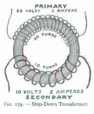
former of about 100 watts capacity, capable of delivering a current of 10 volts and 10 amperes from the secondary will not draw more than approximately one ampere from the 110-volt circuit. This current is only equal to that consumed by two ordinary 16-candle-power lamps or one of 32 candle-power, making it possible to operate the transformer to its full capacity for about one cent an hour. A further advantage is the fact that a "step-down"
