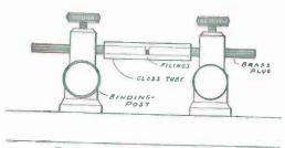
just the right a mount of filings to place in the tube, and how far apart to place the brass rods or plugs.
