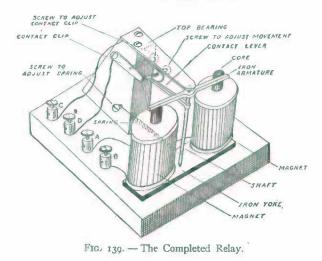
the armature shaft, and the screw mounted on the wooden support with a piece of silk thread. The thread is passed around the shaft once or twice so that the tension of the
