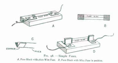
trying to pass than the circuit can safely carry. If a fuse were not placed in such a circuit so as to shut the current off before the danger point is reached, any electrical device might become "burned out," or in extreme cases, the wires become so hot as to cause a serious fire.
