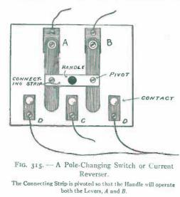
When the switch handle is pushed to the left, the lever A should rest on the left-hand contact, D. The lever B should make contact with C. The motor will then run in one direction. If the handle is pushed to the right so that the levers Aand B make con-
