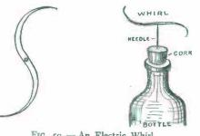
and connected with the prime conductor of the electric machine. When the latter is set in motion, the whirl will commence to revolve at a high rate of speed.
