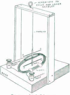
FIG. 112. - Astatic Galvanoscope.
