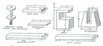
FIG. 136. - Details of the Telegraph Set shown in Figure 135.
