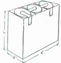
FIG. 294. - A Three-Cell Dry Battery for use in Hand-Lanterns, etc.
