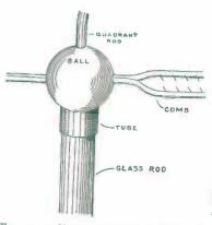
the rod. The rods should be of the proper length to bring the center of the balls on a line with the center of the plates.
