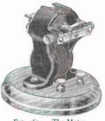
pole motor similar to that shown in Figure 267 will serve very nicely. The wooden base should be removed and the motor screwed down firmly to the floor of the car as in Figure 268. One terminal of the motor is connected to one of the bearings, and the other terminal to the other bearing.
