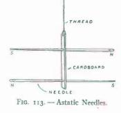
A small hole is punched in the top of the carrier, through which to pass the end of a thread. The upper end of the thread passes through a hole in the bridge and is tied to a small screw-eye in the center of the upper side of the bridge.
