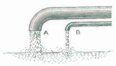
that more water will flow out of the large one than out of the small one. If ten gallons of water flow out of the large pipe in one minute, it may be possible that the comparative sizes of the pipes
