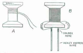
F1G, 118. — Resistance-Coil. A shows how the Wire is doubled and wound on the Spool. B is the completed Coil.
