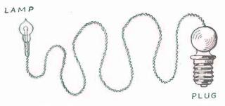
FIG. 300. - A "Pea" Lamp attached to a Flexible Wire and a Plug.
