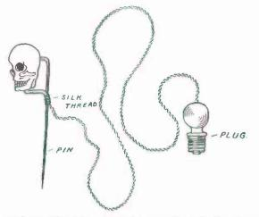
FIG. 302. — The Completed Pin ready to be connected to a Battery by removing the Lamp from a Flashlight and screwing the Plug into its Place.
