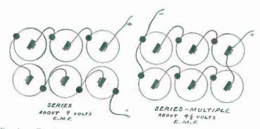
FIG. 69. — Two Methods of Connecting Cells so as to obtain Different Voltage and Amperage Values.
