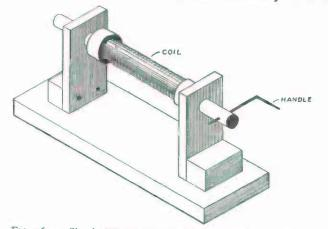
FIG. 162. - Simple Winding Device for winding the Secondary.
