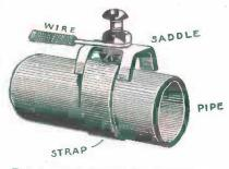
FIG. 200. - A Ground Clamp for Pipes.
