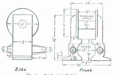
FIG. 255. - Details of the Field Casting.
