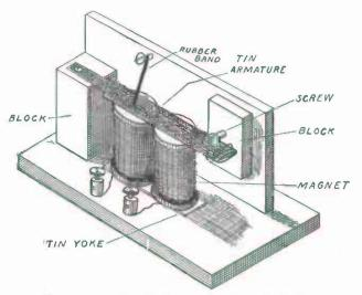
FIG. 133. - A Simple Home-made Telegraph Sender.
