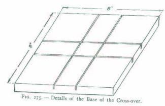
two tracks to cross each other without interference. It consists of a wooden base, eight inches square and threeeighths of an inch thick. Four saw-cuts, each pair exactly parallel, and two inches apart, are made at right angles to each other across the top surface of the base, as shown in the illustration.
