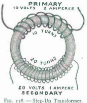
former in Figure 178 represents a "step-up" transformer having ten turns of wire on the primary and twenty turns on the secondary. If an alternating current of 10 volts and 2 amperes is passed into the primary, the secondary winding will double the potential, since it has twice as many turns as the primary and the current delivered
