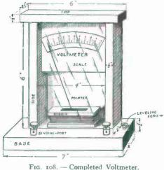
The case is formed of two sides, a back and top of onehalf-inch wood. It is six inches high, four inches wide, and two inches deep. A glass front slides in two shallow grooves cut in the wooden sides, one-eighth of an inch from the front.
