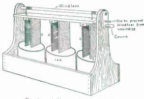
FIG. 64. - A Plunge Battery, with Windlass.
