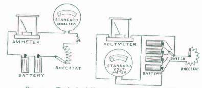
FIG. 109. - Circuits for Calibrating the Ammeter and Voltmeter.
