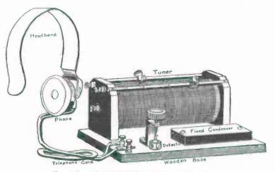
FIG. 316. - A Complete Wireless Receiving Outfit.
