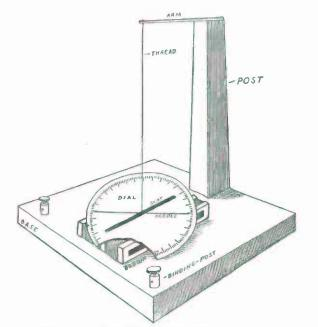
FIG. 115. — Completed Astatic Galvanometer.
