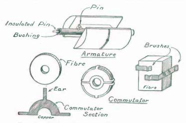
FIG. 253. - Details of the Armature, Commutator, and Brushes.
