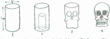
FIG. 301. — Four Steps in Carving a Skull Scarf-Pin. 1. The Bone. 2. Hole drilled in Base. 3. Roughed out. 4. Finished.
