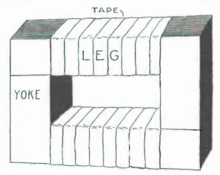
FIG. 181. - The Core, Assembled and Taped.
