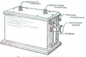
FIG. 221. - A Wireless Spark Coil.
