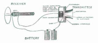
FJG. 145. - A Telephone System, consisting of a Receiver, Transmitter, and a Battery connected in Series. Words spoken into the Transmitter are reproduced by the Receiver.
