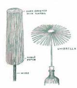
bodies which was illustrated by the action of the pith ball electroscope may be better illustrated by pasting some narrow streamers of tissue paper about one-eighth of an inch wide and four inches long to a small cork covered with tinfoil. The cork is mounted on the upper end of a stiff copper wire supported in a bottle. When the wire is con-
