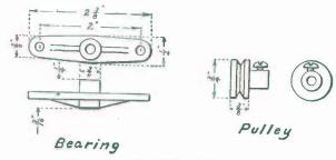
FIG. 260. - The Pulley and Bearings.
