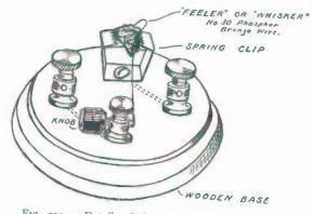
FIG. 212. — Details of the "Cat-Whisker" Detector.
