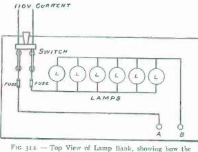
A and B are the Posts to which should be connected any Device it is desirable
