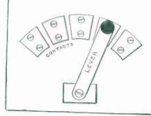
FIG. 189. - The Complete Switch.
