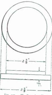
FIG. 320. - The Secondary Head.
