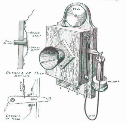
FIG. 149. — A Complete Telephone Instrument. Two Instruments such as this are necessary to form a simple Telephone System.
