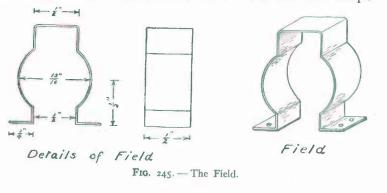
shown in Figure 243. The small bend in the center is most easily made by bending the strip over a knittingneedle and then bending it back to the required extent.
