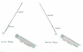
FIG. 10. - An Experiment Illustrating that Like Poles Repel Each Other and Unlike Poles Attract.
