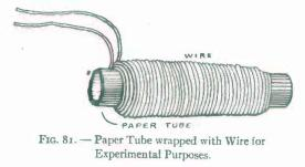
current through it from two or three cells of a battery, and test its magnetic properties by bringing it near a compass needle. It will be found that the coil possesses very marked magnetic properties, and will readily cause the needle to swing about, even though it is held quite a distance away.
