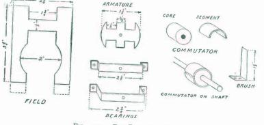
FIG. 249. - Details of the Motor.
