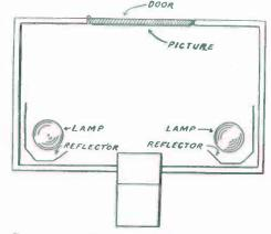
FIG. 300. — A View of the Reflectoscope with the Cover removed, showing the Arrangement of the Lamps, etc.
