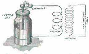
F1G. 317. — Illustrating the Principle of the Tesla Coil. A Leyden Jar discharges through the Primary Coil and a High-Frequency Spark is produced at the Secondary.
