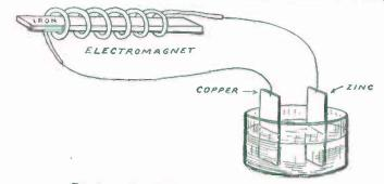
FIG. 83. - The Principle of an Electro-Magnet.
