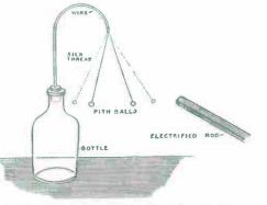
FIG. 23. - A Double Pith-Ball Electroscope.
