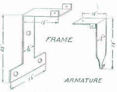
FIG 129. — Details of the Drop-Frame and Armature.
