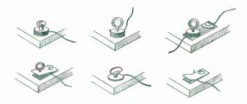
FIG. 93. - Home-made Binding-Posts.
