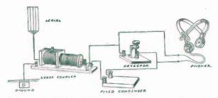
FIG. 219. - Circuit showing how to connect a Loose Coupler.
