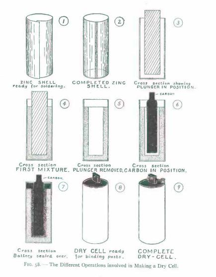
The above paste is then firmly packed into the zinc shell around the wooden plunger, leaving a space of about  $\frac{3}{4}$  of an inch at the top. The paste can be poured in very readily when first mixed but sets and hardens after standing a short while.
