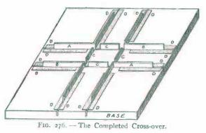
copper. The purpose of these strips is to connect the ends of the track on the cross-over to the ends of the track forming the figure-eight so that the cross-over will not be a "dead" section, that is, a section of track where the car cannot get any current.
