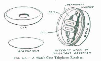
telephone currents pass through the little magnets, they will either strengthen the permanent magnet and assist it in attracting the diaphragm, or detract from its strength and allow the diaphragm to recede, depending upon which direction the current flows.
