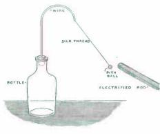
ball. Almost immediately the pith ball will fly away from the glass rod, and no matter how near the rod is brought, it will refuse to be touched again.
