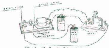
FIG. 236. — The Complete Coherer Outfit.
