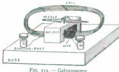
minals, and then, after slipping the coil from the glass, tie the wire with thread in several places so that it will not unwind. Press two sides of the coil together
