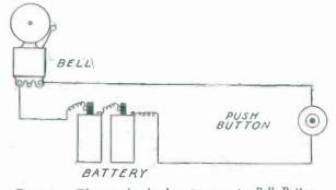
FIG. 122. — Diagram showing how to connect a Bell, Battery, and Push-Button.
