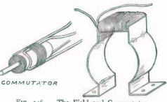
FIG. 246. - The Field and Commutator.
