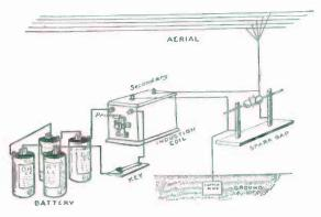
FIG. 194. — A Simple Transmitter.
