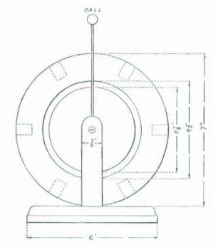
FIG. 321. - End View of the Complete Tesla Coil.
