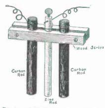
FIG. 60. — A Method of making a Cell Element from Carbon Rods.
