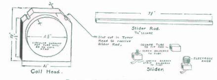
FIG. 201. - Details of the Tuning Coil.
