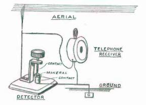
FIG. 195. - A Simple Receptor.
