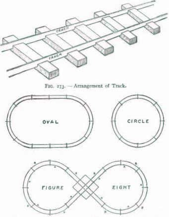
FIG. 274. — Three Different Patterns for laying out the Track. A circle is the easiest form of track to make. In laying out a circle or any sort of curved track, the outside
