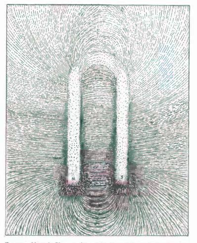
FIG. 14. — Magnetic Phantom showing the Lines of Force about a Horseshoe Magnet,
