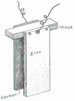
FIG. 59. — A Zinc-Carbon Element, made from Heavy Plates.
