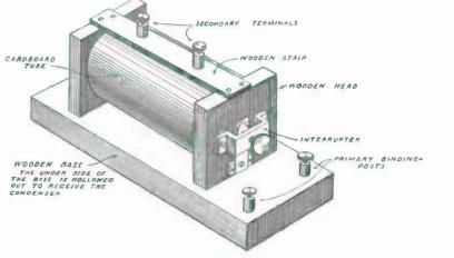
FIG. 166. - Completed Coil.
