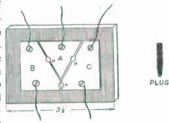
FIG. 100. — Home-made Lightning-Arrester.
