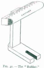
with horsehair. The wood is shellacked and covered with tinfoil previous to tacking on the leather. A strip of wood, two inches wide and one-half an inch thick, is fastened to the back of the rubber. The strip should be just long enough so that when the lower end rests on the base the rubber is level with the axis of the bottle. The lower end may be fastened to the base by means of a small brass hinge. Two rubber bands stretch from
