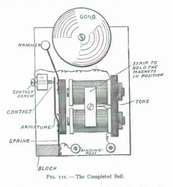
screw. The other end is connected to the binding-post. A second binding-post is connected to the armature.
