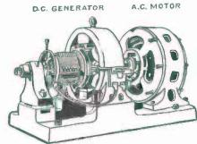
first sent through a set FIG. 177. — Motor Generator Set for changing Alternating Current to Direct Current.
