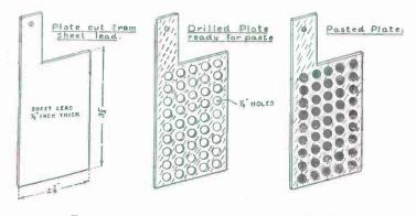
FIG. 71. - How to make the Plates for a Storage Cell.
