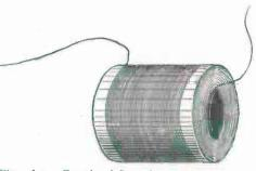
Fig. 163. - Completed Secondary Winding.
