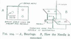
the dents inside of the coil and exactly opposite one another. After the exact position is found, they may be fastened into position by two very small screws.
