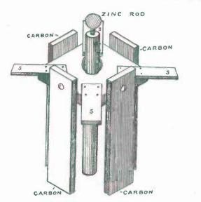
FIG. 62. — A Method of Mounting four Carbon Plates.
