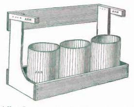
FIG. 65. — A Plunge Battery adapted to a Set of Elements, as shown in Figure 63. They may be lifted out and placed on the "Arms" to drain.
