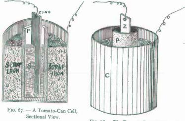
FIG. 68. - The Tomato-Can Cell Complete.
