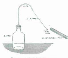
ball. Almost immediately the pith ball will fly away from the glass rod, and no matter how near the rod is brought, it will refuse to be touched again.
