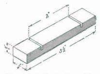
across the top face. This part of the work is best performed in a miter-box so that the cuts will be perfectly square across the ties. A saw should be used which will make a cut of such a size that the steel track will fit tightly into it.
