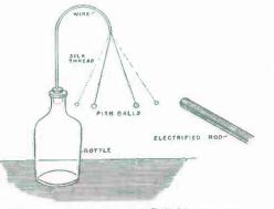
FIG. 23. - A Double Pith-Ball Electroscope.
