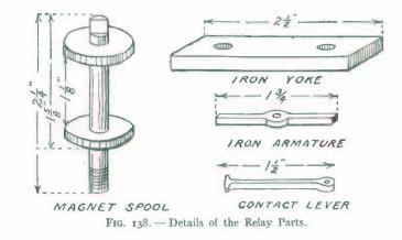
one-quarter inches long. Fit each of the cores with two fiber heads to hold the wire in place. Insulate the legs with paper and wind each with about fifty layers of No. 30 B. & S. gauge single-cotton-covered magnet wire. The winding space between the magnet's heads should be one and oneeighth inches.
