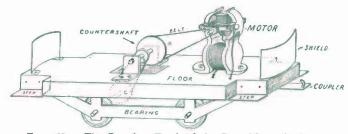
FIG. 268, - The Complete Truck of the Car without the Body.
