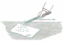
FIG. 17 — An Electrified Glass Rod will Attract in the royal tombs at Small Bits of Paper. Mycenae and at varia
