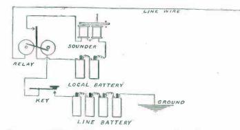
FIG. 1.40. — A Diagram showing how to connect a Relay, Sounder, and Key. Closing the Key will operate the Relay. The Relay will then operate the Sounder in turn.
