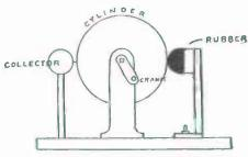
FIG. 29. — Front View of a Cylinder Electric Machine.
