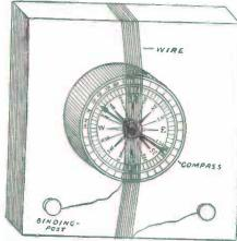
FIG. 110. - Simple Compass Galvanoscope.
