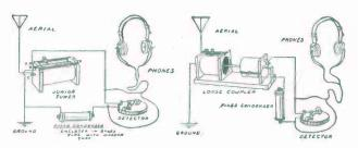
FIG. 220. — A Diagram showing how to connect some of the Instruments described in this Chapter.
