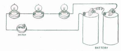
FIG. 288. - How Lamps are Connected in Series.
