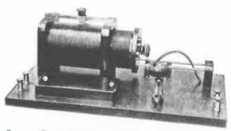
COMPLETE RECEIVING SET. CONSISTING OF A LOOSE COUPLER IN PLACE OF THE TUNING COIL, DETECTOR AND FIXED CONDENSER.
