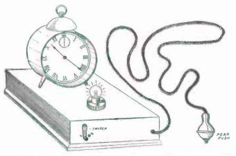
FIG. 298. - An Electric Night-Light for telling the Time during the Night.
