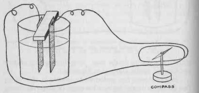
FIG. 224. — Forming a wire which is carrying an electric current into a coil makes the magnetic effect much greater.
