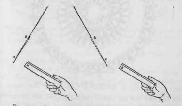
FIG. 210. — An experiment demonstrating that like poles repel and unlike poles attract.
