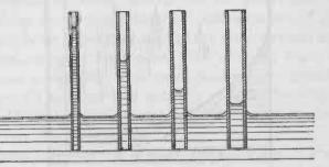
FIG. 78. — Capillary attraction raises water in a tube of small diameter. The water rises to the greatest height in the tube which has the smallest bore.
