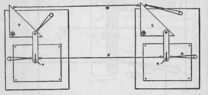
FIG. 54.— Diagram showing how two mechanical telautographs are connected by the strings W and X so as to transmit writing and sketches.
