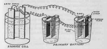
FIG. 222. — Charging the experimental storage cell with the current from two homemade cells.
