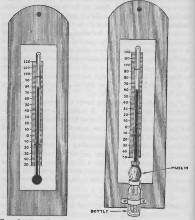
FIG. 278. — An ordinary Fahrenheit thermometer is shown at the left and at the right, the same thermometer converted into a "wet bulb" thermometer.
