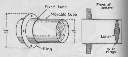
FIG. 200. — The lens of the reflectoscope is a double-convex set in a movable tin tube.
