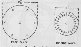
FIG. 148. - The turbine wheel and the face plate.
