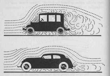
FIG. 72. — The disturbance created in the air by an old-fashioned automobile body is illustrated at the top. At the bottom is shown a modern streamlined automobile body and its effect in moving through the atmosphere.
