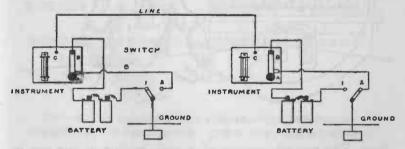
FIG. 242. - The circuit diagram for connecting two telegraph instruments.
