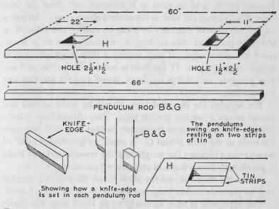
FIG. 59. — Details of the table, pendulum rod for the pen arm and the knife edges used on the harmonograph are shown above.
