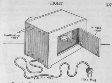
FIG. 198. — Back view of the reflectoscope with the door open.
