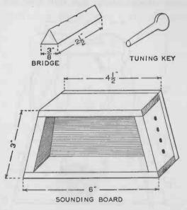
FIG. 123. — The sound box of the door zither is made of wood. At the top are shown the bridge and the tuning key.
