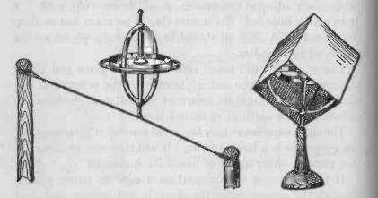
FIG. 66. — The gyroscope walking tight-rope. At the right, the gyroscope is spinning in its box and the box is balanced on one corner.
