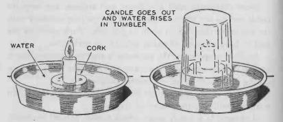
FIG. 9.— This simple apparatus will give a valuable clue regarding the composition of air. The candle will burn for a short time and then go out. The water will rise in the tumbler and there will be much *less* air enclosed in the tumbler.
