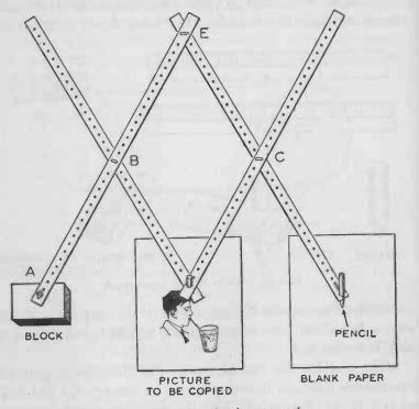
FIG. 50. - The completed pantograph.
