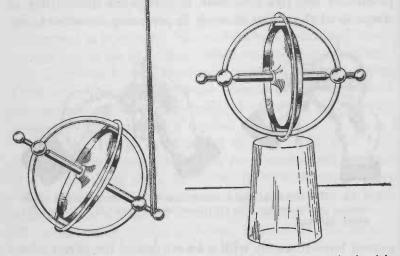
FIG. 65. — At the left a gyroscope is spinning in a loop of string. At the right a gyroscope is shown spinning on its circle on the bottom of a glass tumbler.
