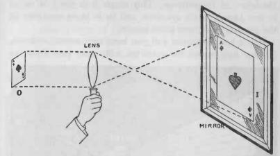
FIG. 168. — Another diagram which shows how a magnifying glass makes objects appear larger than they really are. The dotted lines show the path of the light rays.
