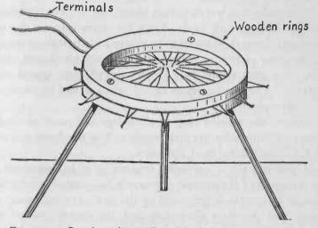
FIG. 144. — Complete thermopile. An alcohol lamp should be placed underneath the thermopile so that the flame heats the inside ends of the wires in the center of the wooden ring.
