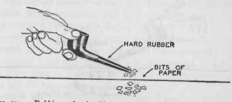
FIG. 204. — Rubbing a hard rubber pipe-stem with a piece of flannel will electrify the rubber so that it will attract small bits of paper.
