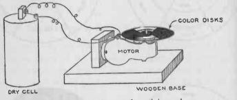
FIG. 173. — The color top for mixing colors.
