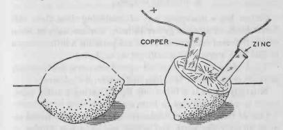
FIG. 29. — The strong acid nature of lemon juice can be shown by the experiment of making a voltaic cell out of a lemon.
