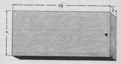
FIG. 286. - The wooden back for the weather glass.
