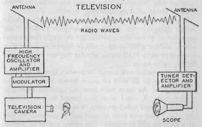
FIG. 247.— The Principle of Television. Notice that a type of antenna different from those shown in Figs. 245 and 246 is shown. The waves used in television are shorter than those commonly used for radio telegraphy and telephony and require a "short-wave antenna."
