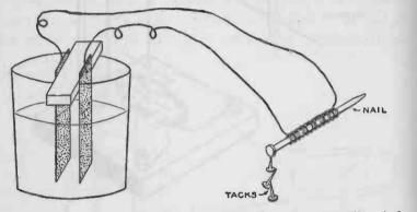
FIG. 226. — If some insulated wire is wound around an iron nail and the terminals of the coil connected to a battery, the nail will become an electromagnet.
