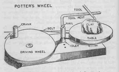
FIG. 31. - The completed potter's wheel ready for operation.
