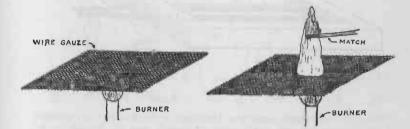
FIG. 136. — If a piece of copper gauze is held in the flame of an alcohol lamp, Bunsen burner or candle, the flame will burn below and not above the gauze, unless a lighted match is held above.
