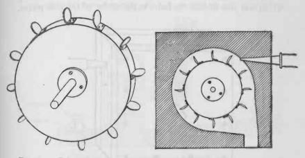
FIG. 104. — The completed wheel with the buckets and shaft in place is shown at the left. Alongside it is the motor with one side piece removed to show the position of the wheel and the nozzle.
