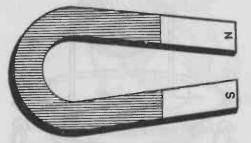
FIG. 4. — The magnet was once only a plaything. It is now an essential part of telephone receivers, magnetos, radio speakers, electrical meters and other instruments.
