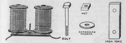
FIG. 227. — At the left is a horseshoe electromagnet. The parts for making a horseshoe electromagnet are also illustrated.
