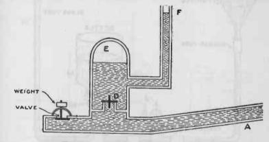
FIG. 106. — Cross-section of a hydraulic ram.
