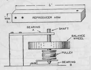
FIG. 130. — The arm which supports the reproducer is shown in the upper part of the illustration. The ower sketch shows the balance wheel and its pulleys.
