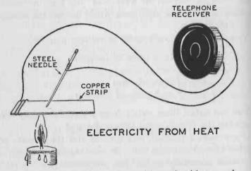
FIG. 143.—An experiment showing how electricity may be generated directly from heat.
