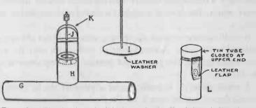
FIG. 108. — The sketch at the left shows the details of the spindle valve for the hydraulic ram. At the right is illustrated the valve L which prevents the water that is pumped upwards into the bottle from flowing back again.
