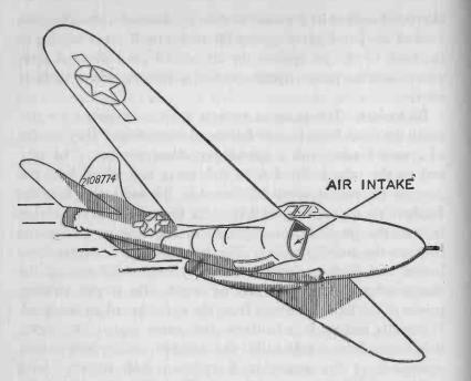
FIG. 72C.—A Propellerless Airplane. The jet-propelled P-59 is driven by gas turbines which suck in air through intakes on each side of the fuselage. The hot gases are jetted through two nozzles astern.
