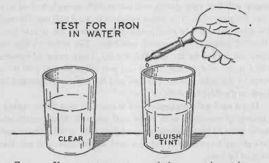
FIG. 13. — You can test water to see whether or not it contains any iron by adding a few drops of a solution of sodium ferrocyanide. If the water contains iron it will assume a bluish tint.
