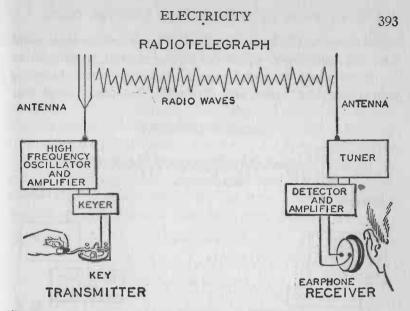
FIG. 245. — The Principle of Radiotelegraphy. By comparing this diagram with Figs. 246 and 247 you will understand that the basic difference between radiotelegraphy, radiotelephony and television lies in the method of modulating or impressing the message on the radio waves.
