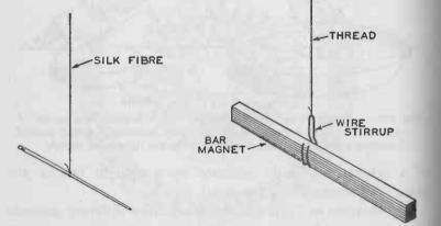
FIG. 213. — Two methods of making simple compasses by suspending bar magnets from threads. The bar magnet at the left is a magnetised sewing-needle.
