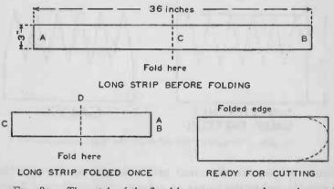
FIG. 282. — The petals of the floral barometer are cut from a long strip of paper folded and trimmed as shown above.
