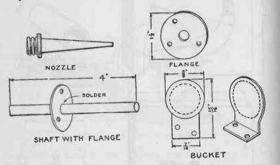
FIG. 103. - Details of the nozzle, shaft and buckets for the water motor.
