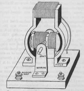
FIG. 233. - A small electric motor which you can build.
