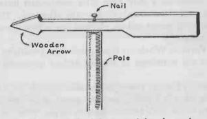
FIG. 262. — A simple wind vane consisting of a wooden arrow pivoted on top of a pole.
