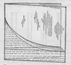
FIG. 79. — You can see the effect of capillary attraction with two panes of glass and some colored water.
