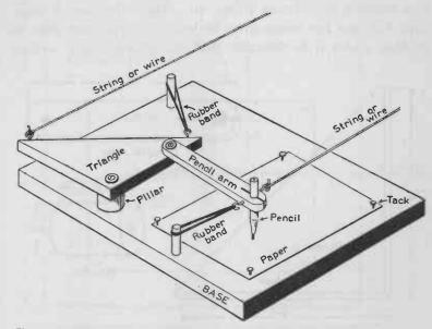
FIG. 51. — A mechanical telautograph like that above will transmit writing and drawing from one room to another.
