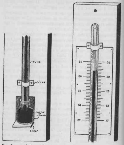
FIG. 289. — At the lower left is shown the lower end of the barometer and at the right, the upper end.
