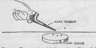
FIG. 205. — The apparatus used in the experiment illustrated above comprises an electrified pipe-stem, can cover, and some fragments of charcoal from a burnt match. The experiment shows the repulsion which takes place between two objects charged with the same kind of electricity.
