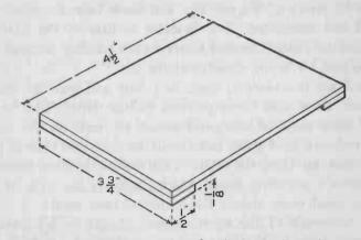
FIG. 241. — The wooden base for the key and sounder.
