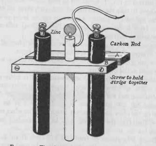
FIG. 210. — The elements of a homemade Voltaic cell, consisting of two carbon rods and a zinc rod may be clamped between two wooden strips. The strips should be painted with paraffin.
