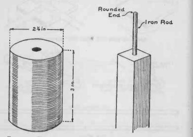
FIG. 271. — The rods and cones are fastened to the wooden cylinder and the cylinder is set upon an iron rod driven into a pole. The upper end of the rod should be rounded.
