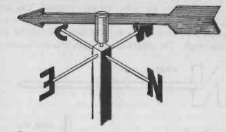
FIG. 265. — A weather vane which shows the points of the compass.
