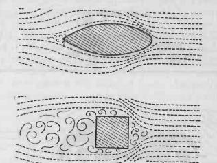
FIG. 71. — The dotted lines represent streams of air slipping past a square object and a streamlined form. Notice the turbulence or "air-hole" stirred up in the wake of the square object. The streamlined object is more easily pushed through the air because it creates less disturbance in its passage.
