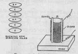
FIG. 217. - A simple Voltaic pile.
