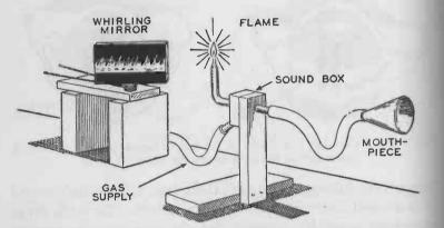
FIG. 116. — The manometric flame apparatus for transmitting the motion of sound waves to a gas flame. The nature of the sound waves is revealed by the image of the flame in a revolving mirror.
