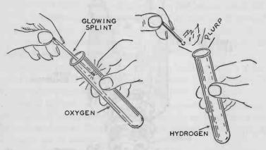
FIG. 11. — If a splinter of wood retaining a glowing spark is immersed in a test-tube containing oxygen, it will instantly burn brilliantly and burst into flame. If a match is held to the mouth of a test-tube containing hydrogen, the gas will burn with a "plurp" sound.
