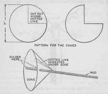
FIG. 269. — The pattern for the cones is a circle with a quadrant cut out as shown. A cone is soldered on each of the four rods.
