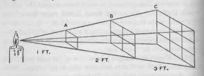
FIG. 159. — This diagram illustrates the law of intensity of illumination. The light from the candle spreads so that the light which falls on the square card one foot away, spreads out and covers a card four times as large two feet away and nine times as large three feet away.
