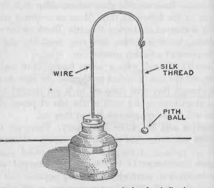
FIG. 206. — An electroscope is a device for indicating the presence of static electricity. A pith ball electroscope consists of a tiny ball of dry pith (you can also use cork) suspended from a silk thread.
