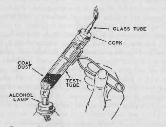
FIG. 25.— An experiment showing how illuminating gas, coke and coal-tar are produced by heating soft coal.
