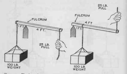
FIG. 43. — If a lever is arranged so that the distance from the fulcrum to the point where the power is applied is 4 times as great as that between the fulcrum and the weight, the pull required to lift the object must be only slightly more than one-quarter the weight of the object to be lifted. A 25 lb. pull will lift a 100 lb. weight.
