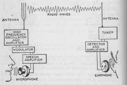
FIG. 246. — The Principle of Radiotelephony.
