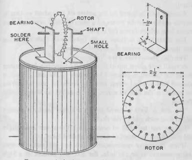
FIG. 145. — A simple steam turbine made from a tin can.
