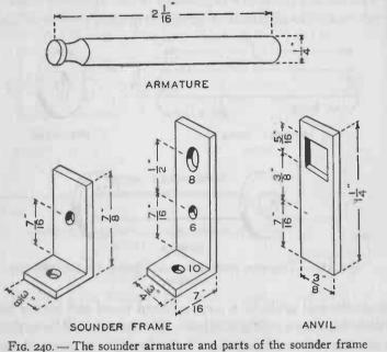
FIG. 240. — The sounder armature and parts of the sounder trame and anvil.
