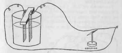
FIG. 223. — Oersted's famous experiment by means of which he discovered that an electric current will produce magnetism.
