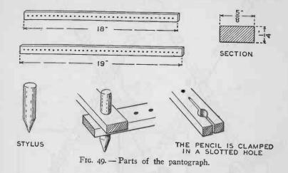
sixteenth of an inch in diameter. One of the long sticks should have a large hole, into which a pencil will fit tightly, bored an inch from one end.
