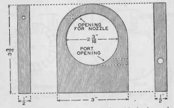
FIG. 149. — The turbine casing is made of wood in the shape and according to the dimensions shown above.
