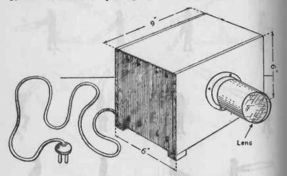
FIG. 197. — The completed reflectoscope from the front.
