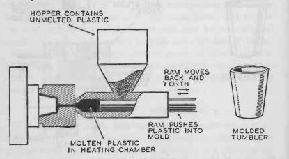
FIG. 33C. — Molding a Thermoplastic Plastic. This is a more rapid process than molding a thermosetting plastic. The mold shown is also for making a molded tumbler. The portion of the mold called the cavity is shown in section.
