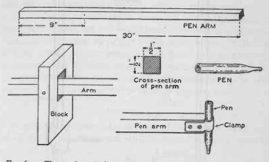
Fig. 60. — The pen is made from a piece of glass tubing. It is clamped on the end of the arm and the arm is supported in the block.
