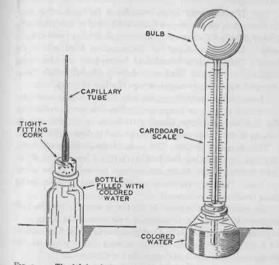
FIG. 142. — The left-hand sketch shows a bottle filled with colored water and provided with a capillary glass tube passing through a tight-fitting cork. At the right is shown an air thermometer.
