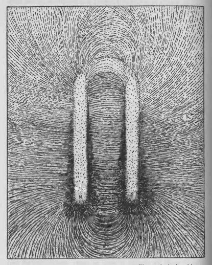
FIG. 215. — The phantom of a horseshoe magnet. The method of making a magnetic phantom is explained in the text.
