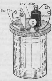
FIG. 231. — A simple homemade electric lamp.
