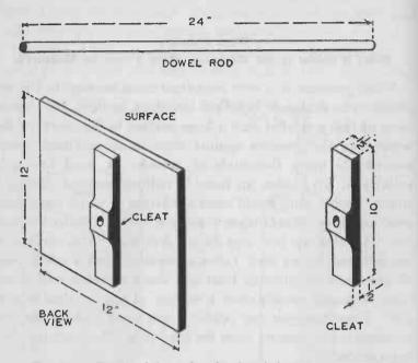
FIG. 272. — Details of the surface for the wind pressure gauge.
