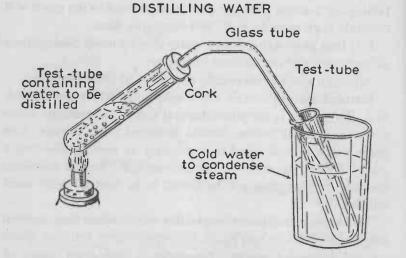
FIG. 12.— A simple distilling apparatus. Steam formed by boiling water in the left hand test-tube passes through the glass tube and is condensed into pure distilled water in the right hand tube.
