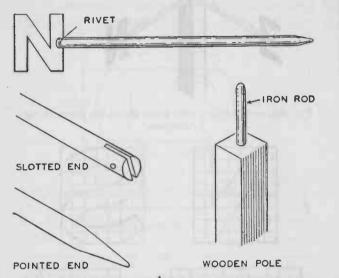
FIG. 267. — One end of each "rod is pointed and the other is slotted. The letters are riveted or soldered into the slotted ends of the rods. The vane is set upon an iron rod driven into the top of the pole.
