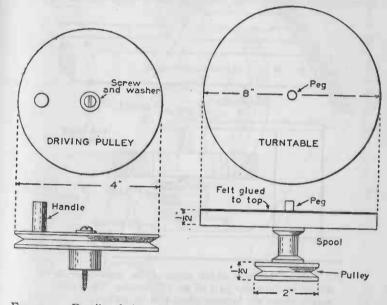
FIG. 129. — Details of the wooden turntable and driving wheel for the phonograph.
