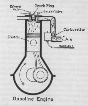
FIG. 157. — Diagram of an internal combustion engine of the type used in automobiles and commonly called a gasoline engine. Compare this with the diagram of a Diesel engine.
