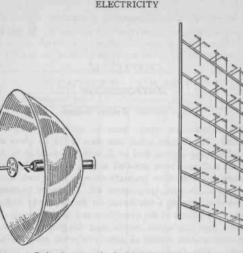
FIG. 251. — Radar Antennas. At the left is the parabolic reflector type and at the right a "bedspring" antenna.
