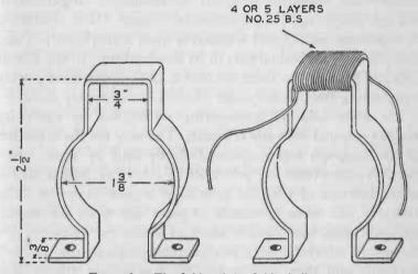
FIG. 236. — The field and the field winding.
