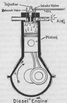
FIG. 158. - Diagram of a Diesel engine.
