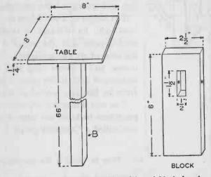
FIG. 58. — Details of the table, stick and block for the harmonograph are shown above.
