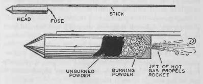
FIG. 72B. — The Skyrocket. In the enlarged view of the head the case is shown cut away to reveal the burning powder and the hot gases which form the jet.
