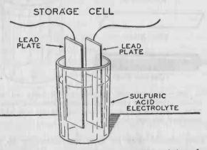
FIG. 221. — An experimental storage cell consisting of two strips of sheet lead immersed in a solution of sulfuric acid in water.
