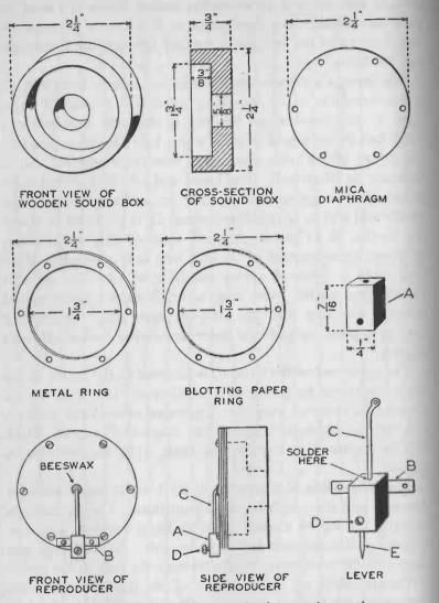
FIG. 128. - Details of the home-made phonograph reproducer.
