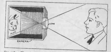
FIG. 178. — The principle of the camera is very similar to that of the eye.
