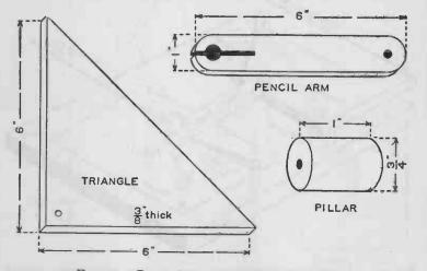
FIG. 52. - Parts of the mechanical telautograph.
