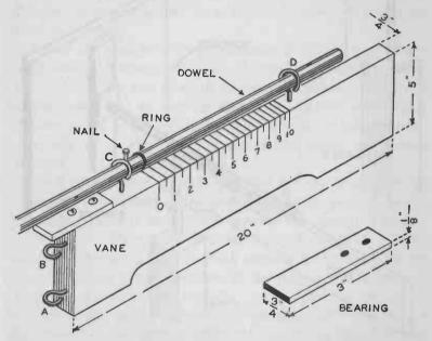
FIG. 273. - Details of the vane and the bearing for the wind pressure gauge.
