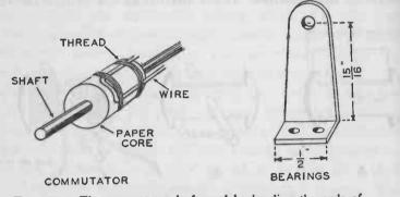
FIG. 235. — The commutator is formed by bending the ends of the armature wires and binding them in position on the paper core. The bearings are made according to the shape and dimensions shown above.
