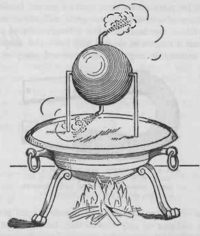
FIG. 3.— The Greek toy called an Eolipile was the forerunner of the modern steam engine. It consisted of a shallow vessel of water closed by a tight-fitting lid and connected to a hollow ball by tubes. When heat was applied and the water boiled, steam escaping from the jets caused the ball to revolve.
