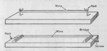
FIG. 121. — At the top is a simple sonometer and below a more elaborate form provided with bridges and tension screw.
