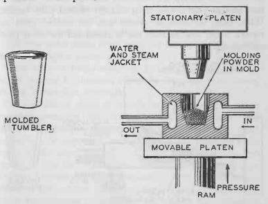
FIG. 33B. — Molding a Thermosetting Plastic. Heat and heavy pressure, the latter supplied by a hydraulic press, are required. The mold is for making the molded tumbler shown at the left. The portion of the mold called the cavity is shown in section.
