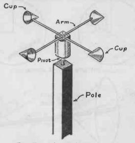
FIG. 268. — A homemade anemometer.
