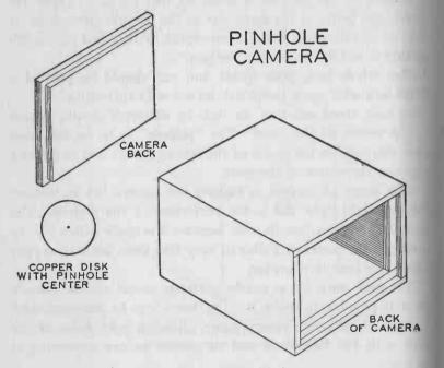
FIG. 180. - Details of the pinhole camera.
