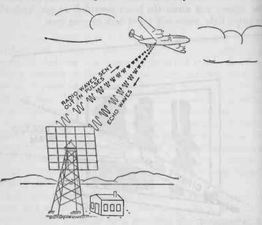
FIG. 249. — The Principle of Radar. Radio waves are sent out in pulses. When they strike an object they are reflected back to the transmitter. Ingenious apparatus locates the reflecting object.
