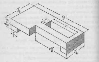
FIG. 151. - The wooden bed for the steam engine.
