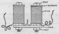
FIG. 228. — An electromagnet made with the parts shown in Figure 227.
