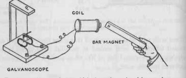
FIG. 229. — An experiment which shows how electricity can be generated by magnetism and motion.
