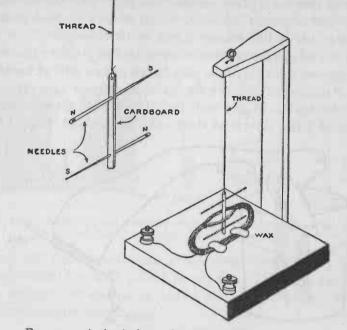
FIG. 225.—A simple form of Astatic galvanoscope which a boy can build.
