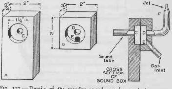
FIG. 117. — Details of the wooden sound box for producing manometric flames.
