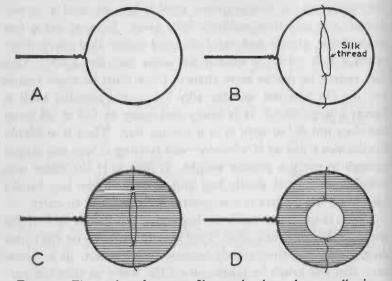
FIG. 75. — The tension of a water film can be shown by a small wire frame (A) with a loop of thread tied across it as at B. Dip the frame in a soap solution so as to form a soap film on the frame as at C. If the film is broken inside the loop by means of a hot wire, the tension of the film will pull the thread into a circle.
