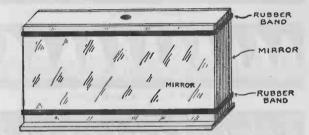
FIG. 119. — The mirrors are cemented to the wooden block with cement or glue. The rubber bands are added for safety sake to prevent the mirror from flying through the air if it should become loosened while rotating.
