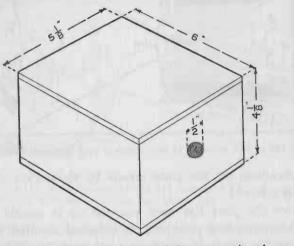
FIG. 179. — The box of the pinhole camera viewed from the front. The copper disk bearing the pinhole is placed over the hole in the front of the box.
