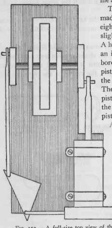
file and a piece of emery paper. The piston rod should be made from a piece of oneeighth-inch brass rod which is slightly flattened at both ends. A hole, three-thirty-seconds of an inch in diameter should be bored near each end of the piston so as to accommodate the "crank" and "wrist" pins. The crank pin fastens the piston rod to the crank and the wrist pin connects the piston rod to the piston.
