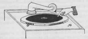
FIG. 126.—A simple experiment which shows that there is really no mystery about a talking machine. If you hold your finger nail in the sound track on a revolving phonograph record your finger nail will vibrate and reproduce the sounds recorded on the record.
