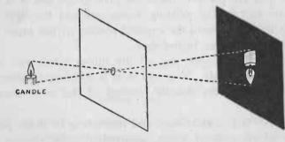
FIG. 176. — The image of a candle flame may be produced on a screen by letting light rays pass through a small hole in a piece of cardboard.
