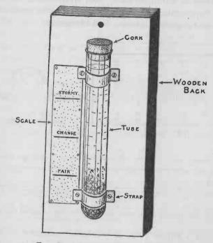
FIG. 287. - The completed weather glass.
