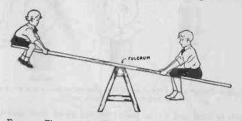
FIG. 44.— The seesaw is a form of lever. A light weight at one side will balance a much heavier weight on the other side if the lighter weight is farther away from the fulcrum.
