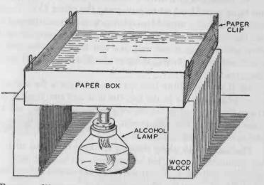
FIG. 135. — Water may be boiled in a paper box over the flame of an alcohol lamp or a Bunsen burner. The water draws the heat away from the paper so rapidly that it cannot become hot enough to ignite and burn until the water has boiled away.
