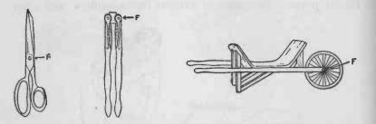
FIG. 41. — A pair of scissors, a nut-cracker and a wheel-barrow are common forms of levers. The fulcrum is located at the point marked F in the illustration.
