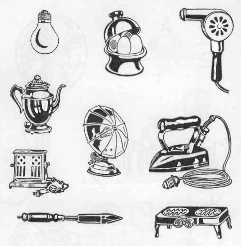
ELECTRICAL DEVICES EMPLOYING THE HEATING EFFECT OF AN ELECTRIC CURRENT
