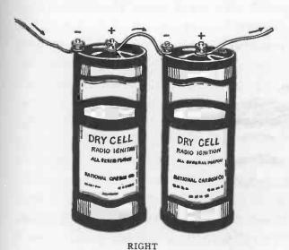
The right way to connect two dry cells in series.
