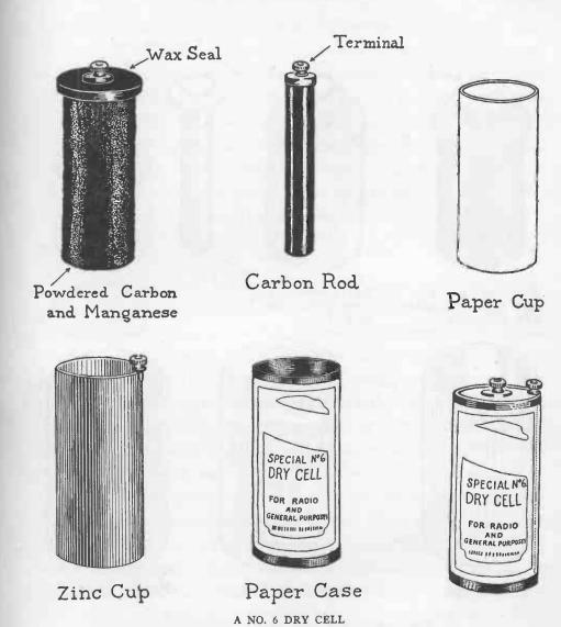
If you take a dry cell apart you will find it is made of the parts shown in this sketch. No. 6 indicates the size, namely 6 inches high by 2½ inches in diameter.
