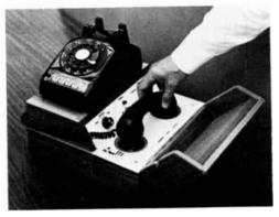
An acoustic coupler converts data to electronic impulses for transmission through telephone lines.
