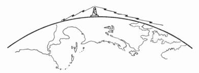
A signal from a TV tower can travel only 20 or 30 miles before it strikes the earth or is lost in space.
