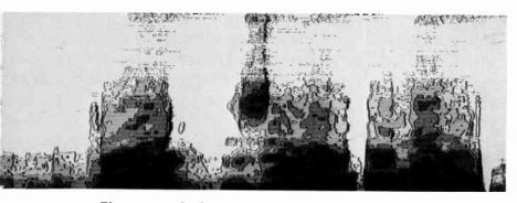
The sonagraph charts the spoken words, "four zero Ohio," by "spreading out" the voice on a sonagram.
