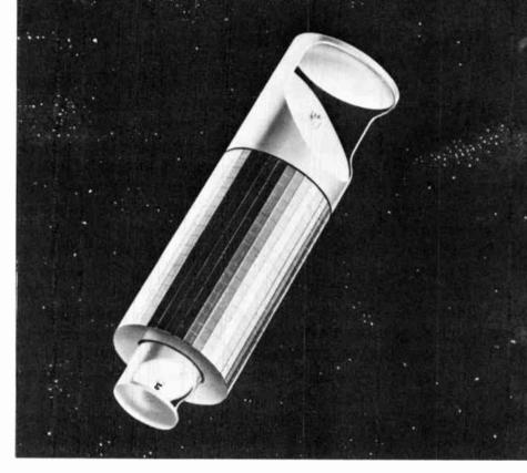
The A T & T design proposal for a satellite utilizing pulse code modulation and frequency modulation techniques.
