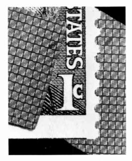
Electronic components developed at Bell Labs for use in integrated circuits. Each square, smaller than a stamp perforation hole, contains 672 transistors and resistors.
