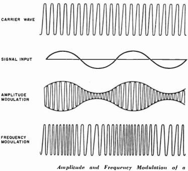
Amplitude and Frequency Modulation of a Carrier Wave by a Signal Input.
