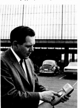
Bell Labs' battery-operated mobile phone unit, equipped for dialing and ringing.
