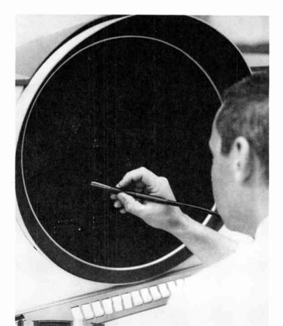
ical data onto tape in a matter of minutes. He does this by "writing" directly on the tube face with an electronic "light pen."
