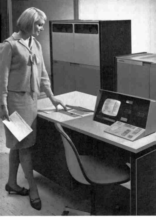
Ampex's Videofile handles document filing and retrieval, replacing file folders with television recordings that may be updated electronically.
