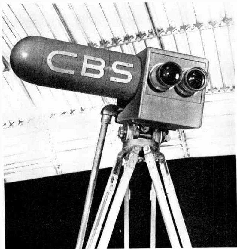
Color camera used in 1940-41 demonstrations at CBS. The revolving color disk is in projecting tube at right of camera.
