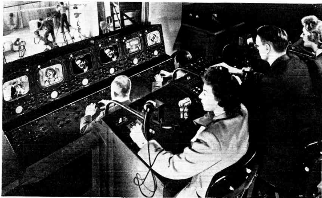
The General Electric control in Schenectady. Director, switching engineer, and sound engineer in foreground. Multiple viewing panel with video engineers in front of them. Fourth screen from left is line monitor. Studio is seen through window in upper left of picture.
