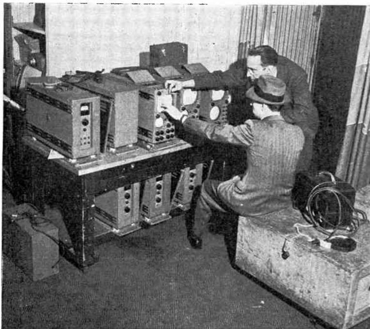
The portable control equipment necessary at the point of pickup in addition to cameras when the truck is not used.
