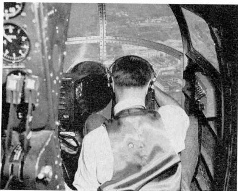
A television camera in the nose of a plane and the pictures received on the viewing screens at the control point in recent tests. The results possible through the use of television cameras in robot planes are clearly evident.
