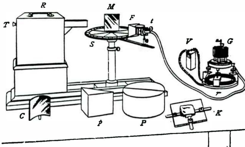
*R*, the Radiator. *T*, the Tapping Key. *S*, the Spectrometer-Circle.
