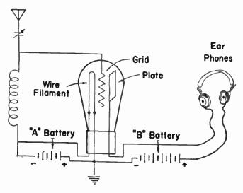
A TUBE USED TO AMPLIFY RADIO SIGNALS
