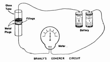
a spark near by, by means of a Hertz exciter, the filings clung together and the current from the battery would be registered by the meter's pointer. When the spark ceased, the
