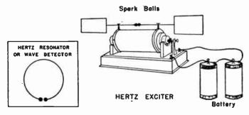
He constructed a device he called an "exciter," consisting of an induction coil, with metal balls attached to the ends of the high-voltage coil. Rising out of each ball was a rod terminating in a metal plate. It was his theory that when the high-voltage current caused a spark to leap from one ball to the other, electric waves would be generated and discharged into the air through the metal plates.
