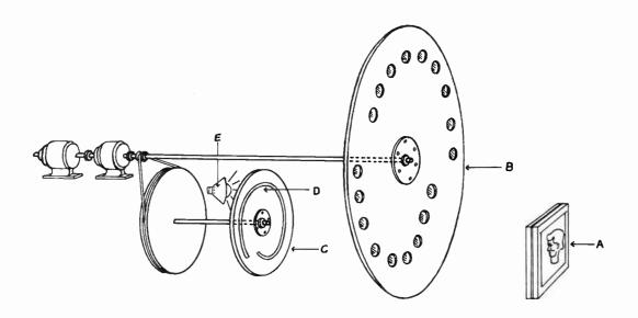
A - REPRODUCED IMAGE (on ground glass screen) B- REVOLVING DISC WITH LENSES
