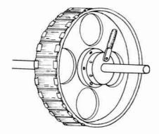
Above The mirror drum arrangement for scanning used by Baird after 1931.
