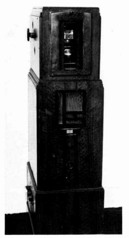
Above Baird's mirror drum receiver of 1932, built by Bush. The picture was made of 30 lines, scanned vertically by mirror drum.
