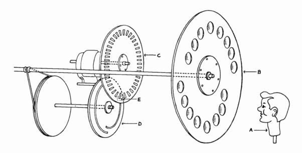
A - DUMMY'S HEAD (object to be transmitted) B- REVOLVING DISC WITH LENSES
