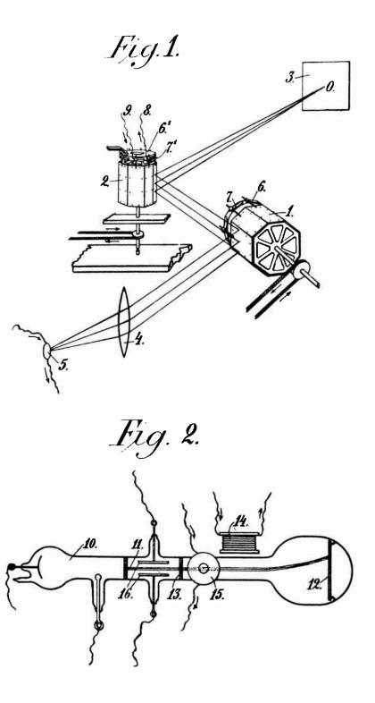
*Right* Rosings patent. Above, the scanning mirrors, and below, the cathode ray tube. The source of electrons is at 10. 15 and 16 are the electromagnets, and 12 is the fluorescent screen that shows them up.
