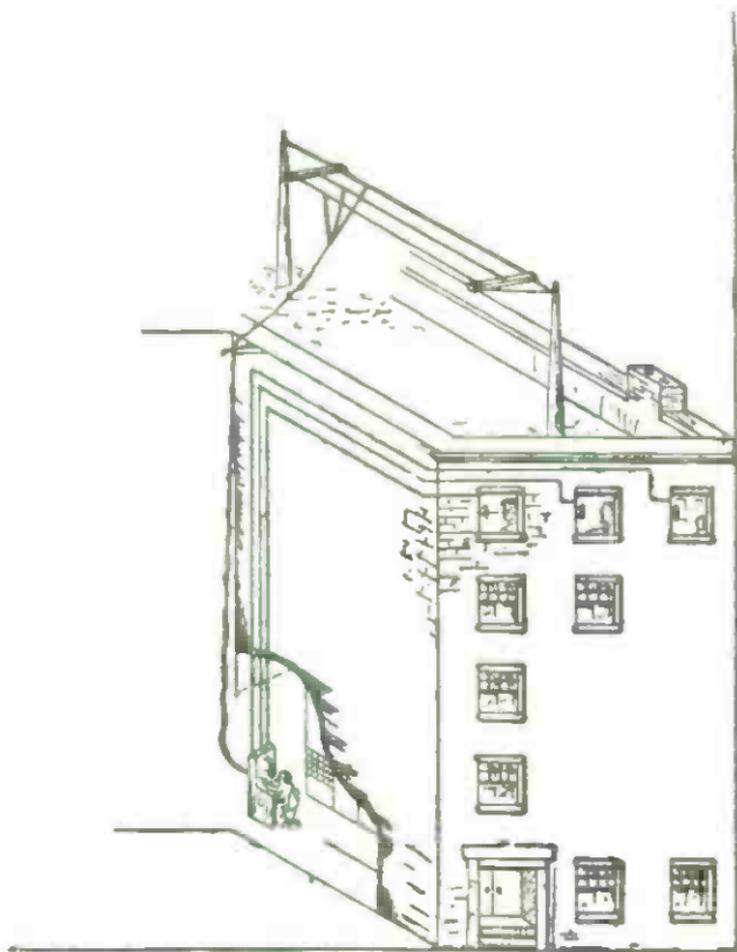
*Apartment houses and hotels can have a radio telephone receiver in every apartment. A common aerial on the roof and a common receiving set in the basement with telephone or loud-speaker connections in the apartments—nothing more is required*
