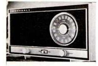
TABLE MODEL AM/FM radio by Motorola. Seven tubes, rectifier, vernier tuning, fiveinch speaker, automatic frequency control on FM, automatic volume control on AM, tuned RF stage. Available in beige or white. Price \$39.95.
