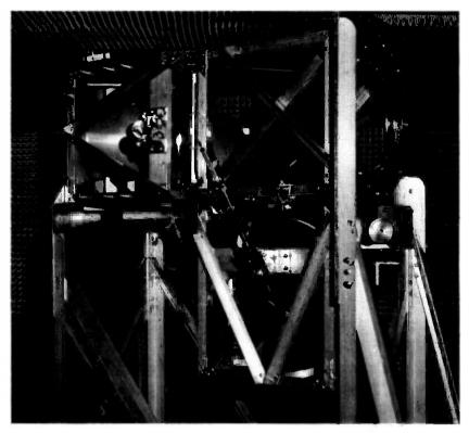
Fig. 10—A  $19/28.5~\mathrm{GHz}$  duo-polarization quasi-optical feed system (see Fig. 3) for the beacon measurements.
