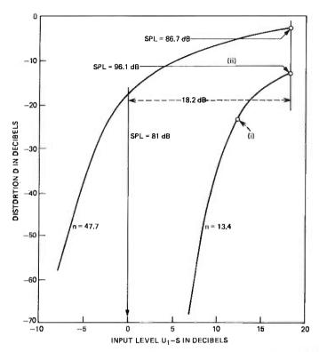
Fig. 4—Total harmonic distortion D defined in (27) versus input signal level  $U_1$  defined in (53) relative to sensitivity level S defined in (56) for two values of n. Various sound pressure levels SPL are indicated; for all n,  $U_1 = S$  corresponds to SPL = 81 dB. Points (i) and (ii) are chosen for waveform examination in Fig. 5.
