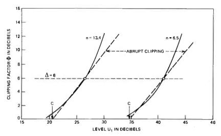
Fig. 7—Clipping factor (21) versus level (53) for two illustrative values of n. Dashed lines represent abrupt clipping approximation (61) which defines the clipping level C of the receiver. The clipping discount  $\Delta$  (see Appendix A) is chosen as  $\Delta = 6$  dB.
