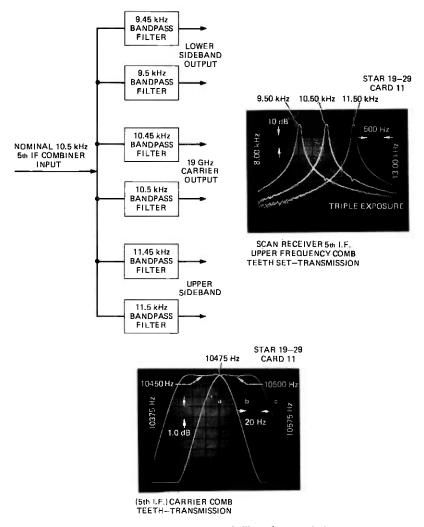
Fig. 6—Scanning receiver comb filter characteristics.
