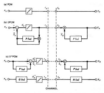
Fig. 1-Structures of PCM, DPCM, and D\*PCM coders.
