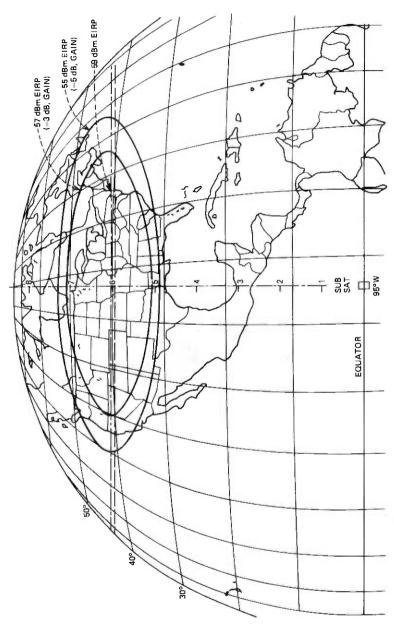
Fig. 2.—28-GHz beacon coverage from satellite at 95°W longitude. Maximum antenna gain is 30 dB. Coverage for 19-GHz beacon is similar.
