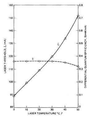
Fig. 10—Laser threshold and differential quantum efficiency as a function of the laser temperature.
