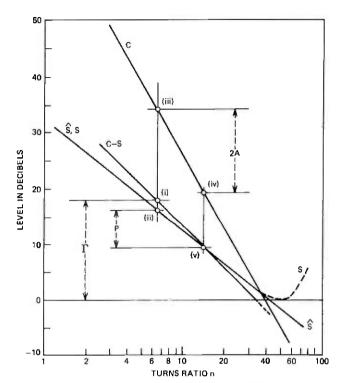
Fig. 9—Receiver clipping level C defined in (61) versus n. Also shown are C - S, S, and S, where S is the sensitivity level (56) and S is the sensitivity level for the distortion-free receiver defined by (52). Points (i) to (v) trace the quality matching procedure based on (54), (63), (69), (70), and (74).
