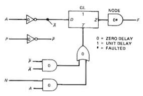
Fig. 8.—The CMOS tri-state inverter model. Only the gate marked \* is faulted by the simulator. Propagation delays are denoted by either 0 or 1.
