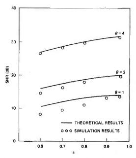
Fig. 2—DPCM performance: SNR vs. value a of the predictor coefficient. Source: Gaussian first-order Markov source with correlation  $\rho=0.9625$ . Quantizer: B-bit quantizer optimized for Gaussian signals. Predictor: Previous sample prediction with coefficient a.
