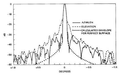
Fig. 15—99.5-GHz scan over a 2 degree range measured with prime-focus dual-mode feed of 20-dB taper. The difference between measured far sidelobe levels and the calculated pattern envelope for perfect surface is consistent<sup>5</sup> with 0.1 mm rms surface tolerance. The higher near-sidelobe level in the elevation plane stems from large-scale surface distortion.
