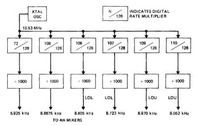
Fig. 10—Receiver fourth local oscillator in control room (crystal oscillator frequency is  $10.533333~\mathrm{MHz}$ ).
