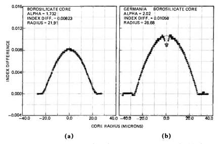
Fig. 1—Refractive-index profiles derived from interference micrographs: (a) a borosilicate graded-core fiber; (b) a germania borosilicate core fiber. The fitted curves are determined from a weighted [eq. (1)] nonlinear least-squares fit to the data  $\Theta$ .
