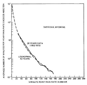
Fig. 20—Comparison of 43-year (1908–1950) distribution of 5-minute rain rate calculated by extreme value theory and lognormal hypothesis (dashed line) with 20-year (1953–1972) data (solid line) at Sheridan, Wyoming.
