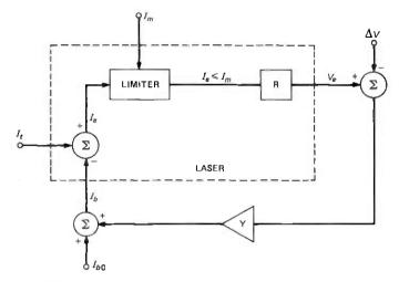
Fig. 6—System representation of the modified ABC circuit.
