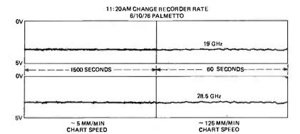
Fig. 11—Periodic amplitude variations. Amplitude scales are linear in voltage; thus the 19-GHz periodic ripple is about 0.2 dB in magnitude. The periodicity was not obvious until the chart speed was increased. At 5 mm/min the variation looked random; however, at 125 mm/min the periodicity becomes apparent.
