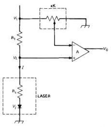
Fig. 8—Circuit to monitor the laser junction voltage.
