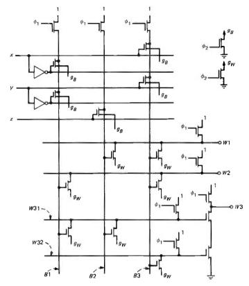
Fig. 17—Dynamic pseudo NMOS programmable logic array (PLA). There are three input variables (x, y, z) and three outputs (W1, W2, W3). Pull-up FETs are PMOS; all others are NMOS.<sup>7</sup>
