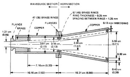
Fig. 6—The 19(28.5)-GHz conical corrugated horn and its hybrid mode launcher.
