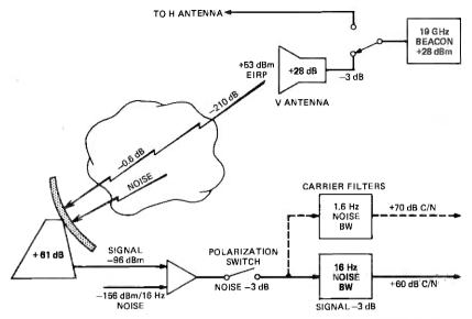
Fig. 6—Radio link summary indicating major parameters that determine the carrier-tonoise ratio of the 19-GHz COMSTAR beacon signals received in clear air with the Crawford Hill main receiving facility.
