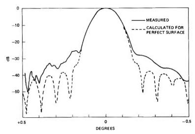
Fig. 16b—28.5-GHz elevation pattern with prime-focus feed of 20-dB taper. The measured first sidelobe level is  $-25~\rm dB$  compared with  $-16~\rm dB$  at  $99.5~\rm GHz$  in Fig. 15.
