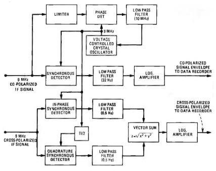
Fig. 5—Synchronous envelope detectors.
