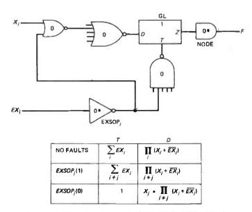
Fig. 21—The general case: S-OP and S-ON faults (0-dominant).
