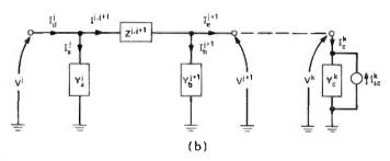
Fig. 2—Interaction model for multiconductor segments and general terminal constraint.
