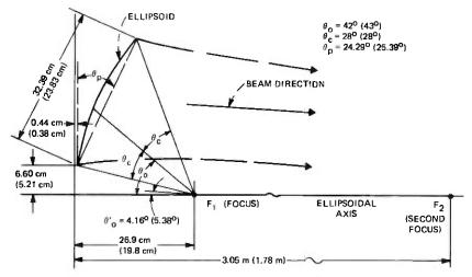
Fig. 8-Schematic diagram of the 19(28.5)-GHz offset ellipsoid.
