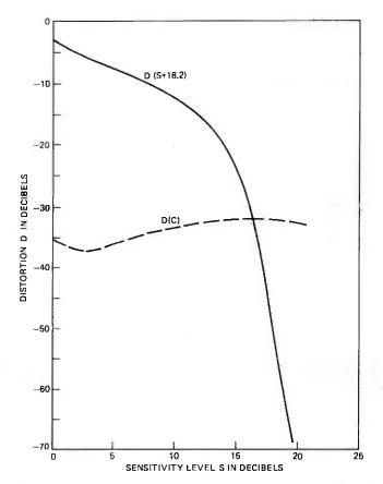
Fig. 6—Total harmonic distortion D (S + 18.2) at the channel clipping level for the case  $\Gamma$  = 18.2 dB versus sensitivity level S defined in (56). Dashed curve shows D(C) at receiver clipping level C defined in (61).
