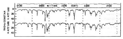
Fig. 4—Typical data obtained from COMSTAR interim experiment (Hurricane Belle, August 9, 1976).
