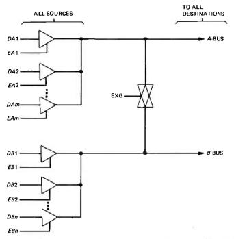
Fig. 14—Two bilateral tri-state buses connected by a transmission gate. All data sources (drivers) are grouped on the left. All data sinks (gate inputs) are to the right.
