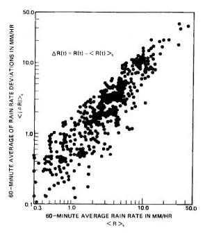
Fig. 24—Two-year data on correlation between hourly mean rain rate,  $\langle R \rangle_s$ , and hourly mean deviation,  $\langle |\Delta R| \rangle_s$ , measured by the tipping bucket rain gauge at Palmetto, Georgia.
