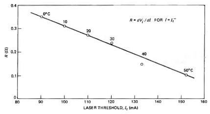
Fig. 7-R as a function of the laser threshold.
