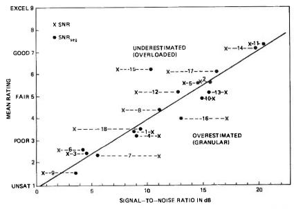
Fig. 10—Mean ratings for the 18 coders vs. SNRs showing the improvement in prediction by measuring SNR segmentally. The solid line is the graph of formula 2, Table III, the regression of rating on  $\text{SNR}_{\text{seg}}$ .
