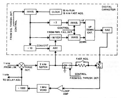
Fig. 15-1-kHz digital phase-locked loop (PLL).
