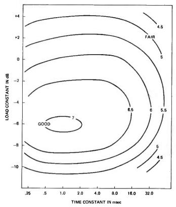
Fig. 8—Equi-rating contours predicted by formula 8, Table III, for 4-bit ADPCM coders.
