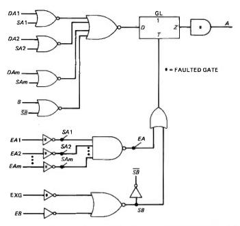
Fig. 16—The A-bus faulted model. Only gates marked \* will be faulted by the simulator. Two SA0/SA1 node (pin) faults and m+1 pairs of stuck-open/stuck-on faults have been assigned. The B-bus faulted model is analogous.
