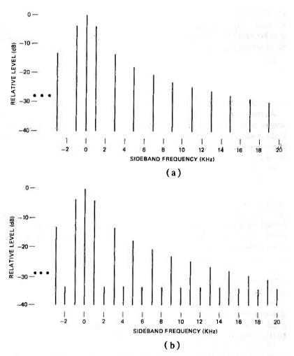
Fig. 12—19-GHz polarization-switching sideband levels, with and without switching asymmetry. Note the even-order sidebands present with switching asymmetry.
