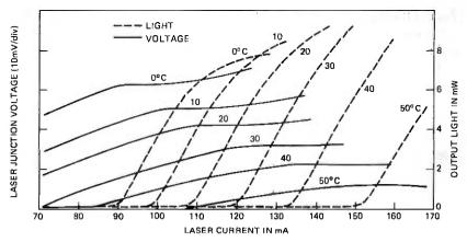
Fig. 5—Laser junction voltage and output light as a function of the bias current and the temperature.
