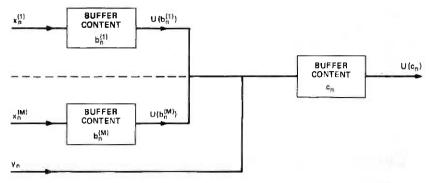
Fig. 1—Schematic of pooling of data from several buffers into a single buffer.
