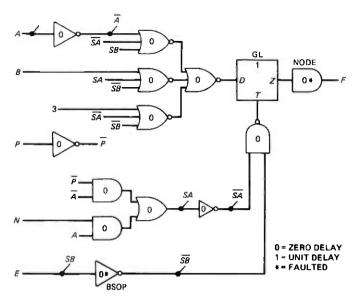
Fig. 10-The CMOS modified tri-state inverter model.
