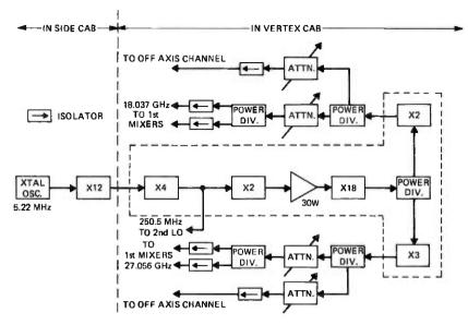
Fig. 5—Receiver first local oscillator (crystal oscillator frequency is 5,218991 MHz).
