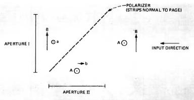
Fig. 2—Polarization separator geometry for 12-foot antenna.
