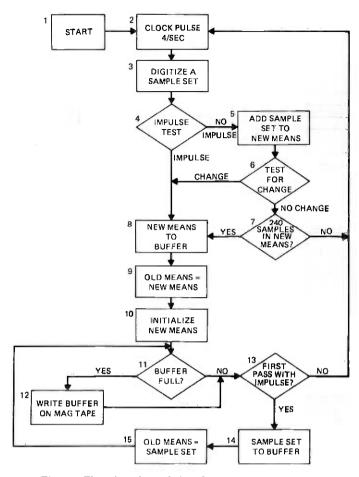
Fig. 17-Flow chart for real-time data screening software.
