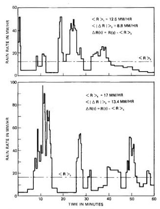
Fig. 23—Time-varying rain rate measured by a tipping bucket rain gauge at Palmetto, Georgia.
