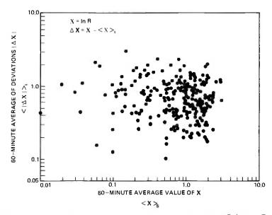
Fig. 25—Two-year data measured by the tipping bucket rain gauge at Palmetto, Georgia, demonstrating that the hourly mean deviation,  $\langle |\Delta X| \rangle_s$ , and the hourly mean value,  $\langle X \rangle_s$  are uncorrelated, where  $X = \ln R$ .
