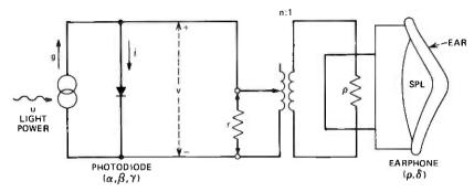
Fig. 1—Circuit of photovoltaic receiver. The earphone resistance  $\rho$  is transformed to r.
