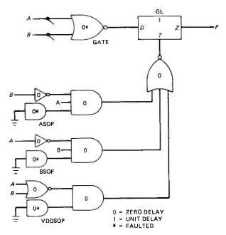
Fig. 4—The CMOS two-input NOR gate model, NR2. The block labeled GL is the gated latch circuit of Fig. 3. Only those gates marked \* are faulted by the simulator. Propagation delays are denoted by either 0 or 1.
