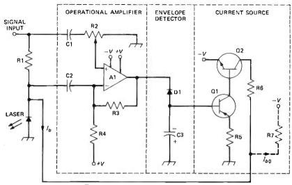
Fig. 2-Automatic bias control circuit.
