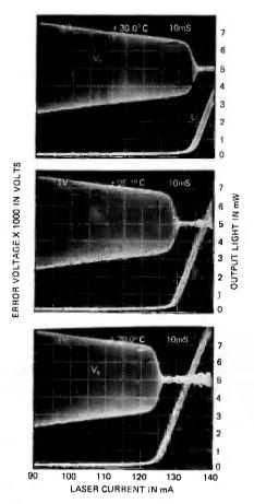
Fig. 9—Voltage at the output of the operational amplifier and laser output light as a function of the laser bias current at three different temperatures and without feedback connection.
