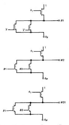
Fig. 18—Subcircuit portions of the PLA of Fig. 17.
