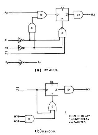
Fig. 19—PLA subcircuit models. Gates marked \* are faulted by the simulator, and 0 and 1 denote delays.
