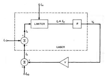
Fig. 4—System representation of the ABC circuit.
