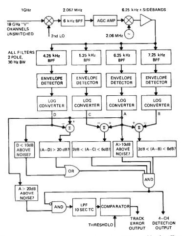
Fig. 13—Four-filter acquisition detector (part of receiver second local oscillator  ${\sf AFC}$  circuitry).
