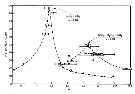
Fig. 5—Root-mean-square pulsewidth reduction factor  $\sigma(\text{step})/\sigma(\text{graded}) = [\Delta NL/(12)^{1/2}c] \ 1/\sigma(\text{graded})$  is plotted vs.  $\alpha$  for germania borosilicate and borosilicate fibers. Data points ( $\square$  for GBS fibers;  $\bullet$  for BS fibers) were obtained by deconvolving expected material dispersion effects (0.12 ns/km for GBS fibers, 0.09 ns/km for BS fibers) from the measured fiber output pulsewidths.
