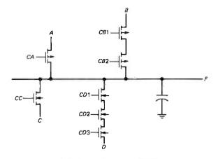
$T = EA \cdot \overline{EASDP} + EB \cdot \overline{EBSOP} + EC \cdot \overline{ECSOP} + \cdots$ WHERE  $EA = \overline{CA}, EB = \overline{CB1} \cdot \overline{CB2}$   $EC = CC, ED = CD1 \cdot CD2 \cdot CD3$
