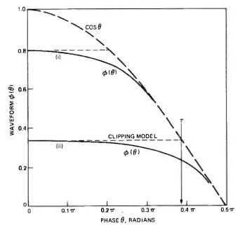
Fig. 5—Normalized waveform (20) for points (i) and (ii) of Fig. 4 for half of fundamental range of  $\theta$ . The clipping model approximation is shown dashed and the parameter  $\tau$  is indicated on (ii).
