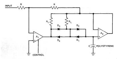
Fig. 7—Leakage compensation in sample-and-hold circuit. The feedback path around  $A_2$  ensures that the drop across  $D_1$  and  $D_2$  is virtually zero, and thus there is no current leakage from C. Resistors  $R_L$  are large and serve to provide a path for residual diode leakage current.
