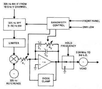
Fig. 9—Receiver third local oscillator PLL circuitry.
