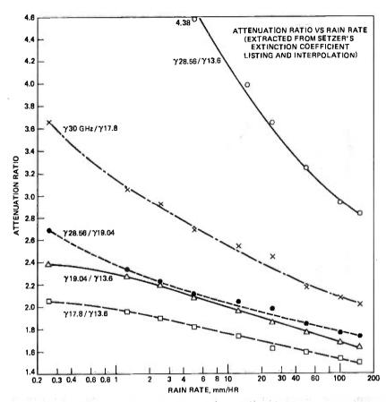
Fig. 14—Attenuation ratios vs. rain rate.
