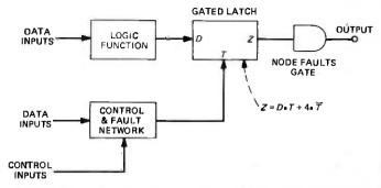
Fig. 3—Block diagram: the general approach for stuck-open/dynamic gate models.
