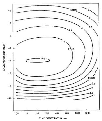
Fig. 9—Equi-rating contours predicted by formula 8, Table III, for 3-bit ADPCM coders.
