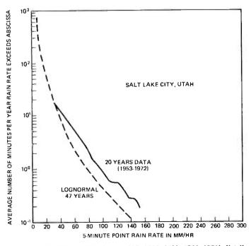
Fig. 21—Comparison of 47-year (1903–1907, 1909–1920, 1922–1951) distribution of 5-minute rain rate calculated by extreme value theory and lognormal hypothesis (dashed line) with 20-year (1953–1972) data (solid line) at Salt Lake City, Utah.
