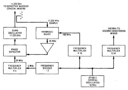
Fig. 4—Receiver local oscillator chain.
