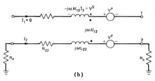
Fig. 5—Classical inductive shielding model. (a) Dependent-source circuit. (b) Complex transformer circuit.
