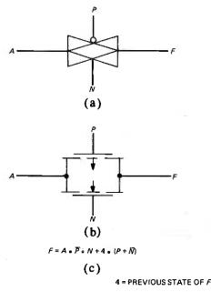
Fig. 5—The CMOS transmission gate: (a) logic symbol, (b) FET realization, and (c) the static, unilateral logic transfer function.
