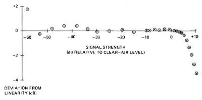
Fig. 19—Receiver input-output amplitude linearity (19-GHz vertical copolarization channel).
