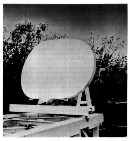
Fig. 2—The subreflector with a machined aluminum surface of 20  $\mu$ m rms. The oval shape is provided for azimuthal off-axis beams.
