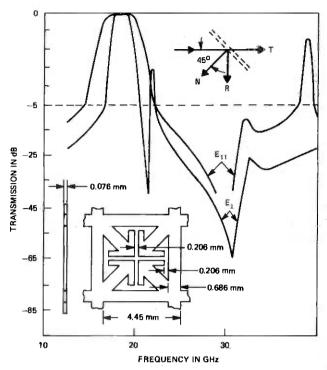
Fig. 5—Transmission of a double-self-supported frequency diplexer (see Fig. 3) with the indicated dimensions of the grid mask at 6.3 mm spacing and 45-degree angle of incidence for two polarizations.
