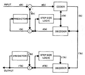
Fig. 1-Block diagram of ADPCM coder-decoder.
