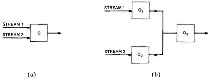
Fig. 2—(a) Queue, Q, fed by two independent input streams, and (b) Queue,  $Q_3$ , fed by the outputs of two queues,  $Q_1$  and  $Q_2$ , which are fed separately by the two input streams.
