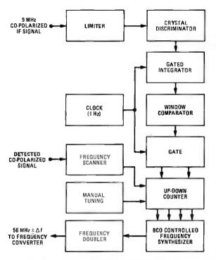
Fig. 3—Automatic frequency tracking control.
