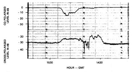
Fig. 9—Anomalous cross polarization event, 11.7 GHz CTS beacon, Holmdel, N.J., August 8, 1976.
