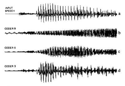
Fig. 5 — Waveforms of the word "tool" for 3-bit ADPCM coders low on dimension II (signal distortion), with different values on dimension III, showing the relationship of attack time to the smooth or rough subjective descriptions.
