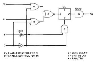
Fig. 13—Input/output port model. Only gates marked \* are faulted, 0 and 1 denote delays, and D and E are enable controls for IN and FI, respectively. FI = fan-in; FO = fanout.
